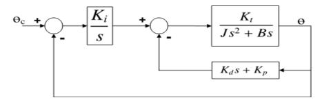
Figure 4.7: IPD Controlled Position Control System
