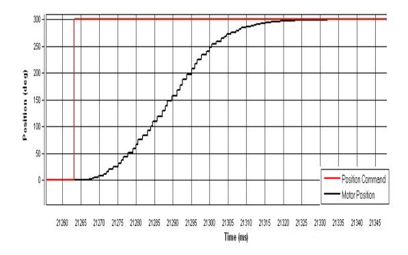
Figure 4.19: Step response of the I-PD controlled system for 300 degree command (experimental result)
