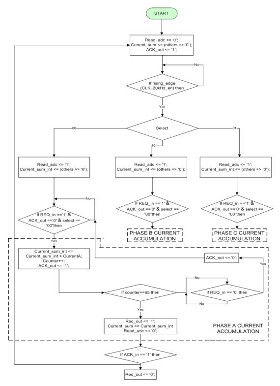
Figure 3.15: Flowchart of the current integrator block
