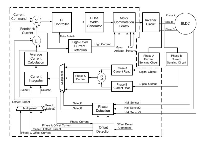
Figure 3.1: Functional Block Diagram of the Current Controller
