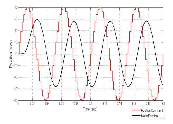
Figure 4.17: Motor position for 20 Hz sine position command of 160 degree magnitude
