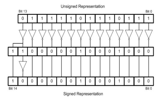
Figure 3.8: Current Scaling of the Negative-Valued Currents
