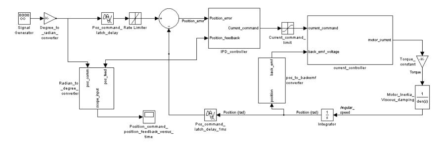
Figure 4.10: Matlab Model of the I-PD Position Control System
