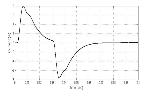
Figure 4.14: Current command of the I-PD controlled system for 300 degree step command
