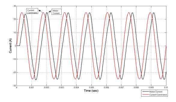
Figure 3.63: Current Command and Current Feedback Signals for a 700 Hz Sine Current Command of 50 A Magnitude
