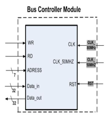
Figure 3.48: Ports of the Bus Controller VHDL Module
