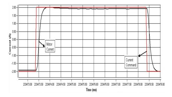
Figure 3.72: Current Command and Current feedback Signals for a 100 Hz Square Current Command of 4A Magnitude
