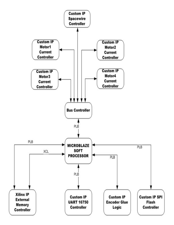
Figure 2.10: Functional Block Diagram of the FPGA Design
