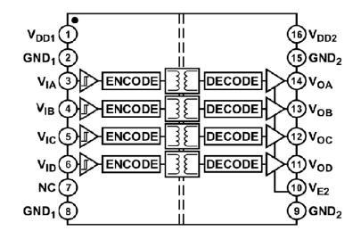
Figure 2.5: Functional Block Diagram of Isolation Chip [14]
