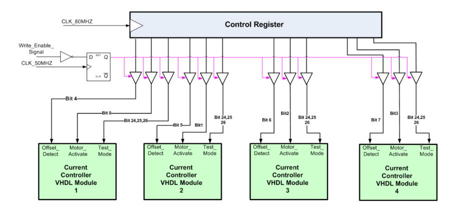
Figure 3.52: Mapping of the control register to the current controller modules' ports
