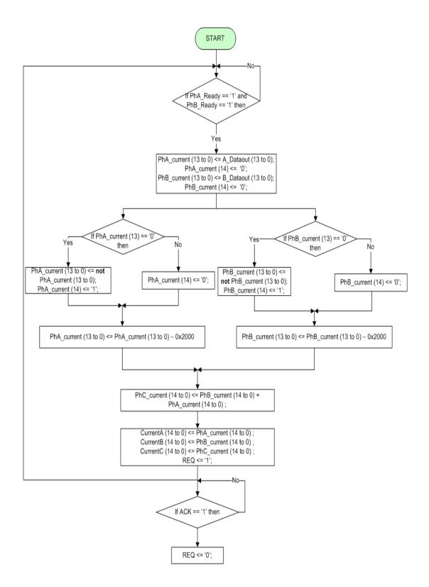
Figure 3.9: Flowchart of the current acquisition block
