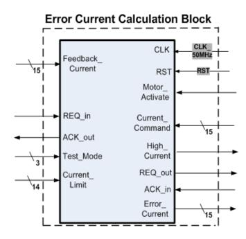
Figure 3.30: Error Current Calculation VHDL Module
