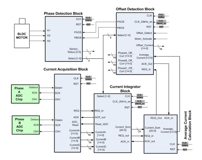
Figure 3.23: Connection of the offset detection block with the other modules
