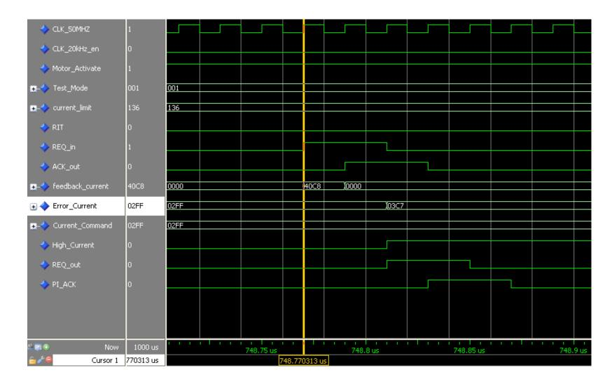
Figure 3.33: Simulation Result Window of the Error Current Calculation Module
