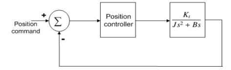
Figure 4.4: Position control system with the motor model
