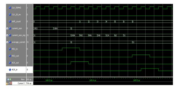
Figure 3.19: Simulation of the Average Current Calculation Module
