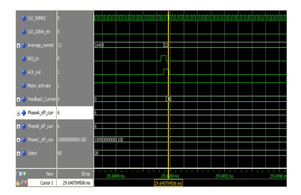
Figure 3.29: Simulation Result Window of the Offset Current Subtraction Module
