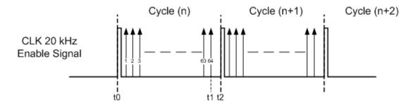
Figure 3.12: Sampling of the Current Feedback
