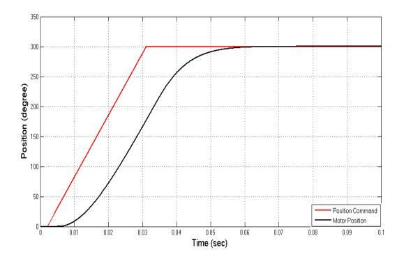
Figure 4.13: Step response of the I-PD controlled system for 300 degree step command
