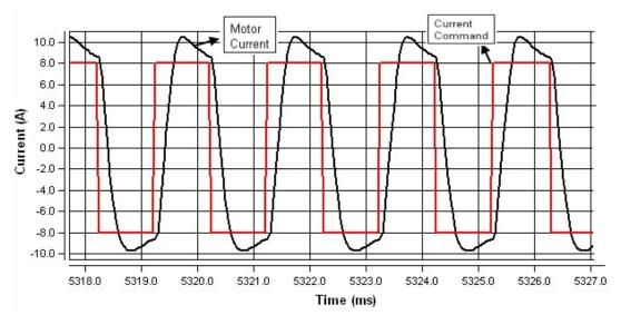
Figure 3.74: Current Feedback Signal for a 500 Hz Square Current Command of 16A Magnitude (Experimental result)
