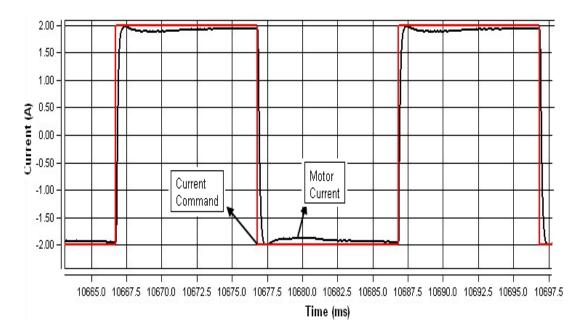
Figure 3.67: Current Command and Current Feedback Signals for a 50 Hz Square Current Command of 4A Magnitude
