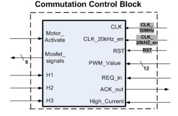
Figure 3.44: Commutation Control VHDL Module
