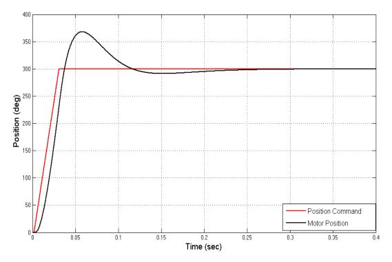
Figure 4.11: Step response of the PID controlled system for 300 degree command
