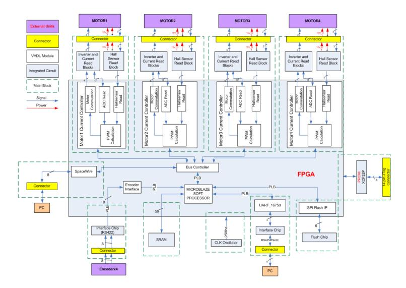
Figure 2.2: Block Diagram of the Electronic Board
