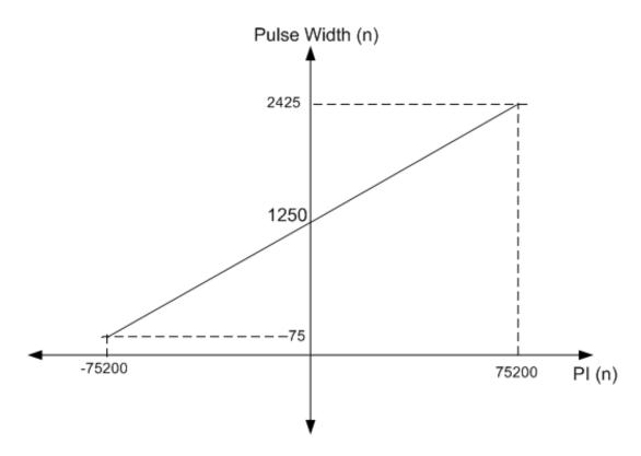
Figure 3.38: PI versus Pulse Width
