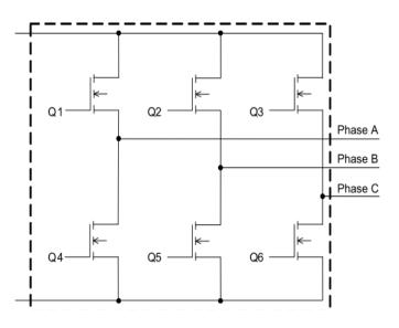
Figure 2.4: Structure of the Inverter Circuit
