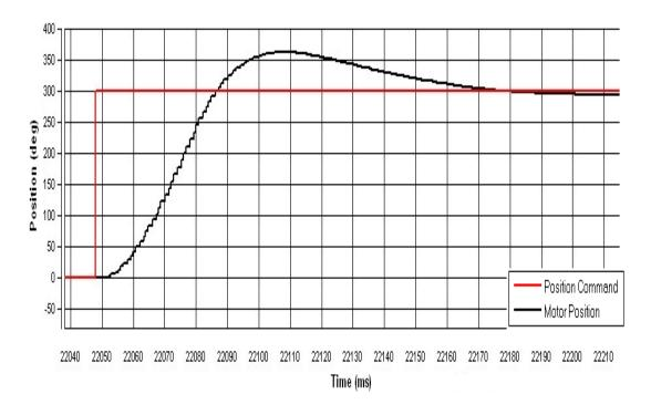
Figure 4.18: Step response of the PID controlled system for 300 degree command (experimental result)
