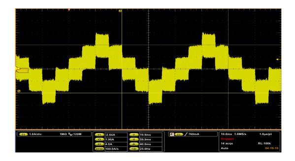
Figure 3.71: Oscilloscope View of Current feedback Signal for a 25 Hz Sine Current Command of 4A Magnitude
