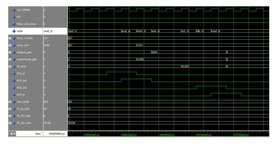
Figure 3.36: Simulation Result Window of the PI Controller Module
