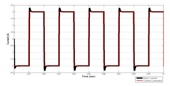
Figure 3.61: Rectified Current Command and Feedback
