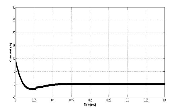
Figure 4.12: Current command of the PID controlled system for 300 degree step command
