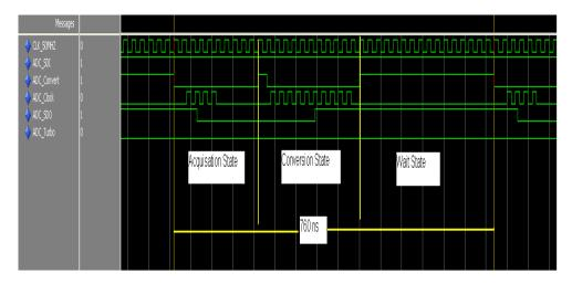
Figure 3.7: Simulation of ADC Driver Code for One Sampling Cycle
