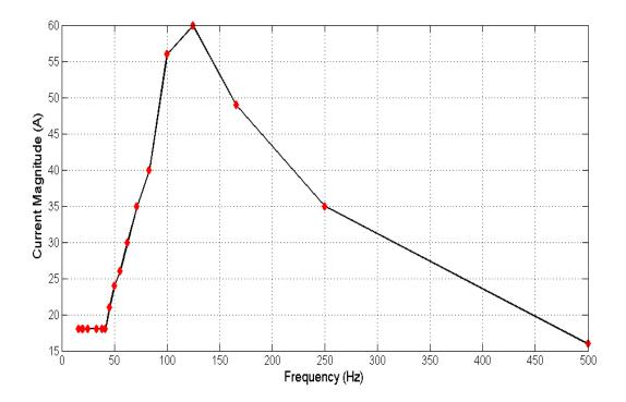
Figure 3.76: Maximum Current Magnitude versus Frequency of the Square Wave Current Command
