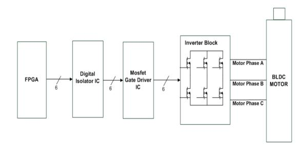
Figure 2.6: Functional Block Diagram of Motor Driver Circuit
