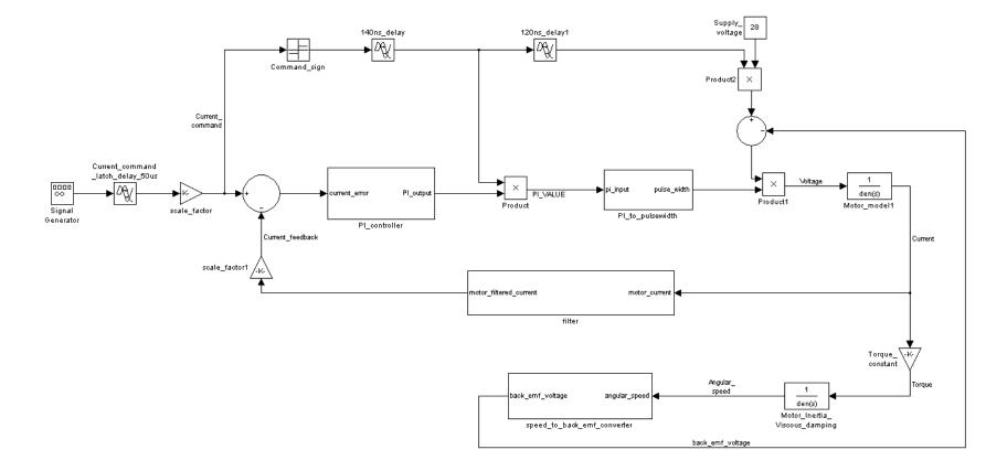
Figure 3.58: MATLAB Model of the Current Controller
