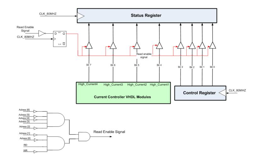
Figure 3.54: Mapping between the status register and current control modules
