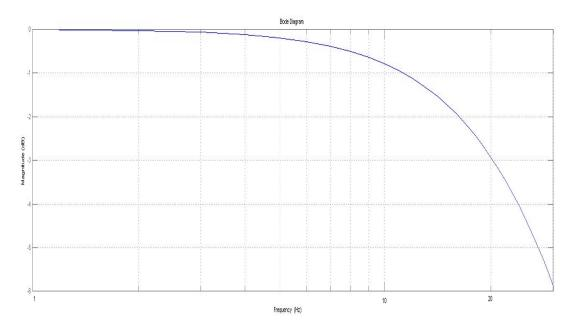
Figure 4.8: Frequency response of the I-PD controlled position control system
