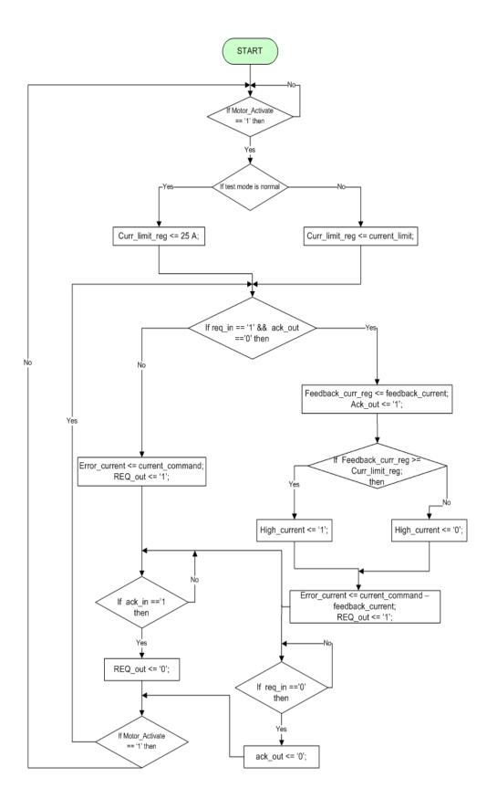
Figure 3.31: Flowchart of the error current calculation VHDL module
