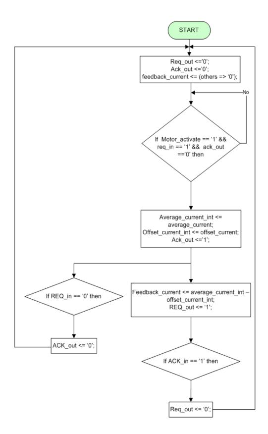
Figure 3.26: Flowchart of the offset current subtraction VHDL module
