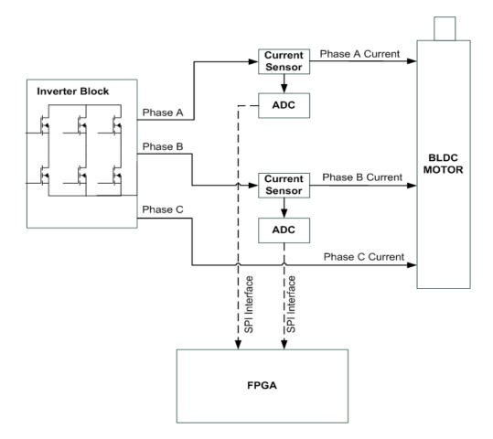
Figure 2.9: Functional Block Diagram of the Current Sensing Circuit
