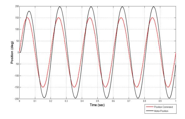
Figure 4.15: Motor position for PID controlled system and 5 Hz, 300 degree peak to peak sine command
