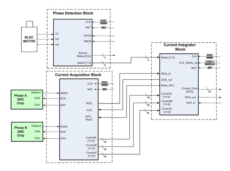
Figure 3.14: Connection between the current integrator module, current acquisition block and phase detection modules
