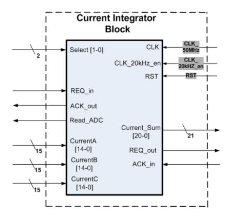
Figure 3.13: Current Integrator VHDL Module
