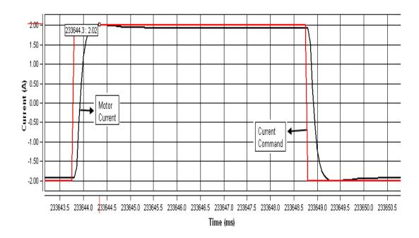
Figure 3.73: Overshoot of Current Feedback Signal for a 100 Hz Square Current Command of 4A Magnitude
