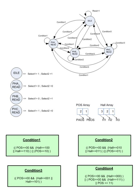
Figure 3.10: State Machine Diagram of the Phase Detection VHDL Module
