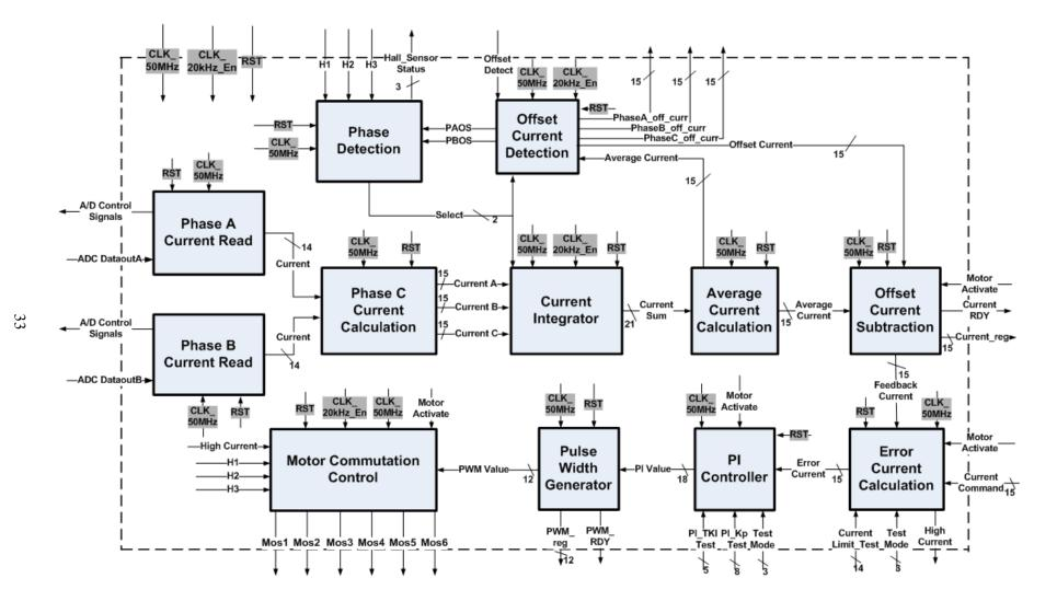
Figure 3.2: Structure of the Current Controller VHDL Module
