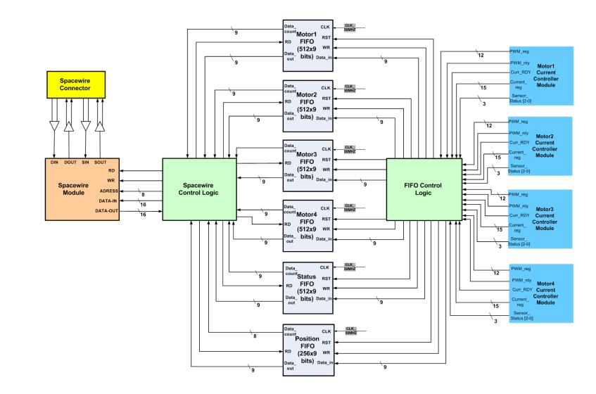
Figure 3.57: Structure of the Feedback Data Control Block
