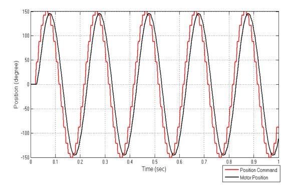
Figure 4.16: Motor position for I-PD controlled system and 5 Hz, 300 degree peak to peak sine command
