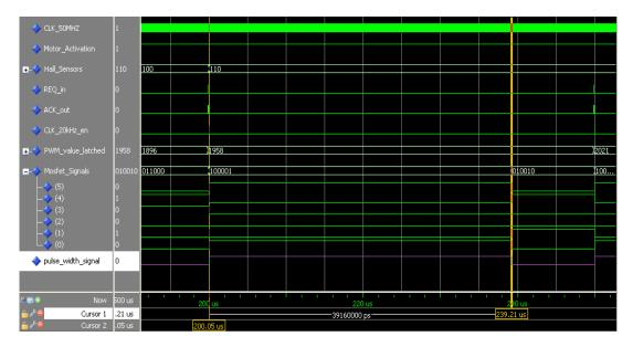
Figure 3.45: Simulation Result Window of the Commutation Control VHDL Module
