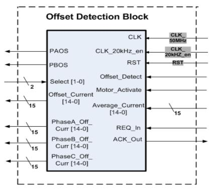
Figure 3.22: Offset Detection VHDL Module
