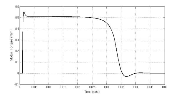
Figure 3.60: Motor Torque for the 4 A Current Command
