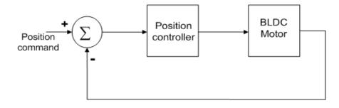
Figure 4.3: Position control system without the postion transducer
