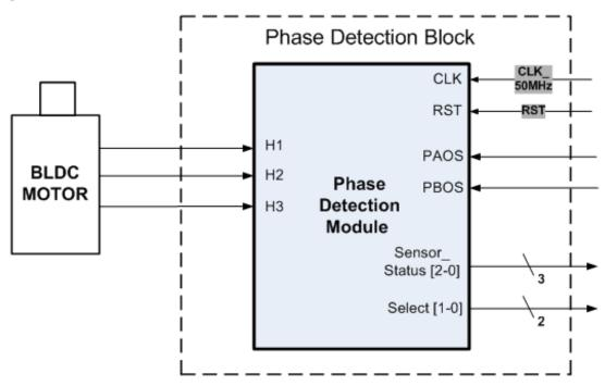
Figure 3.11: Phase detection VHDL module
