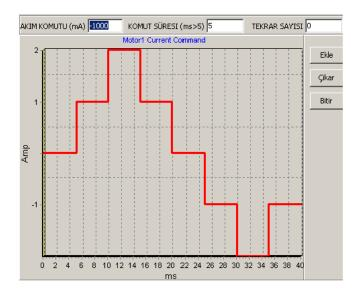
Figure 3.69: Screen Shot of the 25 Hz Sine Current Command of 4A Magnitude
