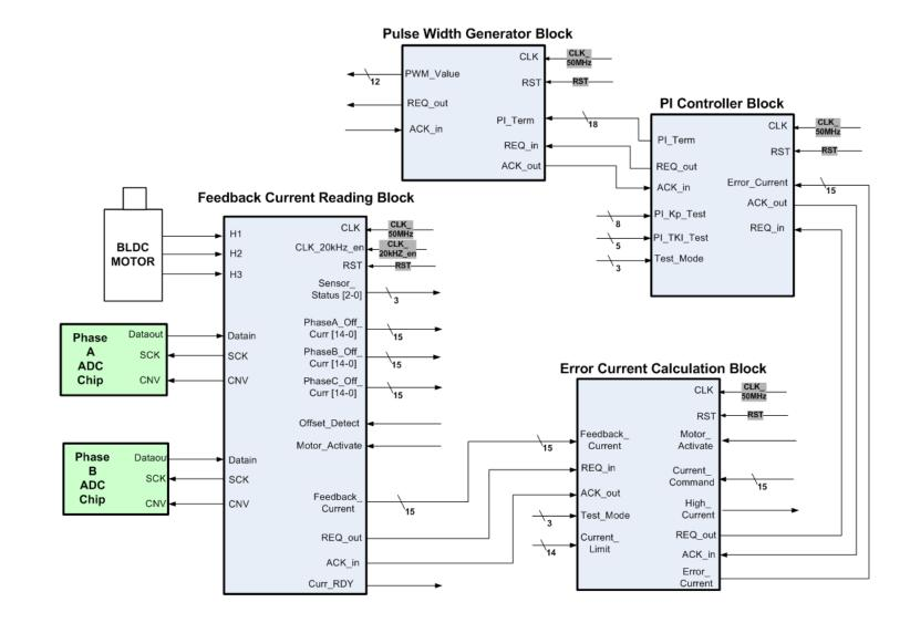
Figure 3.42: Connection between the pulse width generator module and the other VHDL modules
