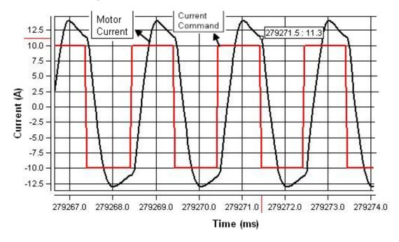
Figure 3.75: Current Feedback Signal for a 500 Hz Square Current Command of 20A Magnitude (Experimental result)
