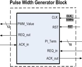
Figure 3.39: Pulse width generator module
