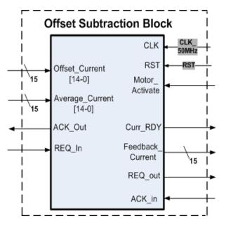
Figure 3.25: Offset current subtraction VHDL module
