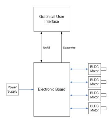
Figure 2.1: General Diagram of the Motor Control System
