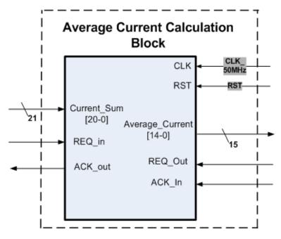
Ports of the average current calculation module are shown in the Figure 3.18.
