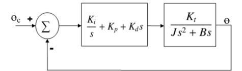
Figure 4.5: PID Controlled Position Control System
