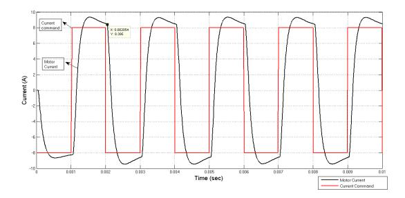
Figure 3.65: Current Command and Current Feedback Signals for 500 Hz Square Wave Current Command of 16 A Magnitude
