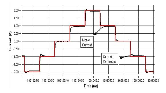
Figure 3.70: Current Command and Current feedback Signals for a 25 Hz Sine Current Command of 4A Magnitude
