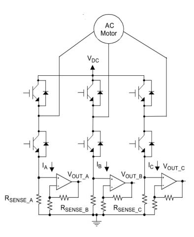
Figure 2.7: Current measurement with three shunt resistors
