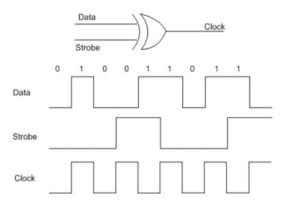
Figure 2.3: Data-Strobe Encoding
