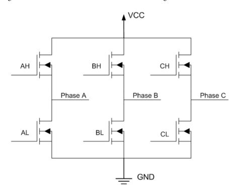
Figure 3.43: Notation of the Commutation Control's Outputs on the Inverter Circuit
