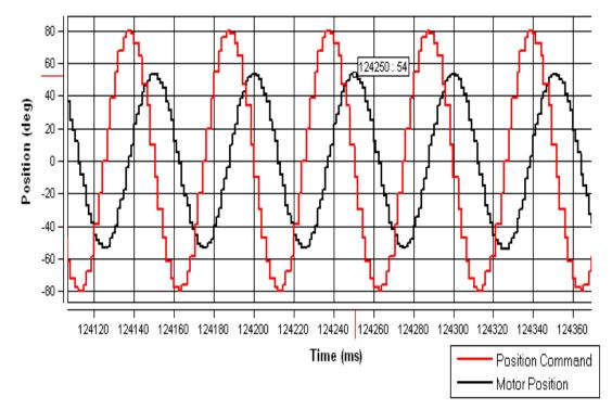
Figure 4.22: Motor position for 20 Hz sine position command of 160 degree magnitude (experimental result)
