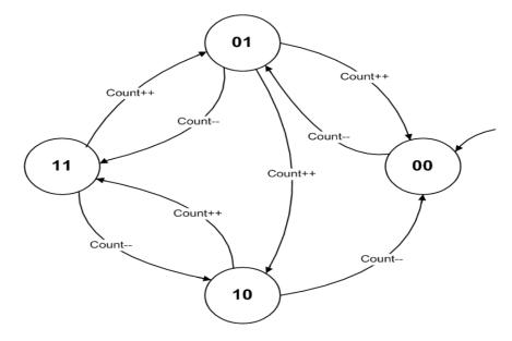
Figure 4.9: State Machine Diagram of the Encoder Interface Module
