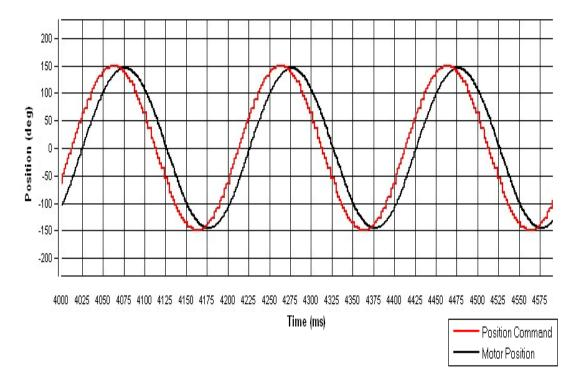
Figure 4.21: Motor position for I-PD controlled system and 5 Hz, 300 degree peak to peak sine command (experimental result)
