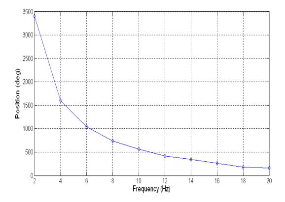
Figure 4.23: Magnitude of the position command versus frequency of the sine wave position command
