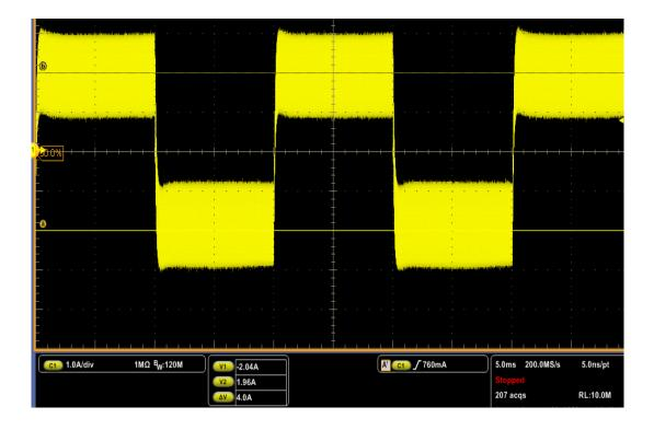
Figure 3.68: Oscilloscope View of Current Feedback Signal for a 50 Hz Square Current Command of 4A Magnitude
