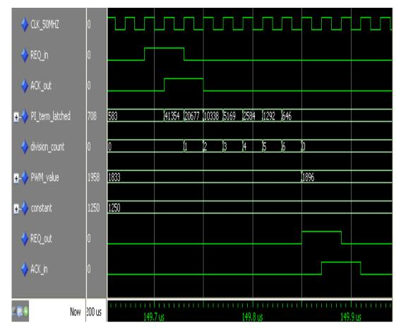
Figure 3.41: Simulation Result Window of the Pulse Width Generator Module
