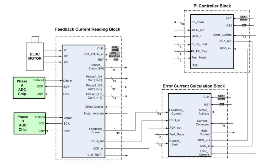
Figure 3.37: Connection of the PI controller module with the other modules
