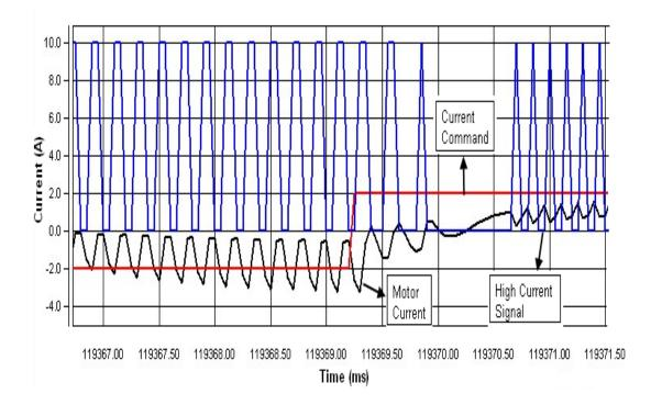
Figure 3.77: High Current Signal for 1 A Current Limit
