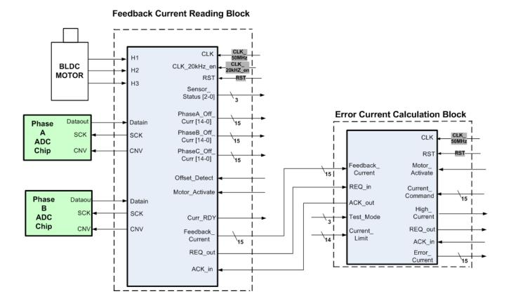
Figure 3.32: Connection diagram between the error current calculation module and the feedback current reading module
