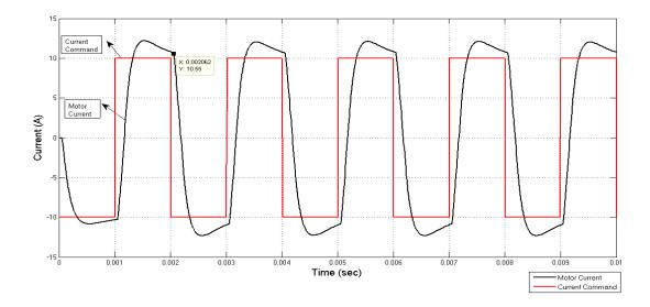
Figure 3.66: Current Command and Current Feedback Signals for 500 Hz Square Wave Current Command of 20 A Magnitude
