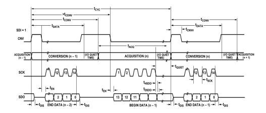
Figure 3.6: Serial Interface Timing Diagram of AD7944 chip [19]
