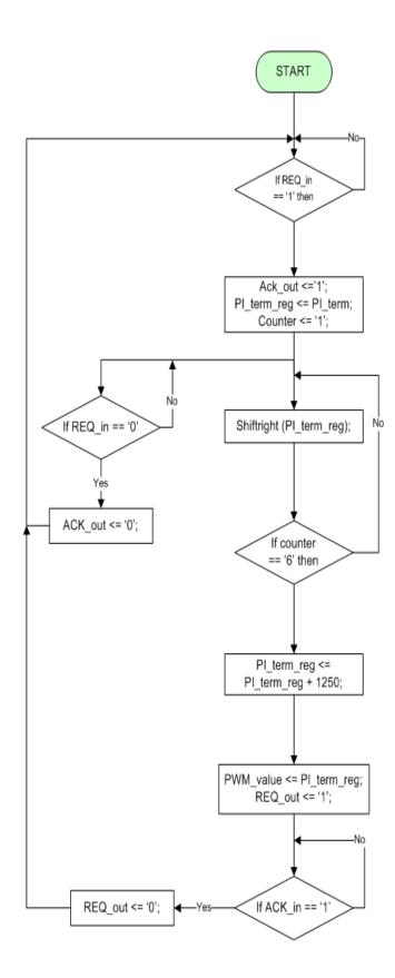
Figure 3.40: Flowchart of the pulse width generator VHDL module
