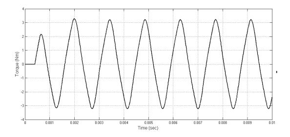
Figure 3.64: Motor Torque for 700 Sine Current Command of 50 A Magnitude
