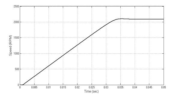
Figure 3.59: Motor Speed for the 4 A Current Command
