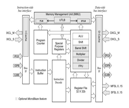
Figure 2.11: Functional Block Diagram of the Microblaze Processor Core [17]
