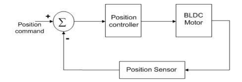
Figure 4.2: Position control system without the current control loop
