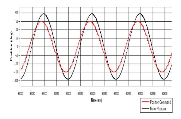
Figure 4.20: Motor position for PID controlled system and 5 Hz, 300 degree peak to peak sine command (experimental result)
