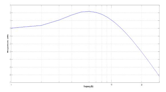
Figure 4.6: Frequency response of the PID controlled position control system
