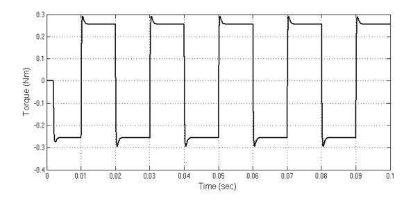
Figure 3.62: Motor Torque for 4A Peak-to-Peak Square Waveform Current Command
