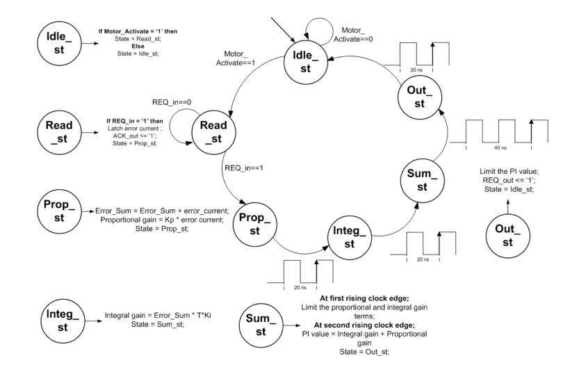
Figure 3.35: PI controller state machine
