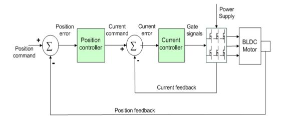
Figure 1.1: Block Diagram of the Control System
