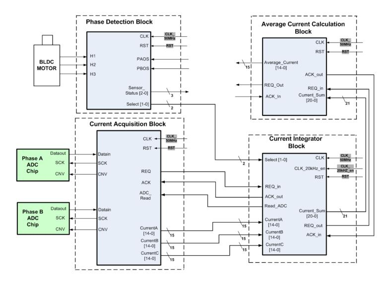
Figure 3.20: Connection of the average current calculation module with the other modules
