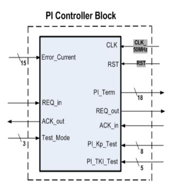
Figure 3.34: PI controller VHDL module
