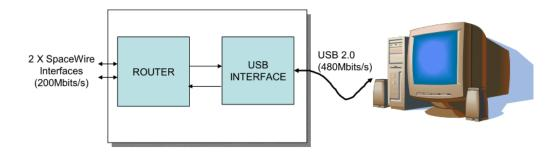
Figure 2.19: An Overview of the SpaceWire Brick Hardware Architecture [18]
