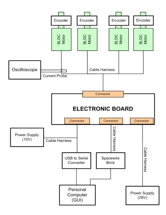
Figure 2.18: Structure of the Test Setup
