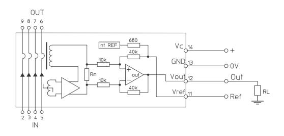
Figure 2.8: Functional Block Diagram of the Current Sensor [16]
