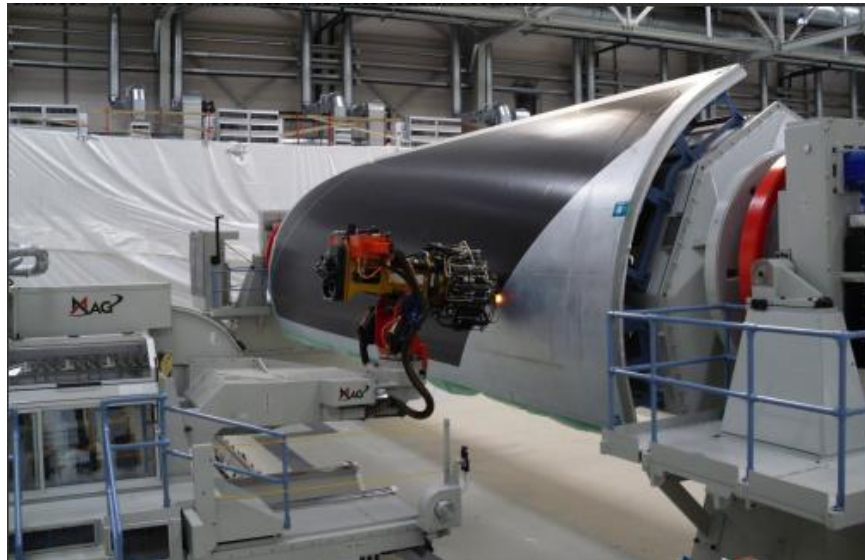
Figure 1.9: Manufacturing of fuselage panel for Airbus A350 aircraft, taken from Ref. [6]
