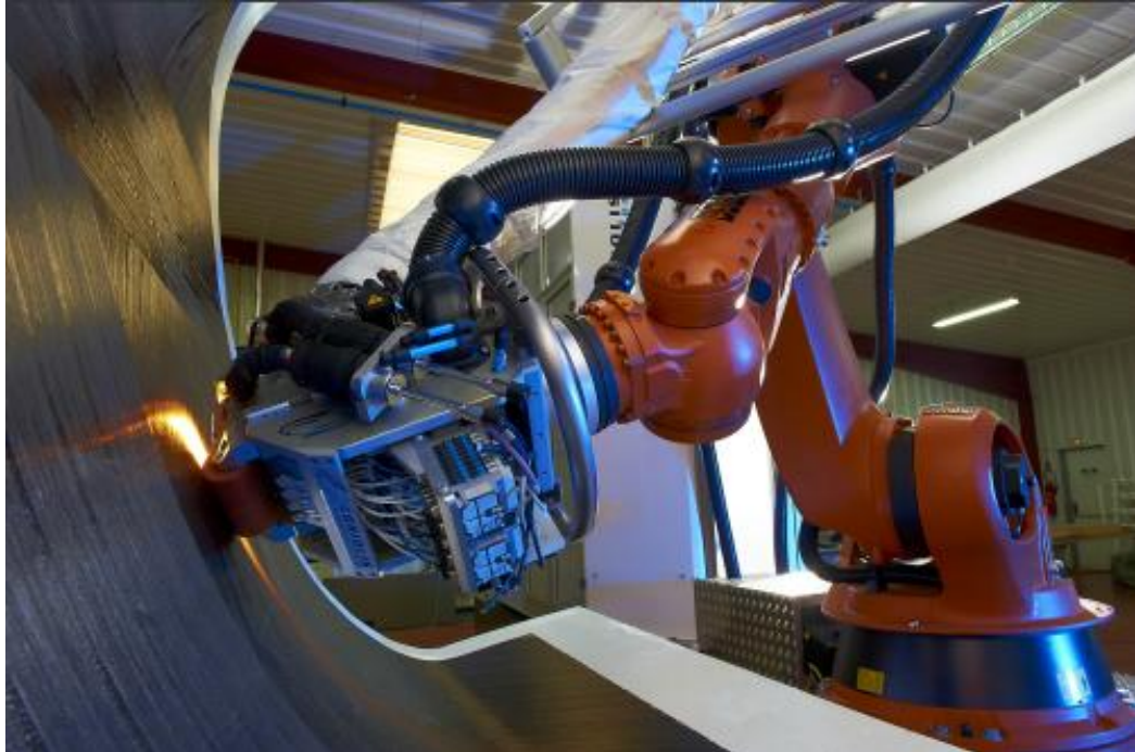
Figure 1.4: An actual tow placement machine used in the industry, taken from Ref. [6]
