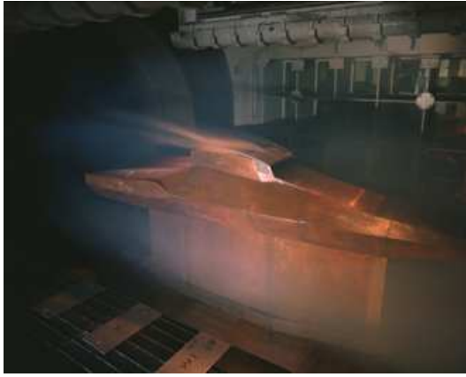
Figure 1.6: The X43 in the NASA LaRC M=10 wind tunnel.
