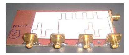
Figure 4.2: A photograph of the final beam former with connectors and applied tuning.
