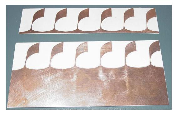
Figure 4.19: Implemented beamformer and antenna assembly – back side of the board
