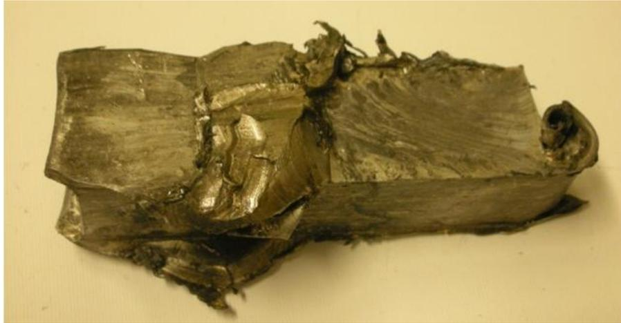
Figure 3.3.49. Failure of S13 due to extreme mushrooming (1A@ 200 °C).
