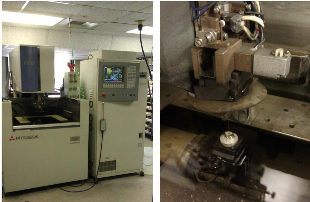
Figure 3.2.6. Wire EDM system.
