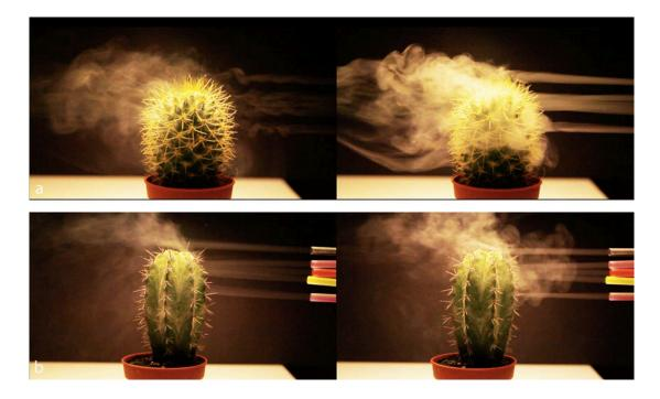
**Figure 4.5** Mammillaria Cowparea and Polaskia Chichipe fluid dynamics performance analysis: (a) low velocity, (b) high velocity air flow. [Experiment and photos by the author]
