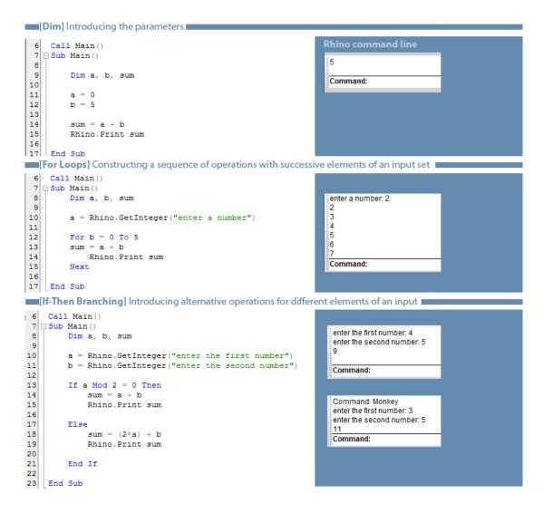
**Figure 4.15** A basic summation operation in rhino script evolves to be more complex as *for loops* and *if-then* branches are introduced. [Illustrated by the author]The interaction of the script program with Rhinoceros is illustrated at the right-hand side. Since the summation operation doesn't include visual elements, the command line screens the outcome of the system.
