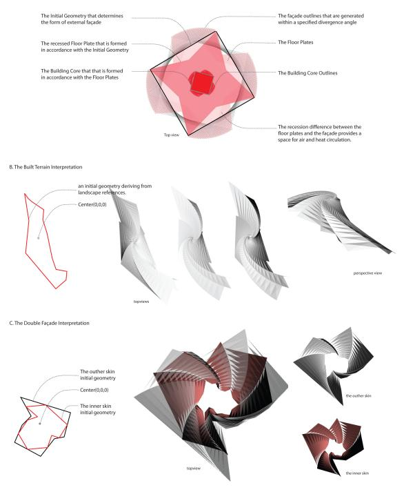
**Figure 5.2** Three different architectural projections of the Cactus Script: (a) High-rise buildings, (b) built terrains, (c) double façades.
