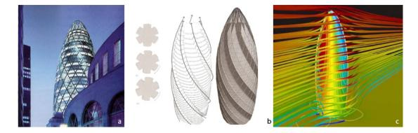
**Figure 4.11** Mary Axe Tower by Norman Foster (2004, London), and its interpretation for transferring natural form's air flow performance into architecture: (a) A photo of the building (b) A graphic illustration of the building's air flow control through the interior floor layers, (c) The CFD analysis of the buildings external form.
