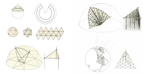
**Figure 2.9** Buckminster Fuller's sketches about the development of geodesic domes. Graphics collected from: R. Buckminster Fuller. *The Critical Path.* pp. 164, 165, 166.
