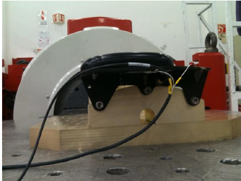
Figure 5.31 A View of the Cantilever Beam Fixture Fixed to Electromagnetic Vibration Test Equipment
