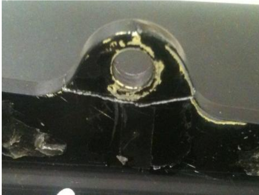
Figure 5.32 Final View of the Bracket that is subjected to Fatigue Test
