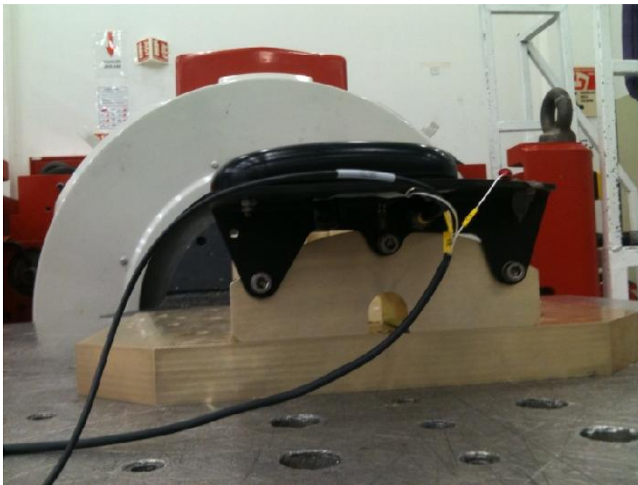
Figure 4.2 Manufactured Bracket and Shaker Fixture
