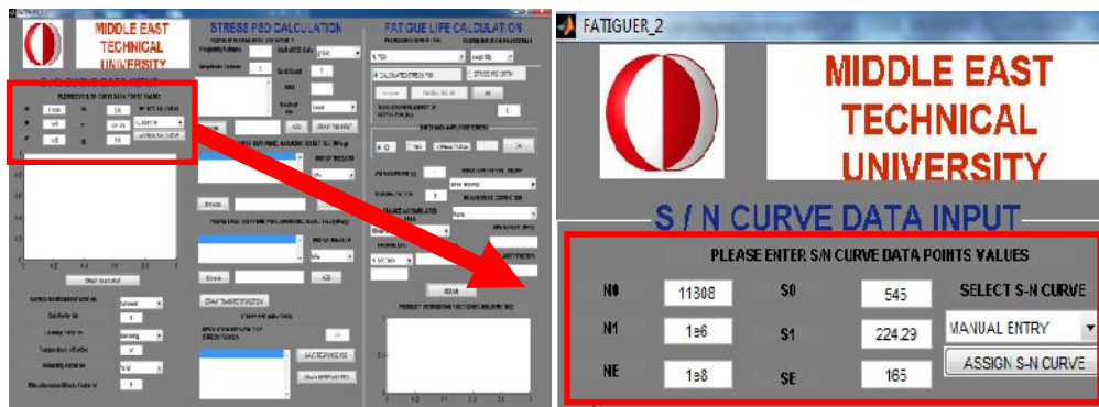
Figure C. 2 Manual Entry for S-N Curve Information of Material
