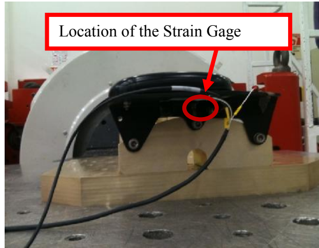
Figure 4.17 Location of the Strain Gage
