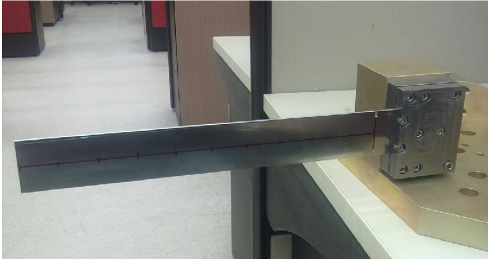
Figure 4.1 Manufactured Beam and Shaker Fixture
