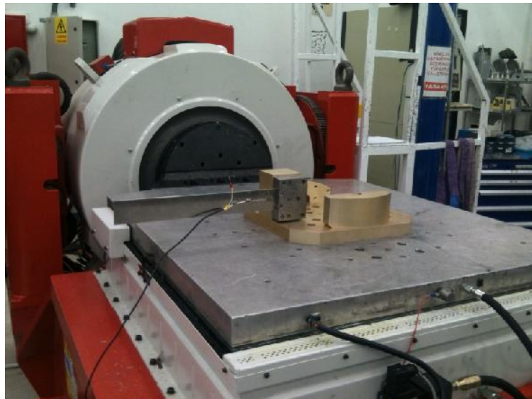
Figure 5.6 A View of the Cantilever Beam Fixture Fixed to Electromagnetic Vibration Test Equipment
