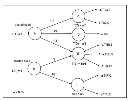
Figure 3.1: TrustRank calculation by splitting method.
