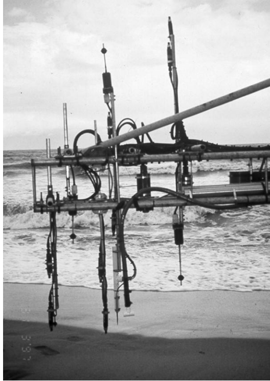
Figure 4.58 Vertical array of instruments mounted on the lower boom of SIS (Miller, 1999)
