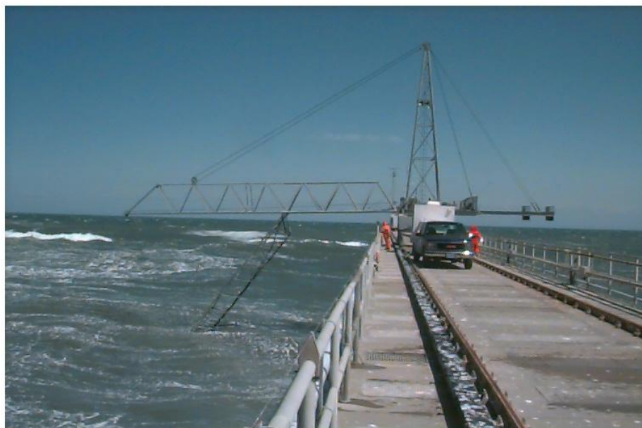
Figure 4.57 Sensor Insertion System (SIS) on the FRF Pier (URL-2)
