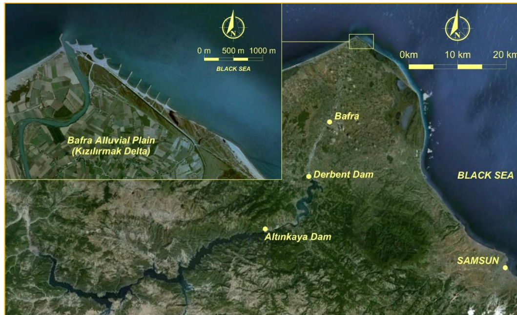
Figure 5.2 Bafra alluvial plain and plan view of the existing shore protection system at the Kızılırmak River mouth (Google Earth, 2011)
