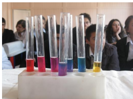
Figure 3.5 The pH scale of red cabbage juice obtained in the experimental class (from left to right HCl solution, lemon juice, vinegar, water, carbonate solution, ammonia, NaOH solution)
