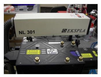
Figure 17. Two different Nd:YAG lasers, One at 1064 nm (Ekspla NL 301) and the other is the second harmonic, i.e. at 532 nm (Big Sky)
