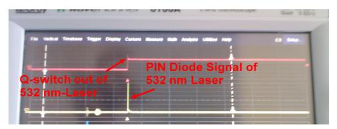
Figure 24. Q-switch out and PIN diode signals of 532 nm-laser shown in oscilloscope screen
