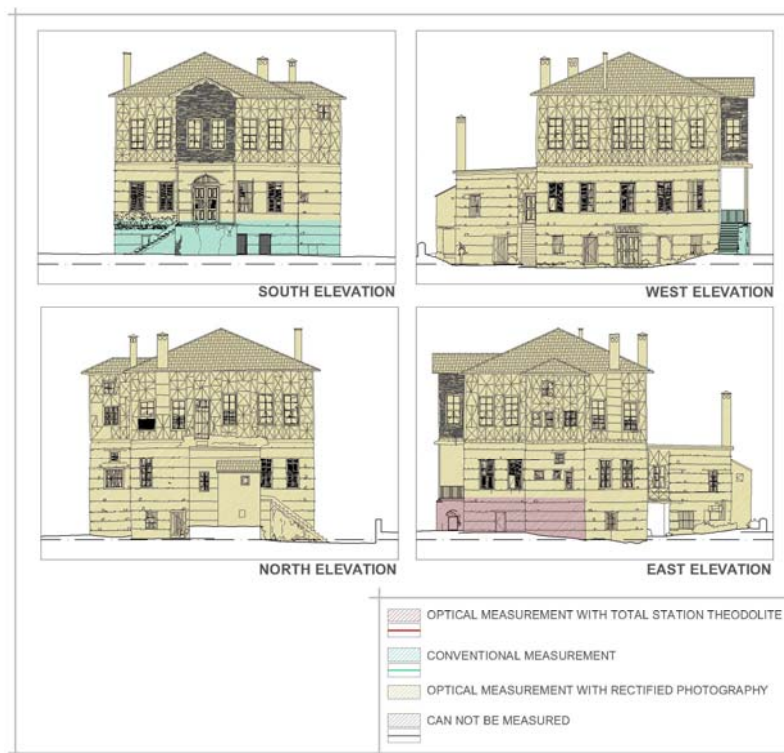
Figure 1.2. Measurement Methods (Parts measured with TST and rectified photography techniques.)
