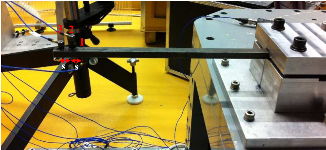
Figure 5.24 Close Accelerometers Method for Substructure A
