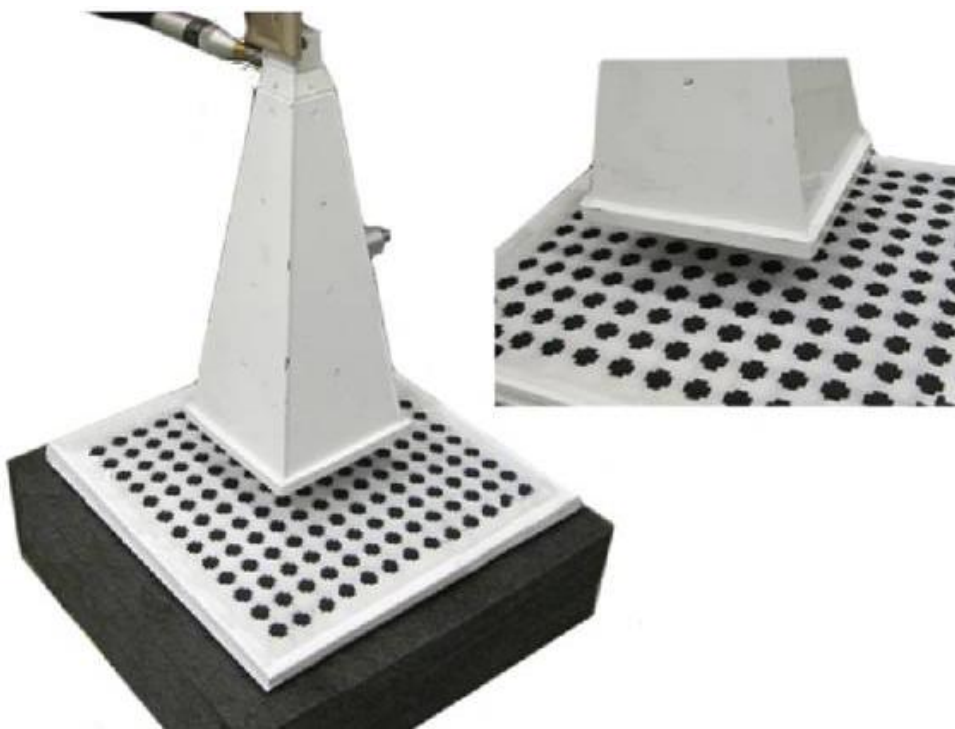
Figure 5-22 Reflectivity measurement setup
