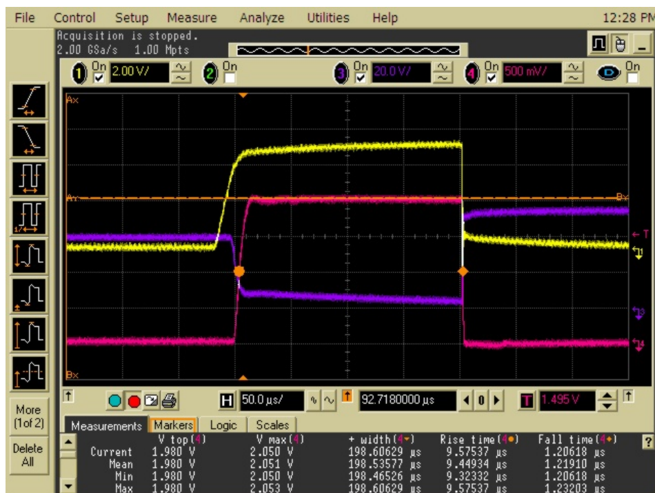
Figure 4-3. Oscilloscope measurements for 100A LD current with duration of 200µs – the voltage across gate and source terminals of the low side MOSFET vs. time (yellow), the voltage across drain and source terminals of the low side MOSFET vs. time (purple) & the current through the LDs vs. time (red).
