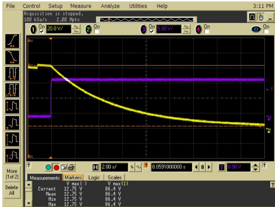
Figure 4-2. Input capacitor discharging and gate voltage of the discharge MOSFET switch in response to “discharge” command – input capacitor voltage vs. time (yellow) & gate voltage of the discharge MOSFET switch vs. time (purple).
