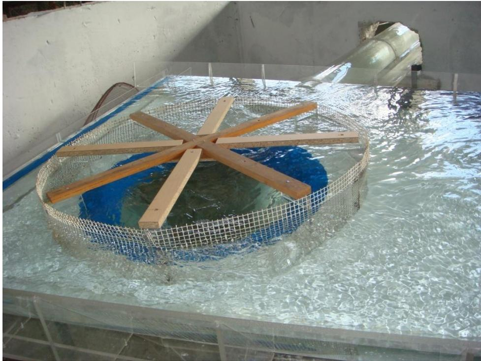
Figure 2.8 Flow conditions with vertical cylindrical screen
