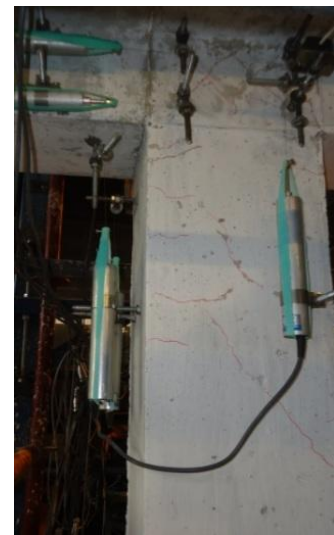
Figure 3. 17: Crack pattern comparison in critical damage regions interior column 103 and the first story interior joint (SP2)
