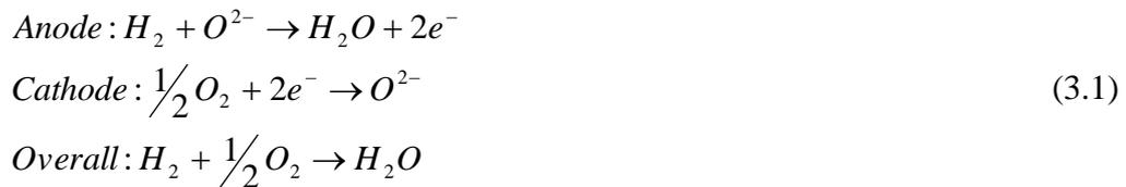
The oxygen ions produced at the cathode, pass through the electrically insulated electrolyte to the anode side. At the anode, the oxygen ions react with the hydrogen ions to form the water and 2 moles of electrons are released for a 1 mole of the hydrogen. These steps are shown in Figure 3.1.
