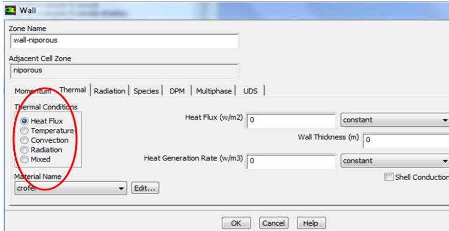
Figure A.12 A screen shot for determining the external wall thermal conditions
