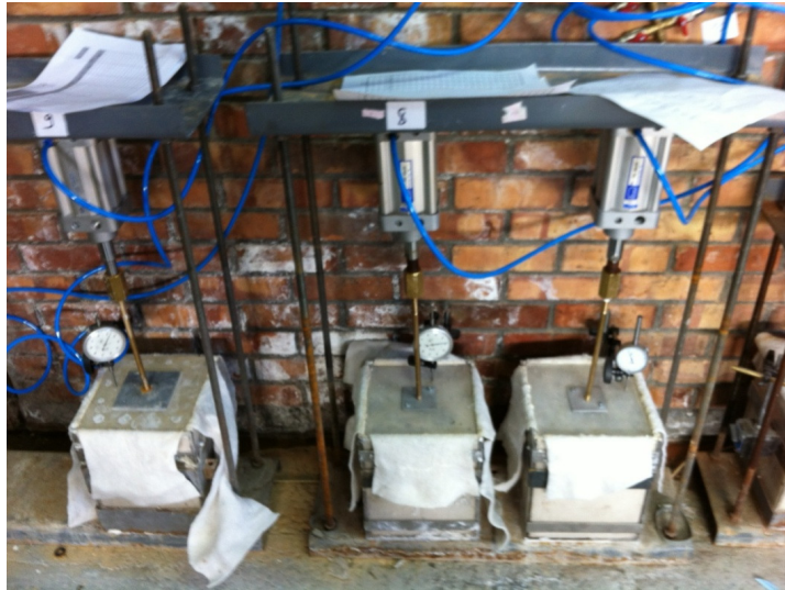
Figure 3.21 Air jack system
