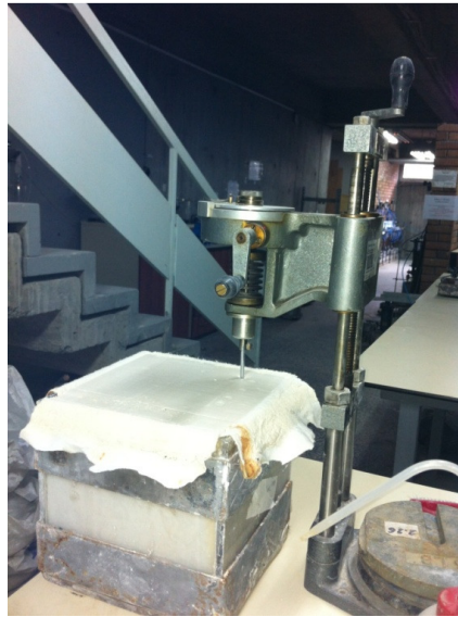
Figure 3.35 Vane shear test
