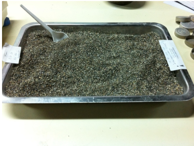
Figure 3.38 Sand used for stone column construction
