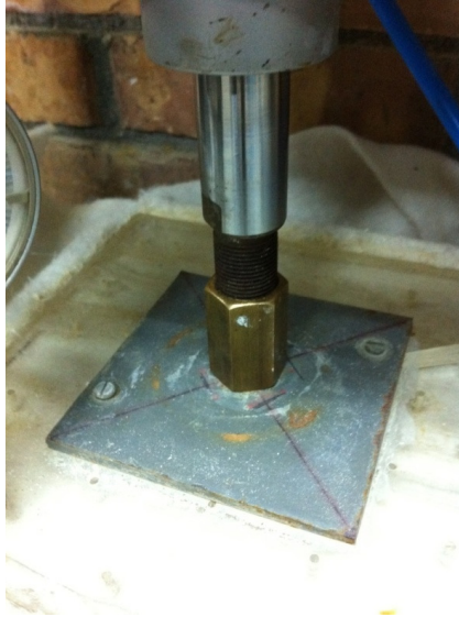
Figure 3.32 Application of consolidation pressure (40kPa) with the jack system
