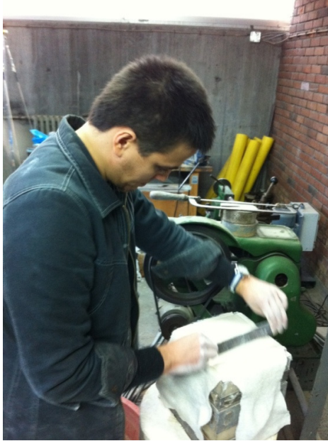
Figure 3.33 Removal of the 50 mm top portion and flattening the surface
