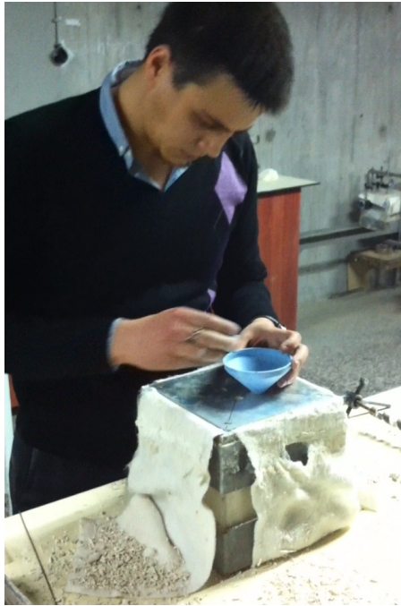
Figure 3.40 Filling the boreholes
