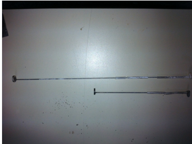
Figure 3.26 Telltales for subsurface settlement measurement
