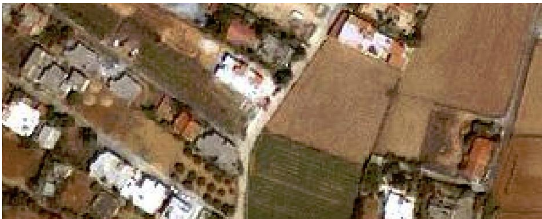
Figure 11: An example of road topology with different road parts having different spectral features
