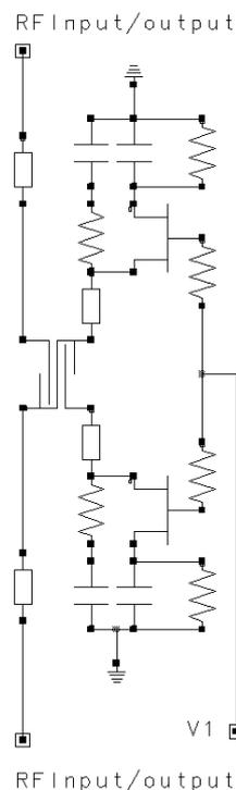
Figure 2-22. Schematic of the phase shifter proposed in [15].
