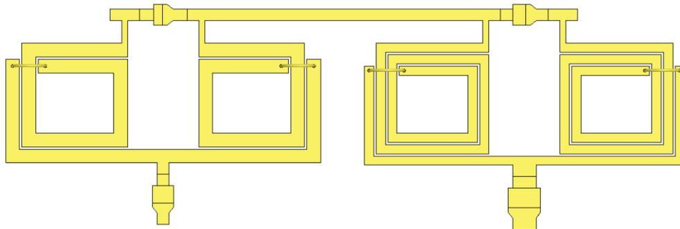
Figure 5-26. Lower branch of 1 to 2 GHz phase shifter 22.5° phase shift bit (Length: 5.826 mm, Width: 1.972 mm, Separation between inductors: 374  $\mu\text{m}$ ).
