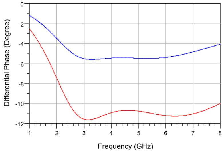
Figure 5-40. Ideal phase responses of 5.625° (blue line), and 11.25° (red line) phase shift bits constructed with ideal lumped elements for 3 to 6 GHz phase shifter.
