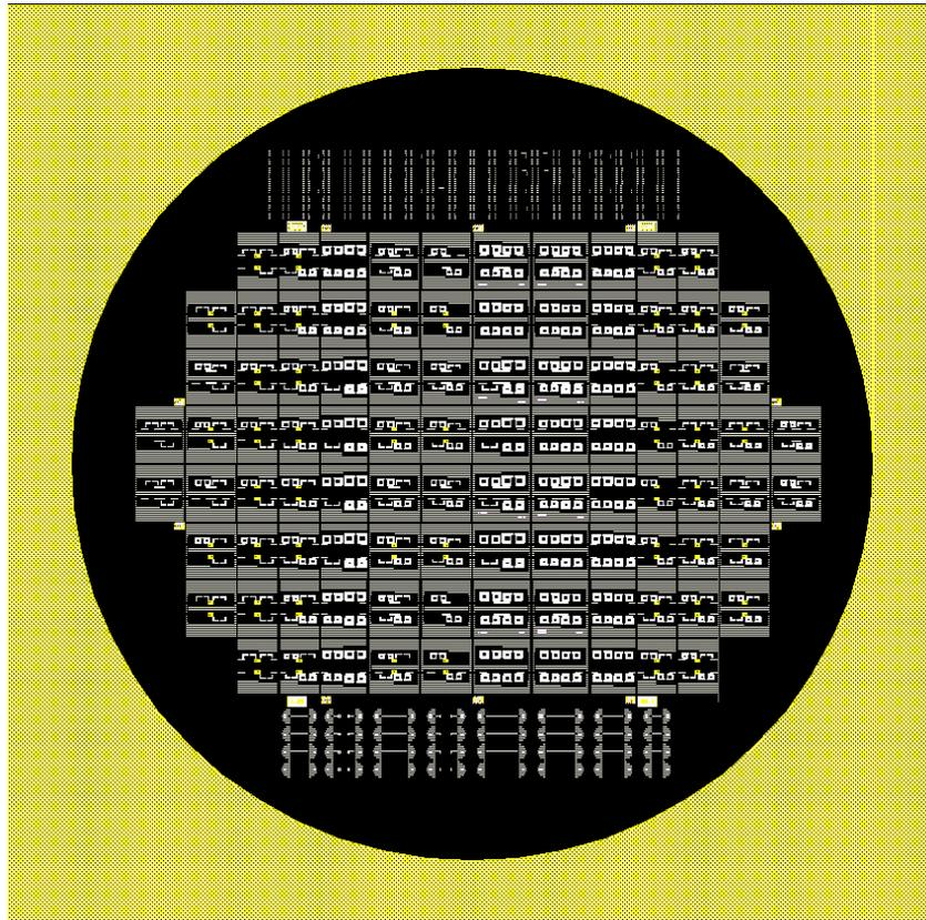
Figure 6-2. Mask Set of Phase Shifters.
