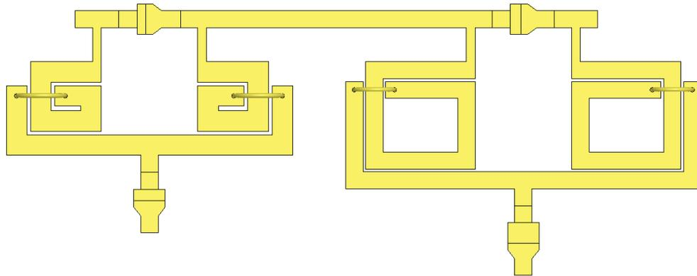
Figure B-12. Lower branch of 3 to 6 GHz phase shifter 45° phase shift bit (Length: 4.008 mm, Width: 1.595 mm, Separation between inductors: 306  $\mu\text{m}$ ).
