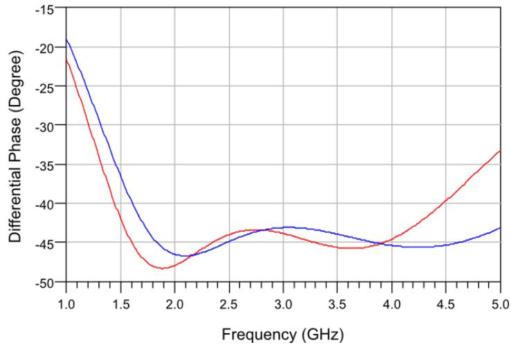
Figure A-10. The differential phase shift response of 2 to 4 GHz phase shifter 45° phase shift bit layout considered, and iterated shunt MIM capacitors (red line represents the present case, and blue line represents the ideal case).
