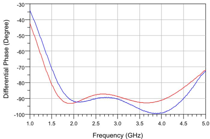
Figure 6-14. Differential phase response of 2-4 GHz 90° DCM phase shift bit measurement in comparison with practical design (red line represents the practical design and blue line represents the measurement result).
