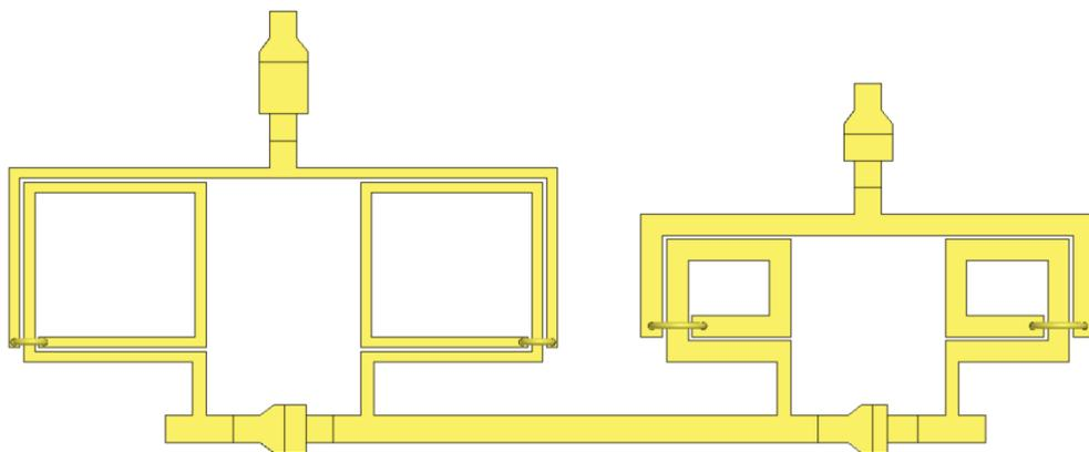
Figure A-11. Upper branch of 2 to 4 GHz phase shifter 45° phase shift bit (Length: 4.014 mm, Width: 1.652 mm, Separation between inductors: 308 μm).
