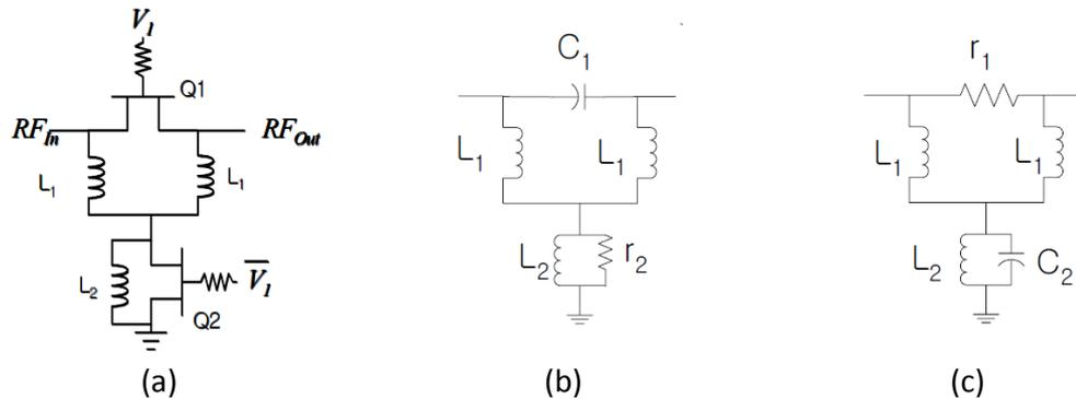
Figure 2-21. (a) The schematic of the phase shifter using resonated FET circuit (b) The equivalent circuit of high-pass filter state (c) The equivalent circuit of the reference state [14].
