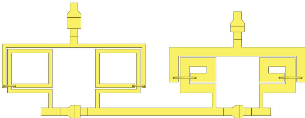
Figure B-7. Upper branch of 3 to 6 GHz phase shifter 90° phase shift bit (Length: 3.936 mm, Width: 1.53 mm, Separation between inductors: 304 μm).
