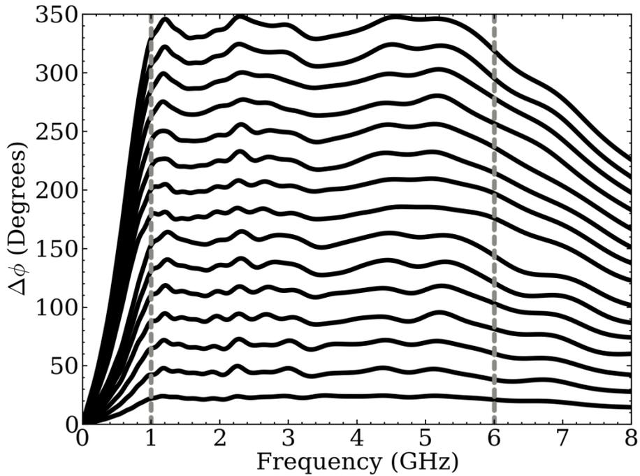
Figure 5-48. Simulated phase performance of the practical UWB phase shifter for all bit states.
