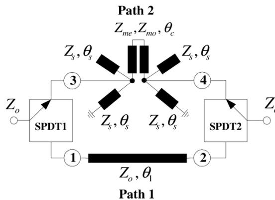
Figure 2-7. The proposed phase shifter consists of a  $\lambda/2$  coupled line and parallel  $\lambda/8$  open and short stubs [7].
