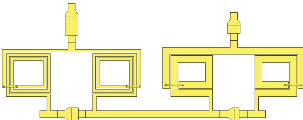
Figure A-3. Upper branch of 2 to 4 GHz phase shifter 180° phase shift bit (Length: 4.218 mm, Width: 1.664 mm, Separation between inductors: 300 μm).
