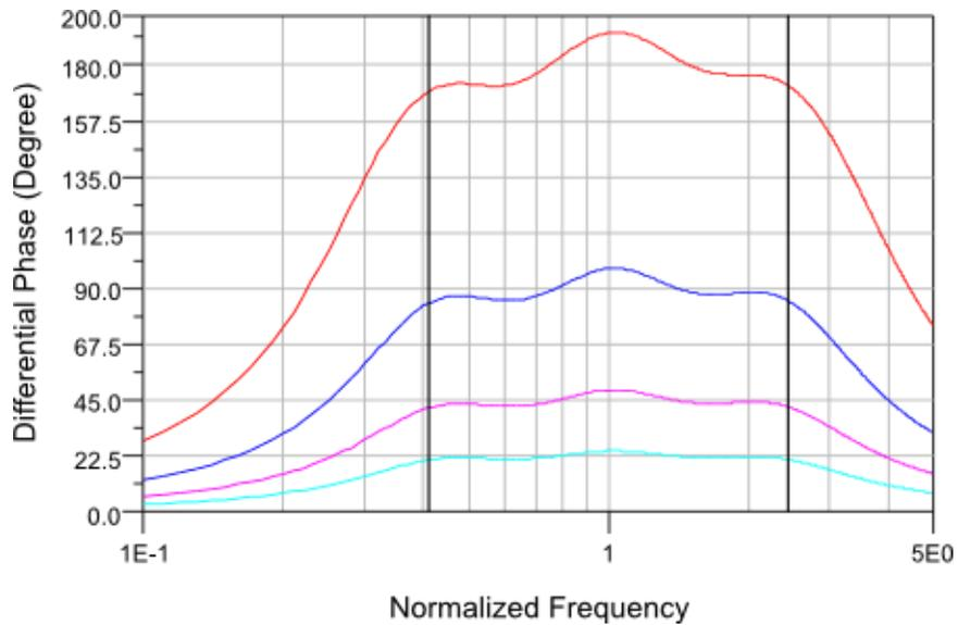
Figure 3-23. Differential phase shift plots for 22.5° (turquoise line), 45° (pink line), 90° (blue line), and 180° (red line), for three-stage 6:1 bandwidth.
