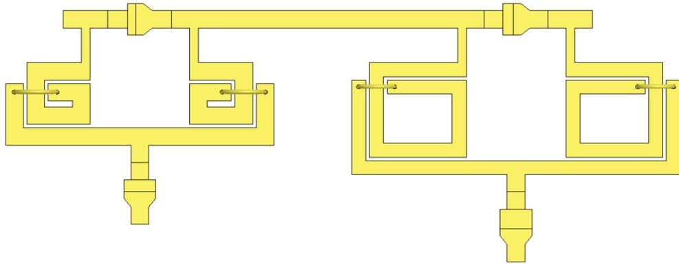
Figure B-8. Lower branch of 3 to 6 GHz phase shifter 90° phase shift bit (Length: 3.802 mm, Width: 1.49 mm, Separation between inductors: 438  $\mu\text{m}$ ).
