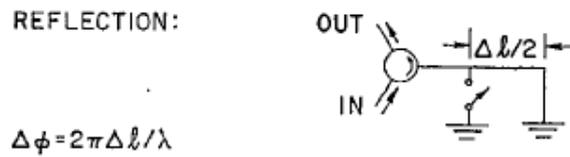
Figure 1-3. Reflection Type Phase Shifter Circuit [2].
