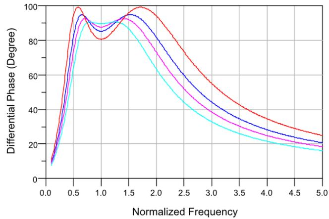
Figure 3-12. Differential phase shift plots for 90° bit two-stage for bandwidths of 2:1 (turquoise line), 3:1 (pink line), 4:1 (blue line), and 6:1 (red line).
