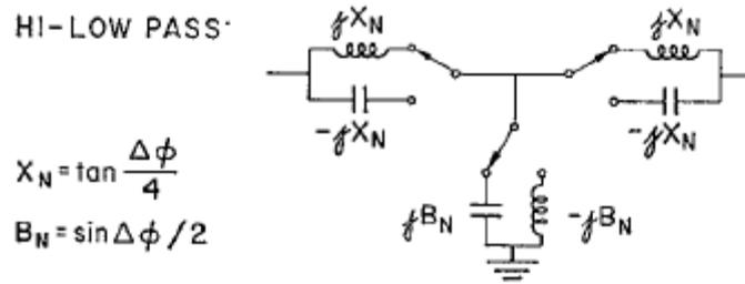
Figure 1-5. The High-Pass/Low-Pass Phase Shifter Circuit [2].
