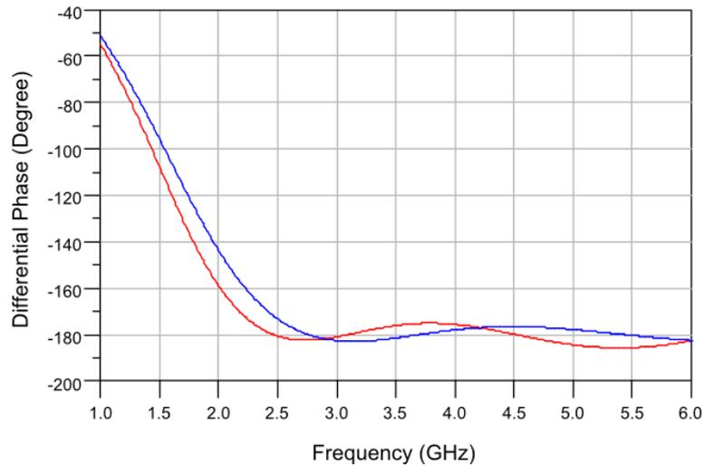
Figure B-2. The differential phase shift response of 3 to 6 GHz phase shifter 180° phase shift bit layout considered, and iterated shunt MIM capacitors (red line represents the present case, and blue line represents the ideal case).
