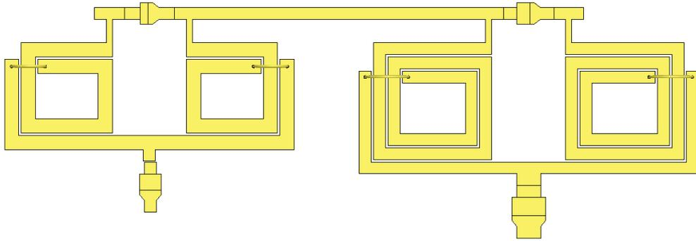
Figure 5-18. Lower branch of 1 to 2 GHz phase shifter 90° phase shift bit (Length: 5.818 mm, Width: 1.998 mm, Separation between inductors: 546  $\mu\text{m}$ ).
