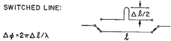
Figure 1-2. Switched Line Phase Shifter Circuit [2].
