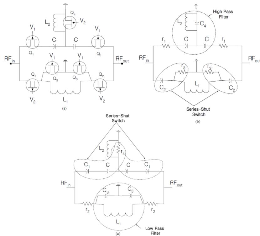
Figure 2-20. (a) The circuit schematic of the proposed phase shifter (b) The state where  $V_1=0V$ ,  $V_2= -4V$  in which the circuit act like a high-pass filter (c) The state where  $V_1=-4V$ ,  $V_2= 0V$  in which the circuit act like a low-pass filter [13].
