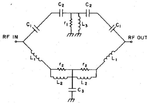
Figure 2-11. The circuit representation when state becomes  $V_1$  is equal to zero and  $V_2$  is below the pinch-off [9].
