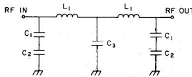
Figure 2-12. Simplified version of the circuit in state  $V_1$  is equal to zero and  $V_2$  is below the pinch-off [9].
