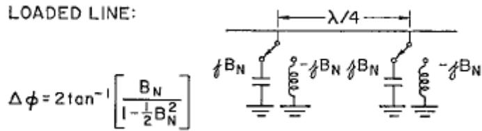
Figure 1-4. The Loaded Line Phase Shifter Circuit [2].
