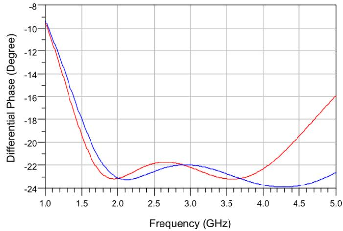
Figure A-14. The differential phase shift response of 2 to 4 GHz phase shifter 22.5° phase shift bit layout considered, and iterated shunt MIM capacitors (red line represents the present case, and blue line represents the ideal case).
