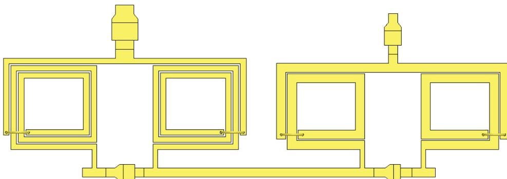
Figure 5-21. Upper branch of 1 to 2 GHz phase shifter 45° phase shift bit (Length: 5.476 mm, Width: 1.932 mm, Separation between inductors: 332 μm).
