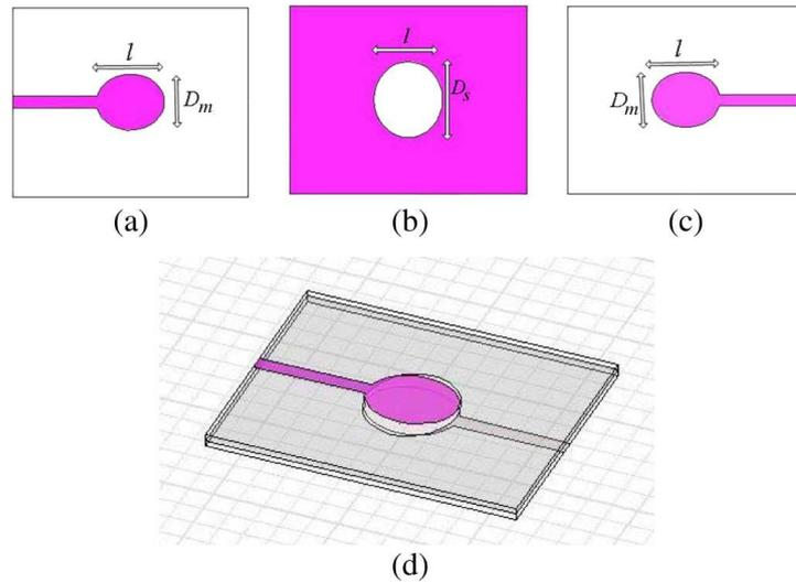
Figure 2-4. Configuration of the proposed phase shifter (a) Top layer (b) Mid layer (c) Bottom layer (d) Whole structure [6].
