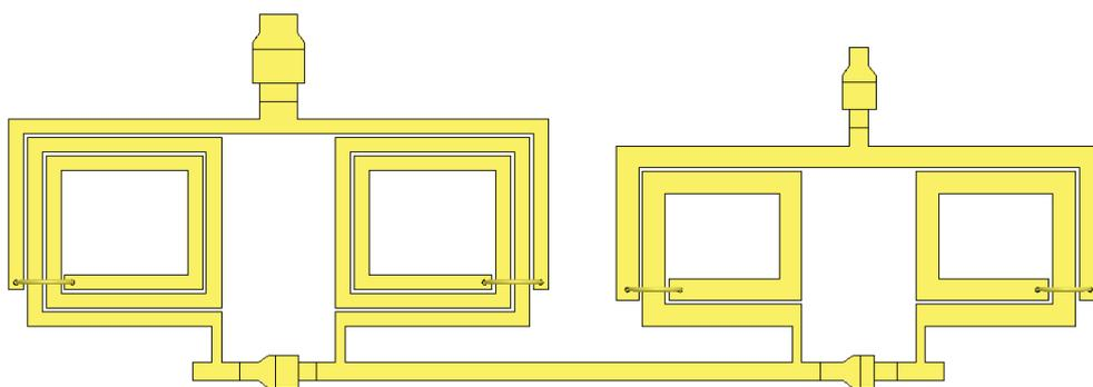
Figure 5-25. Upper branch of 1 to 2 GHz phase shifter 22.5° phase shift bit (Length: 5.836 mm, Width: 2.051 mm, Separation between inductors: 364 μm).
