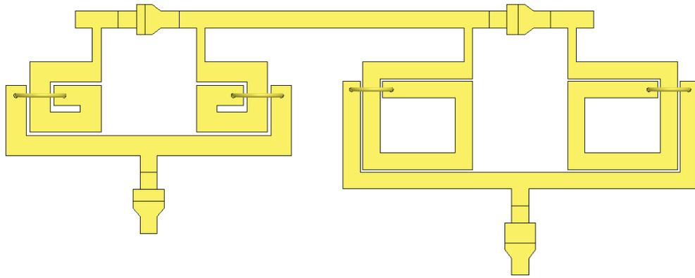
Figure B-16. Lower branch of 3 to 6 GHz phase shifter 22.5° phase shift bit (Length: 4.032 mm, Width: 1.604 mm, Separation between inductors: 300  $\mu\text{m}$ ).
