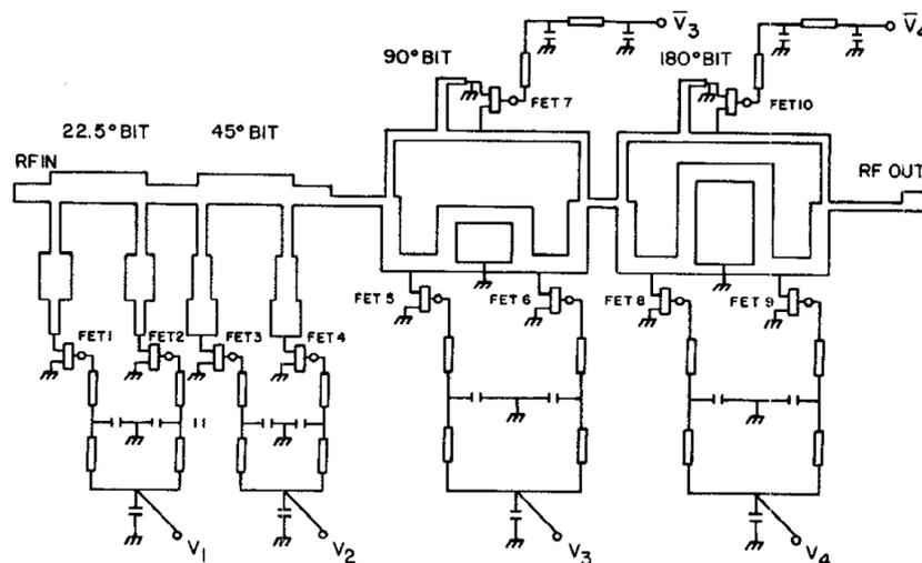
Figure 2-16. The schematic circuit diagram of the four-bit phase shifter [10].
