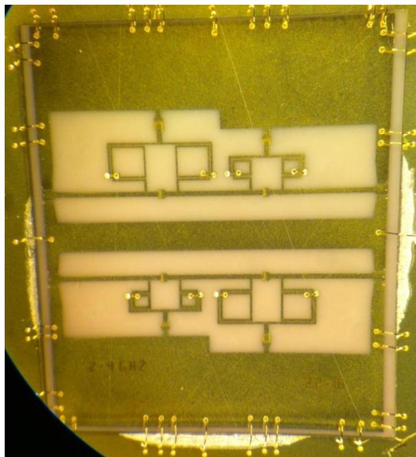
Figure 6-3. An example: Realized 2 to 4 GHz 22.5° Phase shift bit ready for measurement after post-processing.
