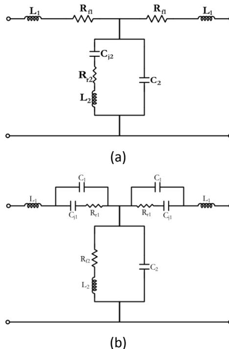
Figure 2-9. Bias States of the Proposed Phase Shifter (a) diodes-1 are forward biased and diode-2 is reverse biased (b) diodes-1 are reverse biased and diode-2 is forward biased.
