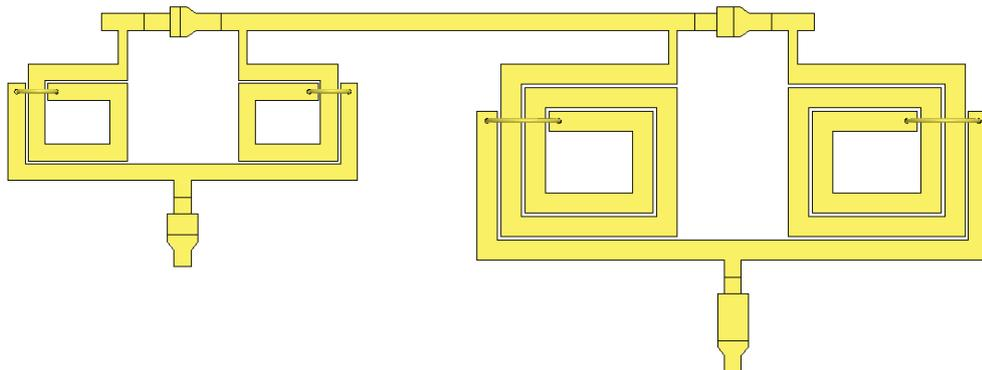
Figure 5-14. Lower branch of 1 to 2 GHz phase shifter 180° phase shift bit (Length: 5.722 mm, Width: 2.18 mm, Separation between inductors: 696  $\mu\text{m}$ ).
