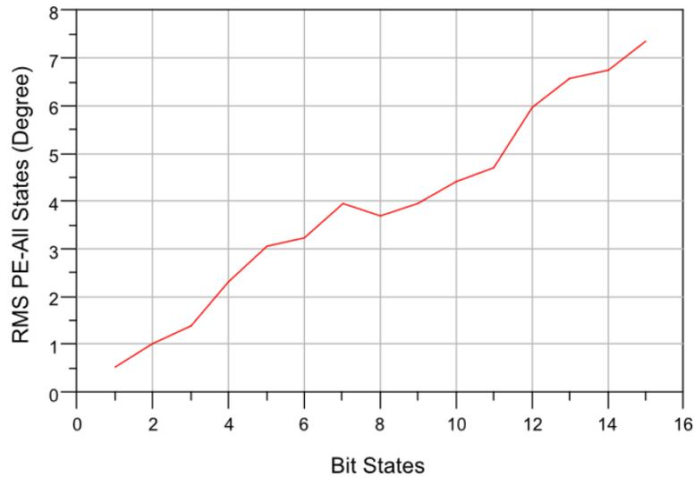
Figure 5-34. Phase rms error graph for bit states of 2 to 4 GHz 4-bit phase shifter.
