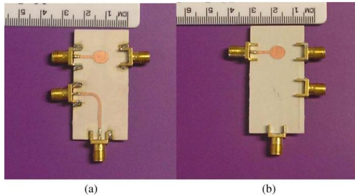
Figure 2-6. One of the manufactured phase shifters. (a) Top layer. (b) Bottom layer. The upper part of (a) and (b) is the phase shifter, where the reference transmission line is shown at the lower part of (a)[6].
