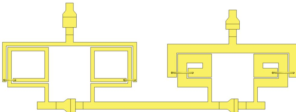
Figure B-11. Upper branch of 3 to 6 GHz phase shifter 45° phase shift bit (Length: 3.908 mm, Width: 1.48 mm, Separation between inductors: 406 μm).
