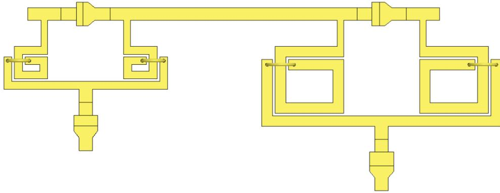
Figure B-4. Lower branch of 3 to 6 GHz phase shifter 180° phase shift bit (Length: 3.732 mm, Width: 1.45 mm, Separation between inductors: 706  $\mu\text{m}$ ).
