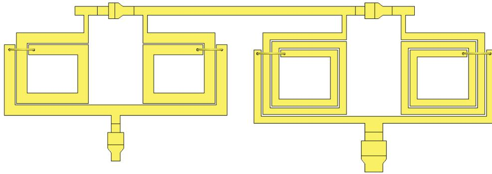
Figure 5-22. Lower branch of 1 to 2 GHz phase shifter 45° phase shift bit (Length: 5.504 mm, Width: 1.94 mm, Separation between inductors: 304  $\mu\text{m}$ ).
