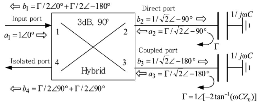
Figure 2-2. Schematic Diagram of a Hybrid Coupled Phase Shifter with Capacitive Reflective Loads [5].
