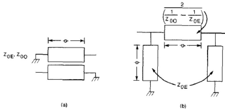
Figure 2-1. (a) Shorted Coupled Lines Sections (b)  $\pi$  Network Transmission Line Section [4].
