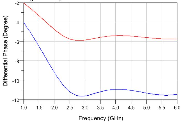
Figure 5-43. Differential phase graphs of 5.625° phase shift state (red line), and 11.25° phase shift state (blue line) constructed with ideal elements.
