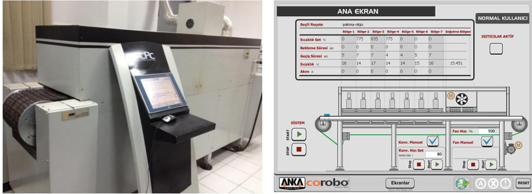
Figure 3.6 a) Photograph of firing furnace used in this study and b) a snapshot of the control software.
