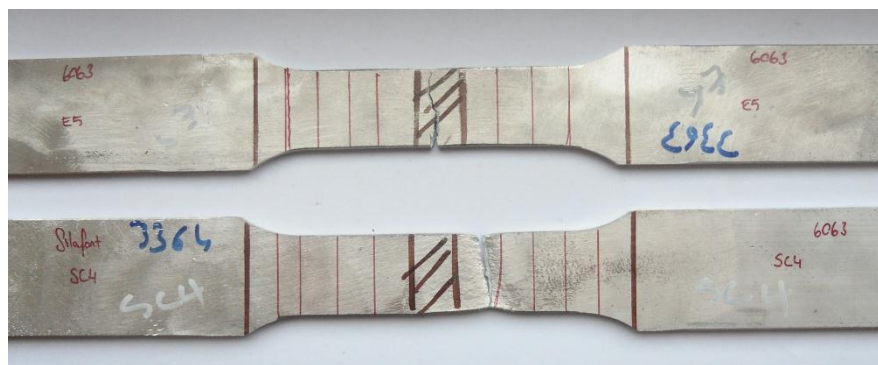
Figure 42: Welded samples after failed in tensile test, (top) extruded – extruded sample, (bottom) extruded – sand cast sample
