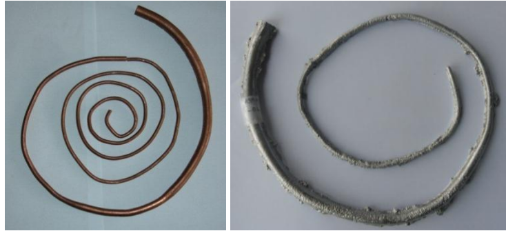
Figure 27: (left) The model of spiral fluidity that was used in sand molding, (right) spiral cast of A390.0 alloy after pouring
