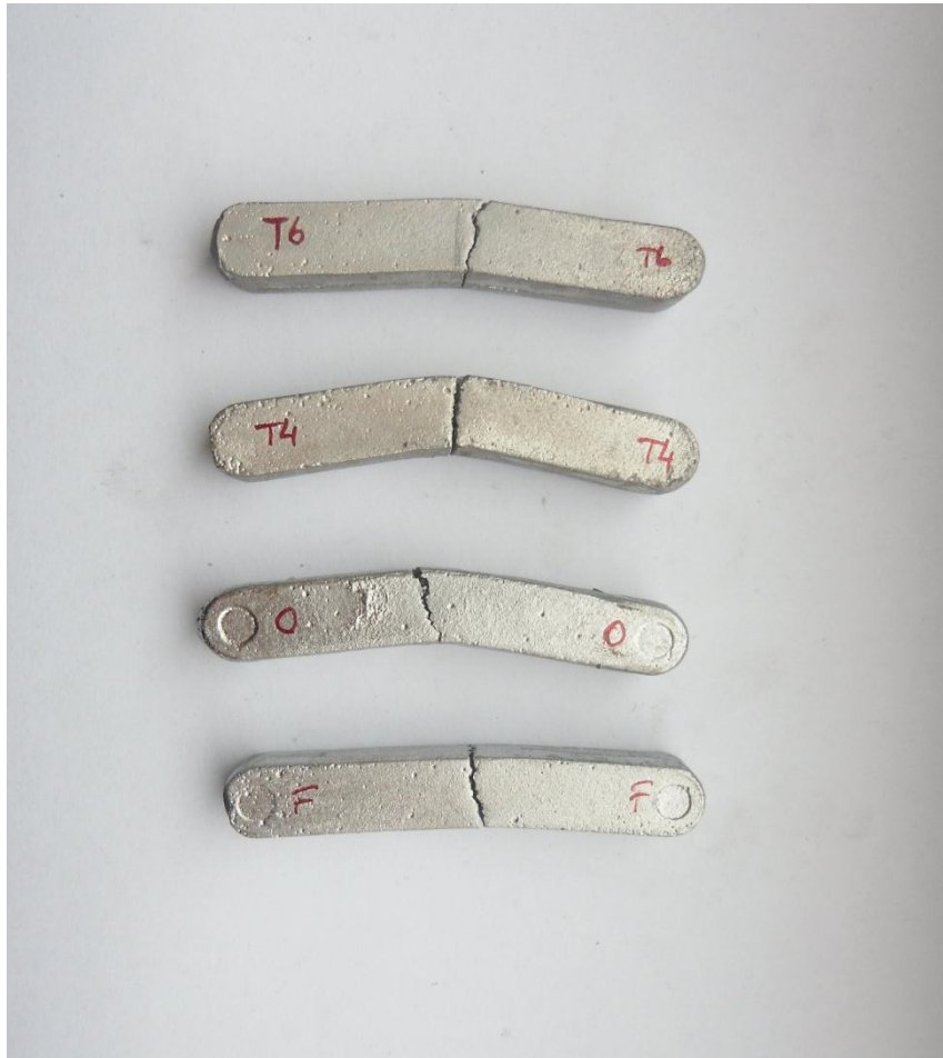
Figure 56: Broken Charpy impact test samples. (From top to bottom) T6 heat treated sample, T4 heat treated sample, annealed heat treated sample and untreated sample
