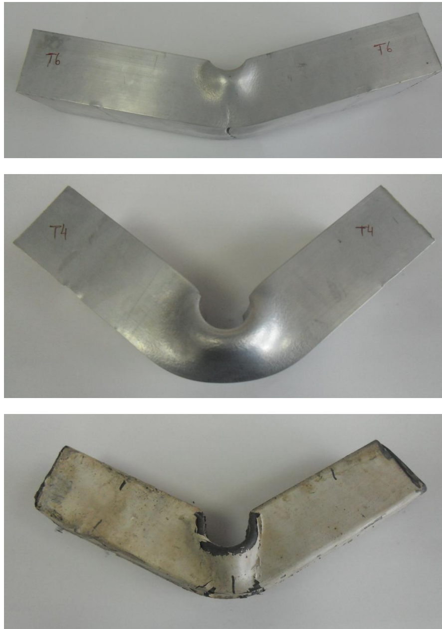
Figure 57: Deformed 3 – point bending samples. (From top to bottom) T6 heat treated aluminum profile, T4 heat treated aluminum profile, low carbon steel profile
