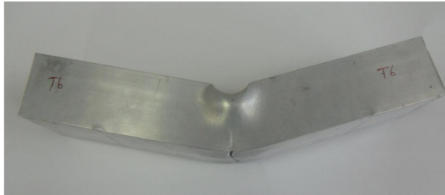
Figure 38: Deformed T6 heat treated profile view after 3-point bending test
