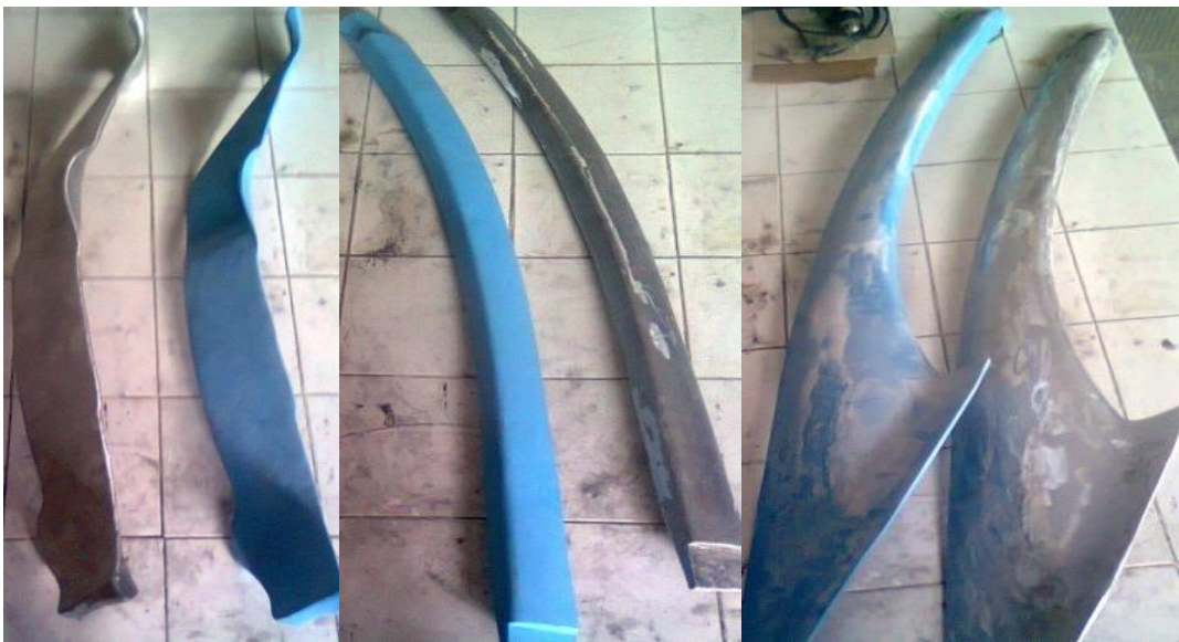
Figure 29: As cast parts of space frame with Silafont – 36 aluminum alloy and their patterns; a) A-pillar, b) B-pillar, c) C-pillar, d) front frame support, e) rear frame support (continued)
