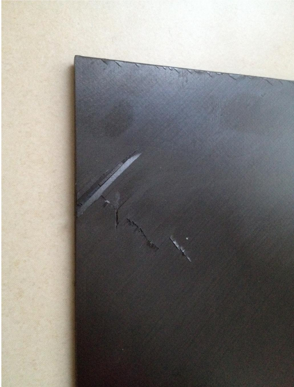
Figure 57. Failure path of UD-1
