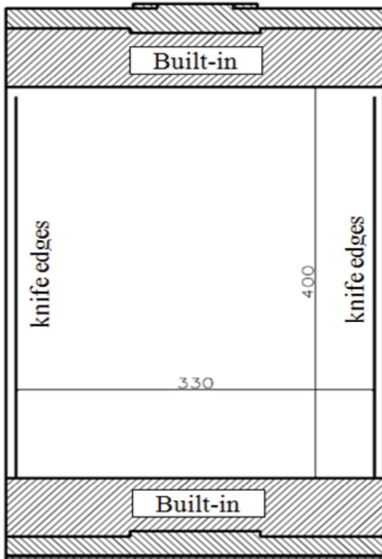
Figure 36. Panel Geometry and Boundary Conditions
