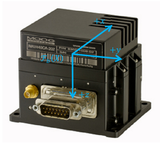
Figure 5.7 The IMU and the body frame attached to it [16]
