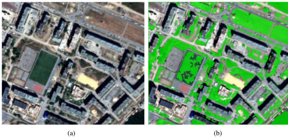
Figure 4.2: Wet soil detection example. (a) Sample image having wet soil regions. (b) Regions detected using boosted- NDVI thresholding ( b = 20 , T_{b-NDVI} = 0.5 ).
