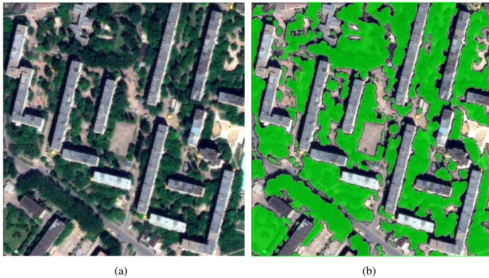
Figure 4.1: Vegetation detection example. (a) Sample image with large vegetation area. (b) Vegetation regions detected using NDVI thresholding.
