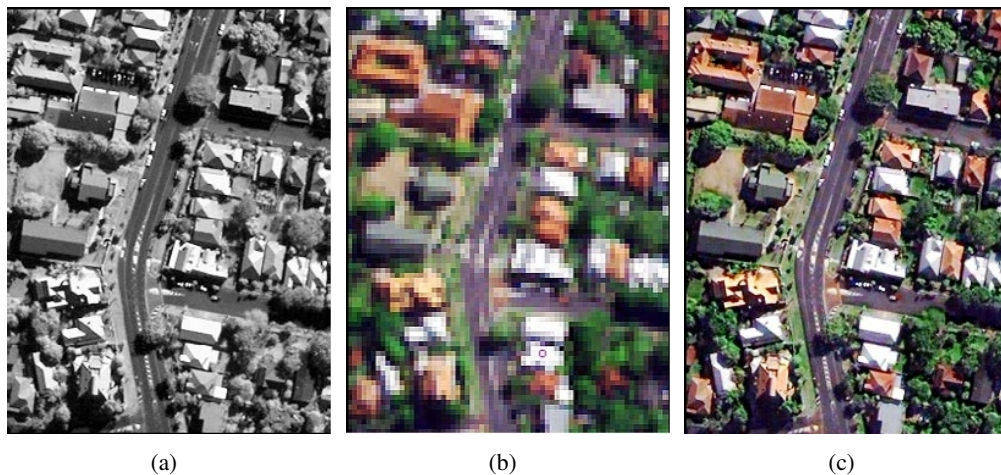
Figure 3.3: Pansharpening process applied on a satellite image. (a) High-resolution panchromatic image. (b) Low-resolution multispectral image. (c) Resulting high-resolution pansharpened image.
