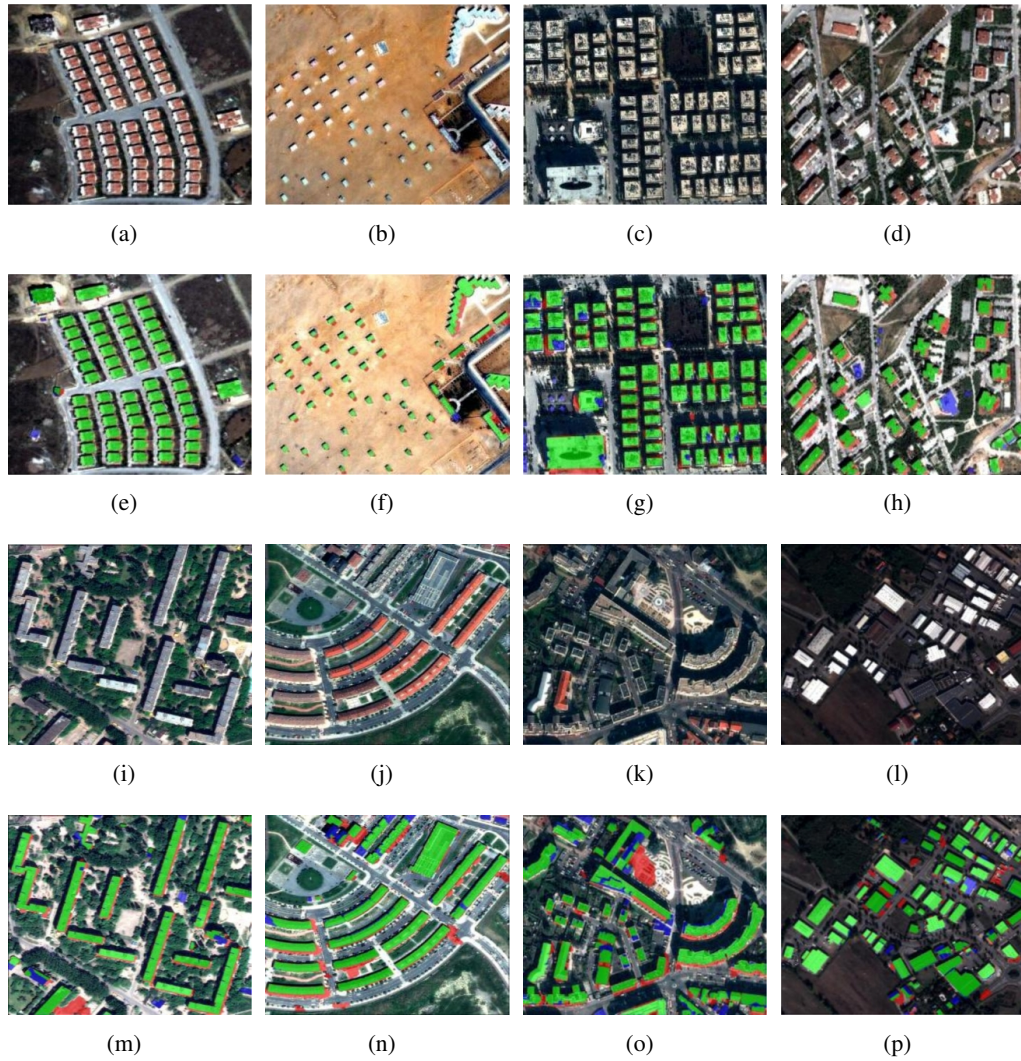
Figure 7.1: Visual detection results with respect to ground truths. The original images are shown in odd rows, the detection results are shown in even rows. Green, blue and red pixels represent detection, miss and false alarm respectively.
