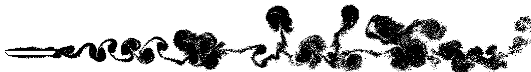
Figure 4-2 Flow pattern for the velocity 5.5 m/s at non-dimensional time 10
