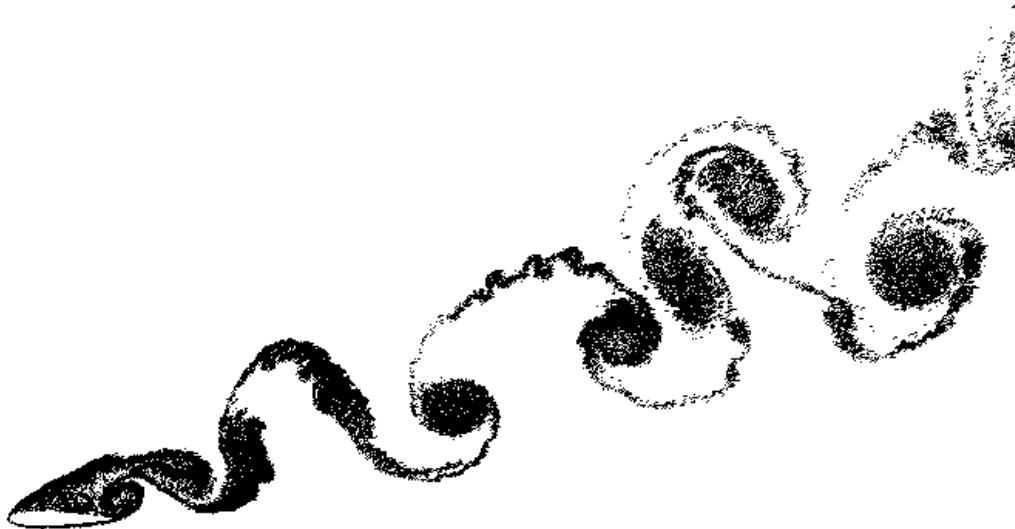
Figure 3-18 Flow around NACA 0012 airfoil at non-dimensional time 20 for Re = 10\ 000 , at angle of attack 20^\circ
