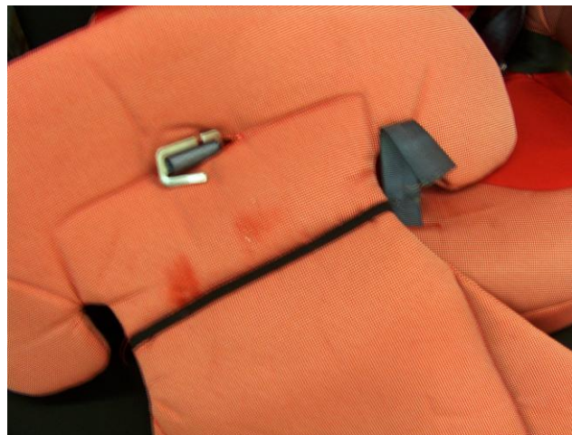
Figure 5.14 CRS D Seat Belt Failure
