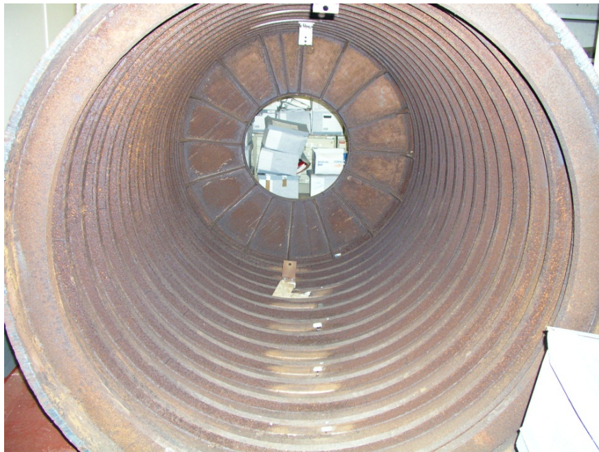
Figure 4-2 Ring stiffened submarine view [36]
