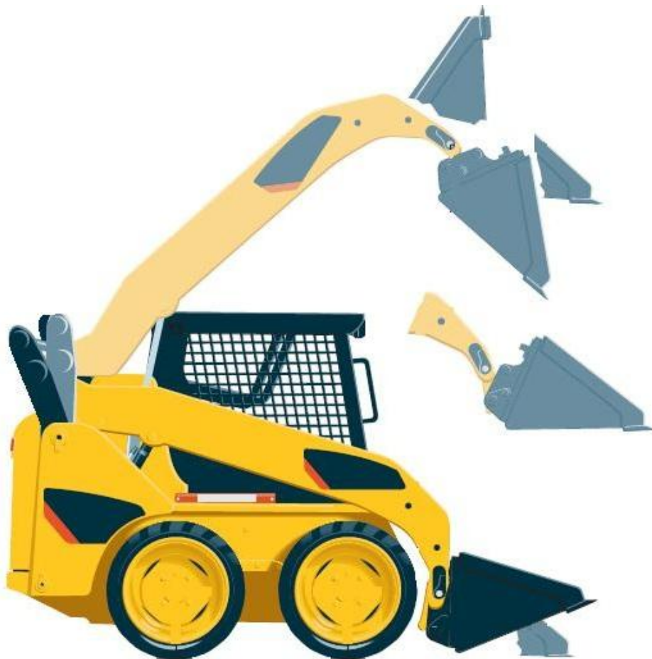
Figure 3-5 – A design criterion - the position of the connecting rods [52]
