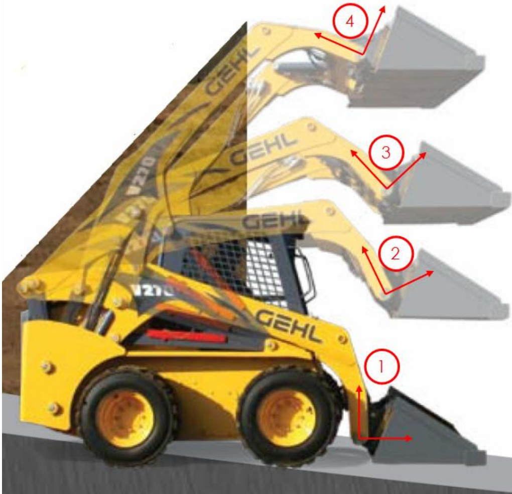
Figure 3-2 – A design criterion - the path of the hinge pin [50]
