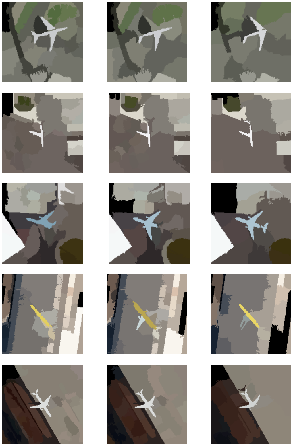
(a) (b) (c) Figure 12 : Mean-shift segmentation results for plane images (minimum segment area = 320) (a) h_s = 7 and h_r = 6.5 (b) h_s = 10 and h_r = 9.5 (c) h_s = 17 and h_r = 16.5
