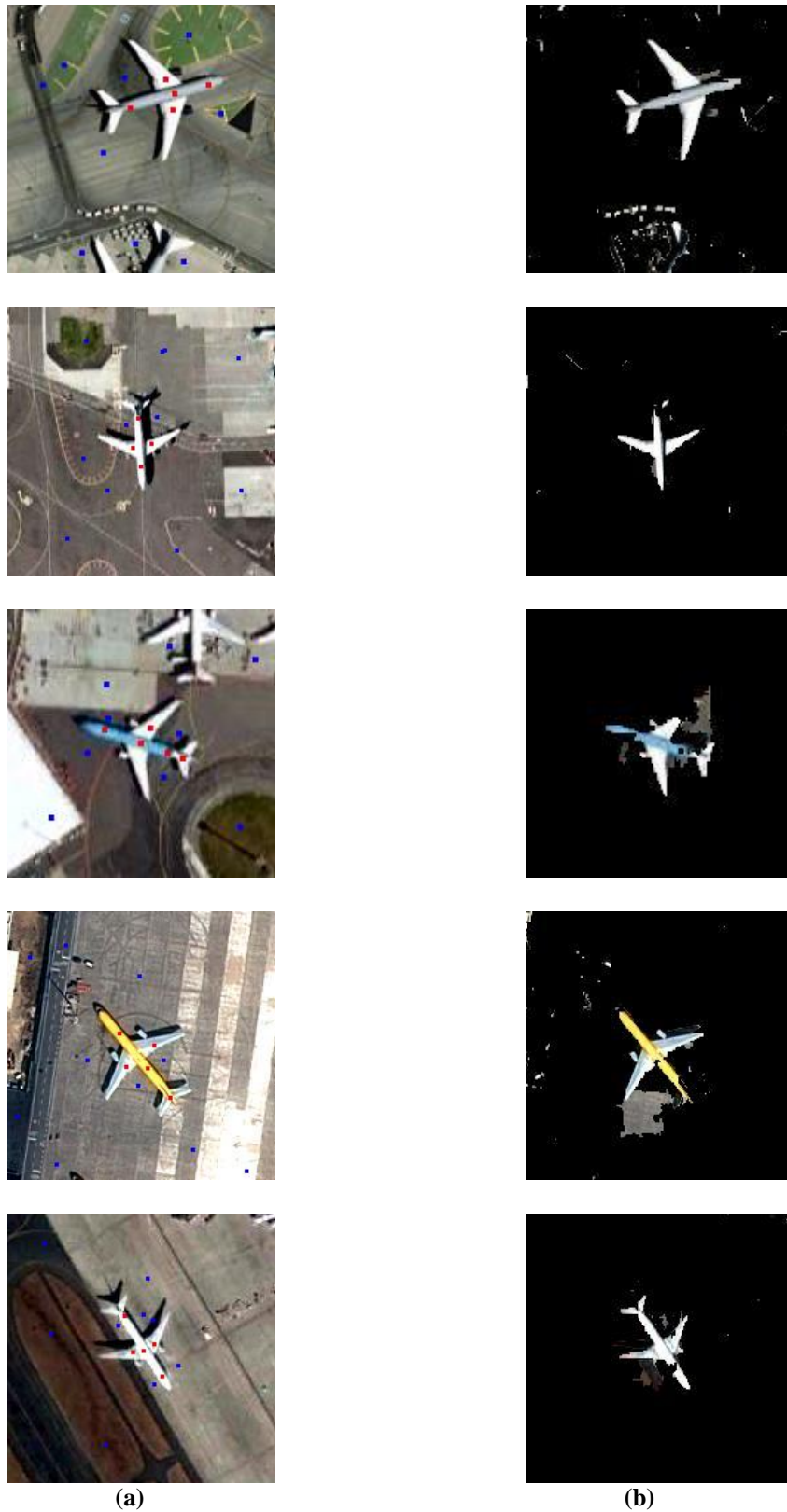
Figure 16 : Interactive graph-cuts segmentation results for plane images (a) The user input (b) The segmentation results
