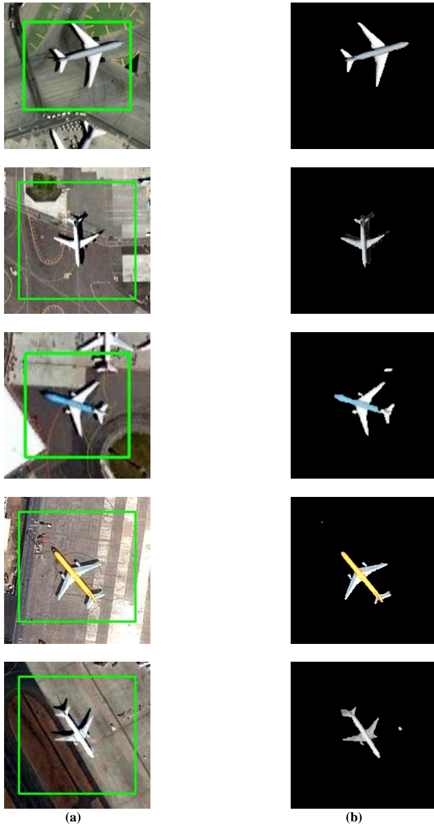
Figure 20: Interactive GrabCut segmentation results for plane images (a) The user input (b) The segmentation results
