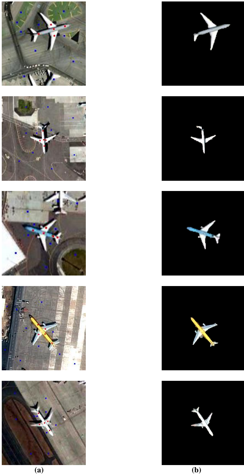
Figure 18: Interactive GrowCut segmentation results for plane images (a) The user input (b) The segmentation results
