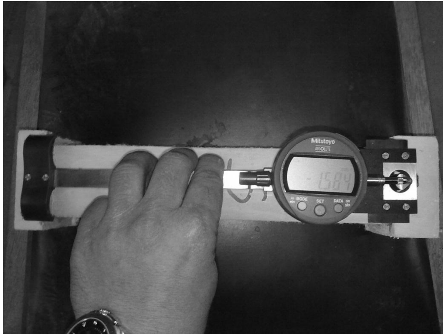
Figure 3.16 Measurement with DEMEC digital mechanical strain gage
