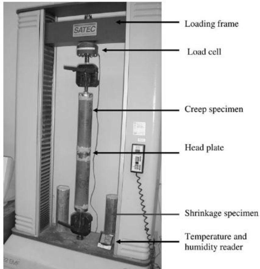
Figure 2.18 Setup for tensile creep test (Garas et al., 2009)
