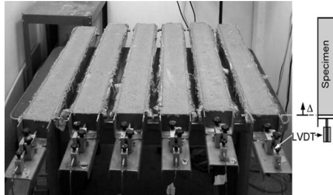
Figure 2.13 Free shrinkage specimens (Wongtanakitcharoen and Naaman, 2007)
