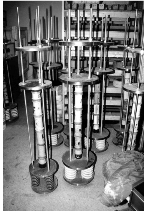
Figure 2.16 ASTM C 512 test setup of creep under compression (ASTM, 1987)
