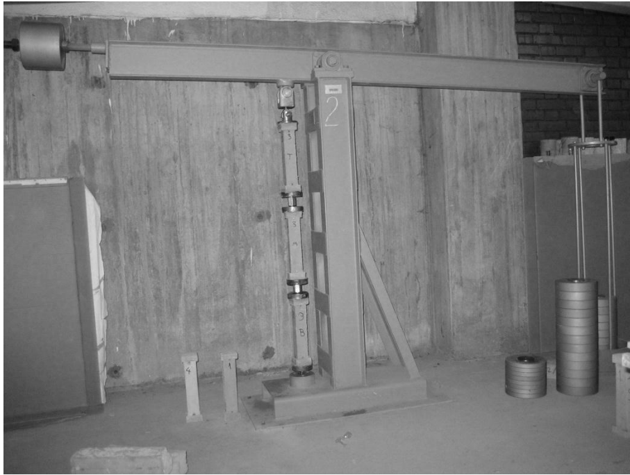
Figure 3.11 Tensile creep loading frame
