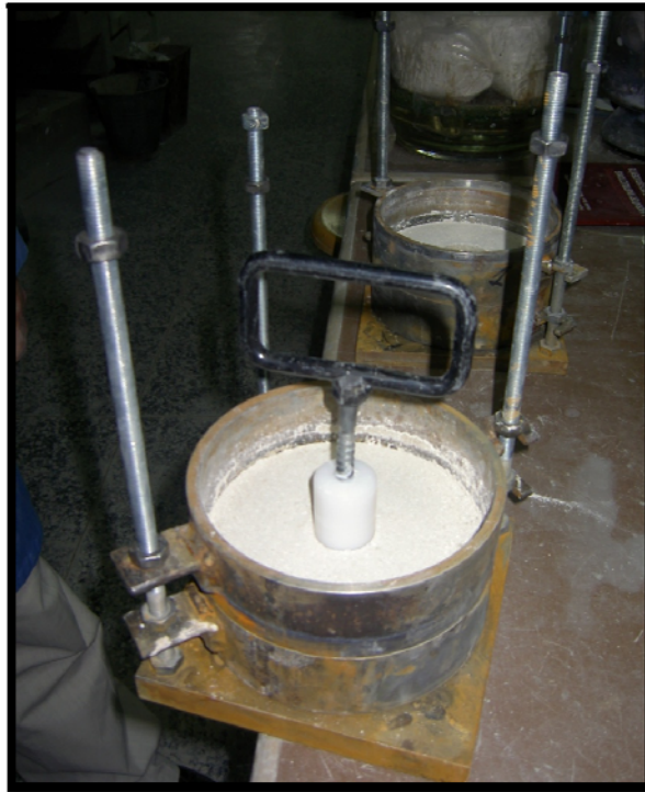
Figure 4. 28 Extraction of Cylindrical Mould from the Specimen
