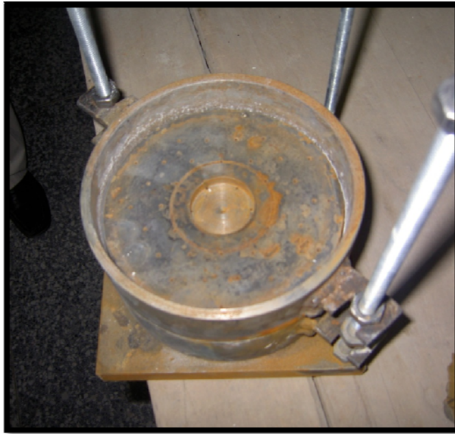
Figure 4. 32 Top Cap Placed on CBR Specimen
