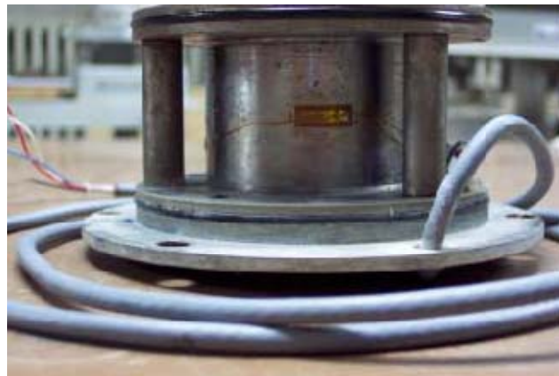
Figure 3. 7 An Active Strain Gauge on the Thin-Wall Ring (Ertekin, 1991)
