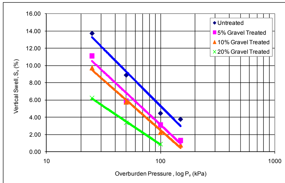
Figure 5. 14 Vertical Swell Percentage vs. Overburden Pressure for Oedometer Tests Performed with Swell Overburden Testing Technique on Type-2 Expansive Soil Samples Improved by Gravel
