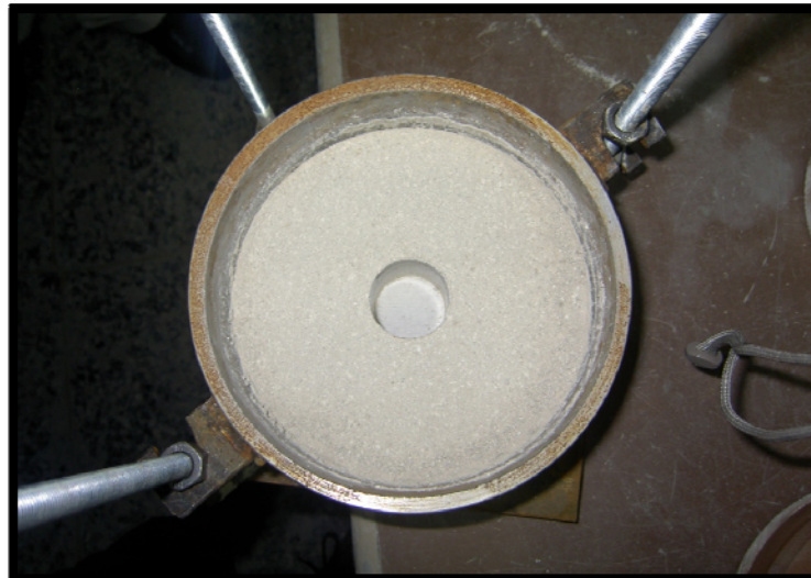
Figure 4. 29 Hole inside CBR Specimen
