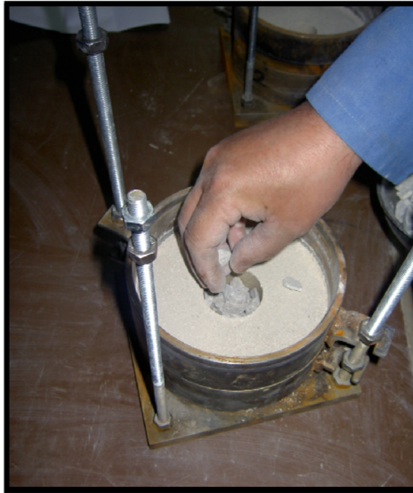
Figure 4. 30 Placement of Granular Material into Hole in CBR Sample
