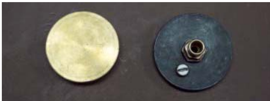
Figure 3. 9 Bottom Cap (Left) and Top Cap (Right) with Supply (Center) Inlet and Release (Outlet) Points
