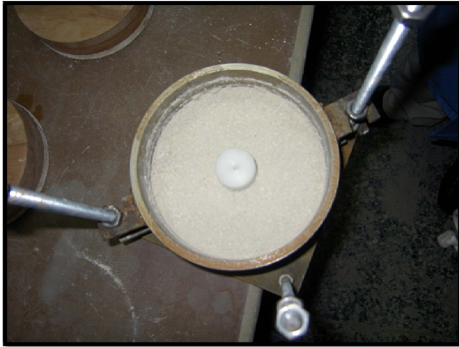
Figure 4. 27 Sample Compacted inside CBR Mould
