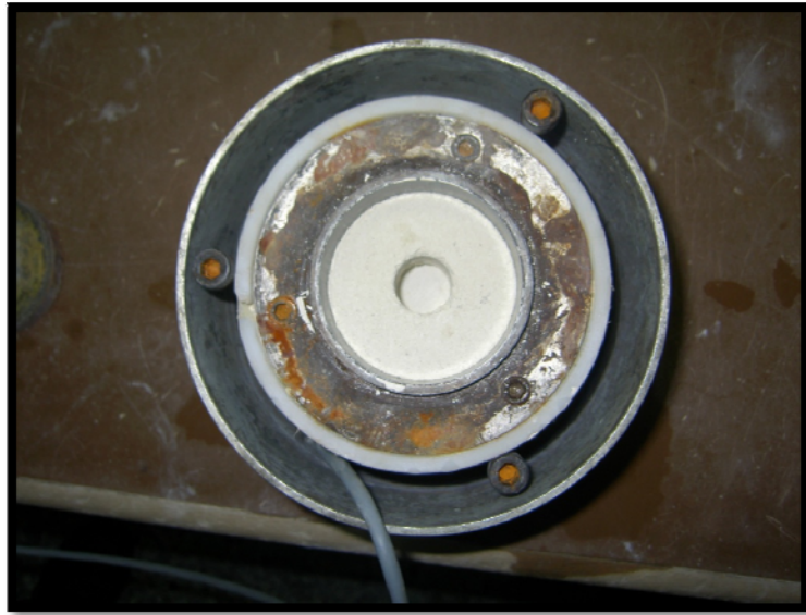
Figure 4. 22 Hole Opened inside Specimen to Construct Granular Column
