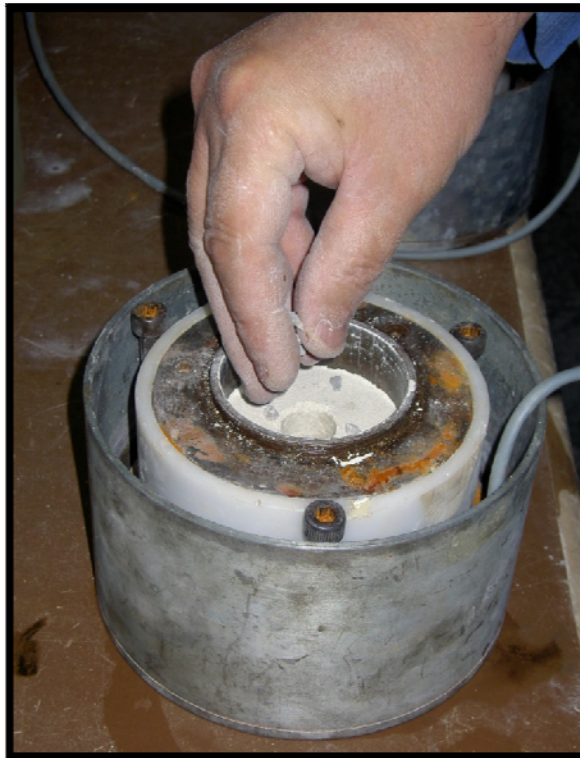
Figure 4. 23 Placement of Granular Soil inside the Hole
