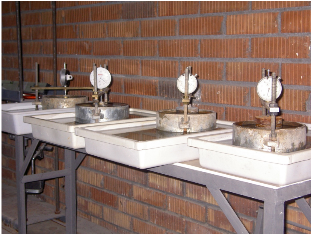
Figure 3. 12 Modified CBR Moulds with Inundation Containers
