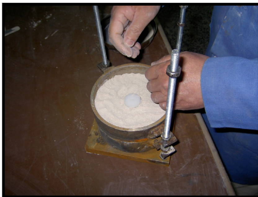
Figure 4. 25 Placement of Sample inside Modified CBR Mould
