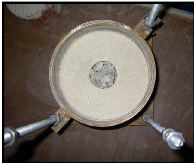
Figure 4. 31 Hole Filled with Granular Material in CBR Sample
