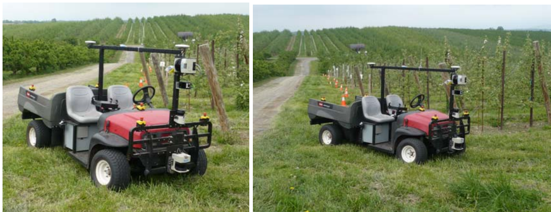
Figure 7.2: Toro MDE eWorkman based autonomous vehicle
