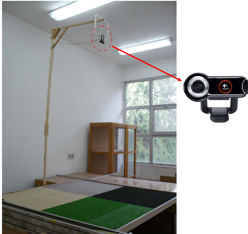
Figure 4.6: Experimental surface and camera located at the top of the surface
