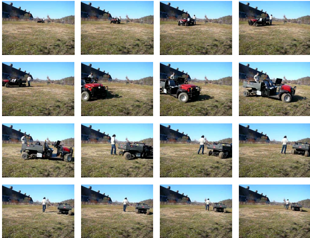
Figure 8.14: Video frames showing turning procedure of the vehicle (the human is walking near by the vehicle for safety reasons and is not interfering the vehicle)
