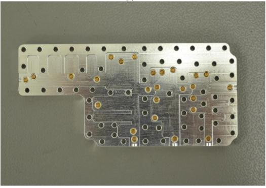
(c) Figure 5.16 Measurement results and layout for manifold for odd numbered channels (continued) (b) Manifold Layout (c) Top Cover
