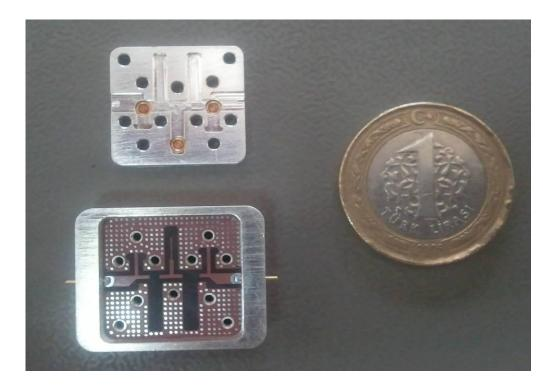
(a) Figure 4. 9 (a) 14 GHz HP filter module
