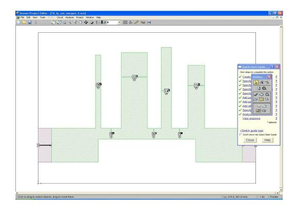
Figure 5.9 18 GHz LP filter : N-port SONNET layout
