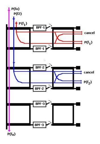
Figure 2. 10 A Switchable Hybrid Multiplexer
