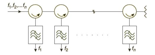
Figure 2. 11 A Circulator Coupled Multiplexer
