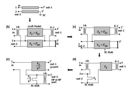
Figure 3. 10 Type-2 Series Diplexing Circuit
