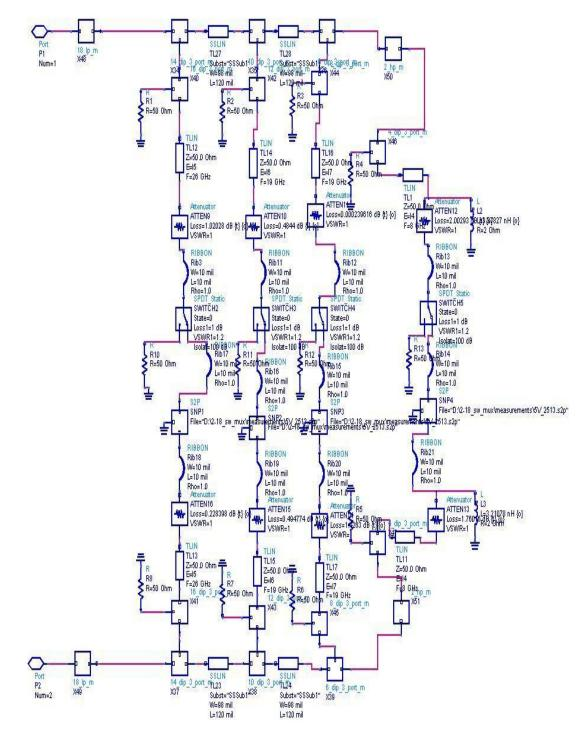
Figure 5. 40 Final SW\_MUX structure: odd half
