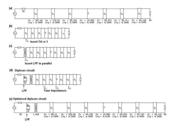
Figure 3. 15 Formation of the Diplexer with T-junction
