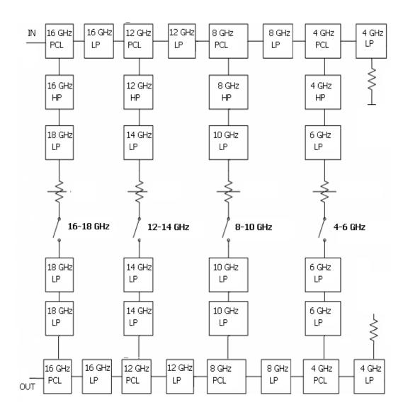
Figure 2. 16 Even Half of SW\_MUX with LP filter
