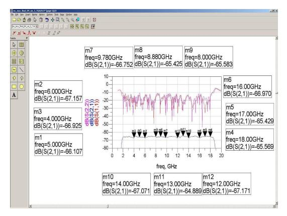
Figure 5.44 Response when all channels are OFF
