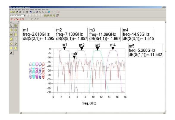
Figure 5.22 ADS results for multiplexer containing odd numbered channels
