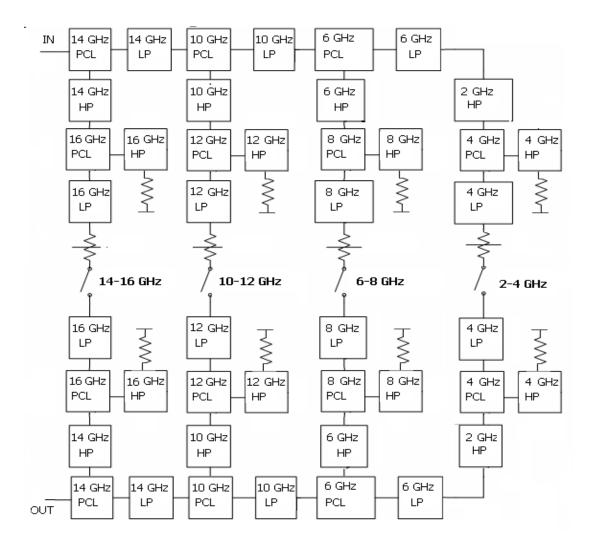
Figure 2. 20 Odd Half of SW\_MUX with diplexers in place of extra attenuators.
