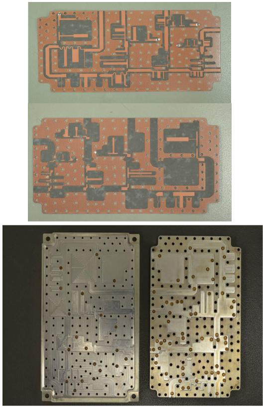
(b) Figure 5. 26 Measurement results and layout for multiplexer containing even numbered channels: (b) module decomposed
