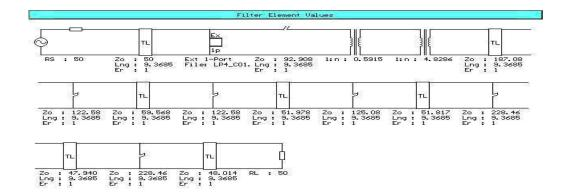
Figure 3. 21 . Final HP channel schematics for Option-2
