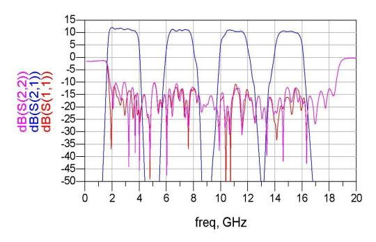
Figure 5. 37 Even channel SW\_MUX with amplifiers: results
