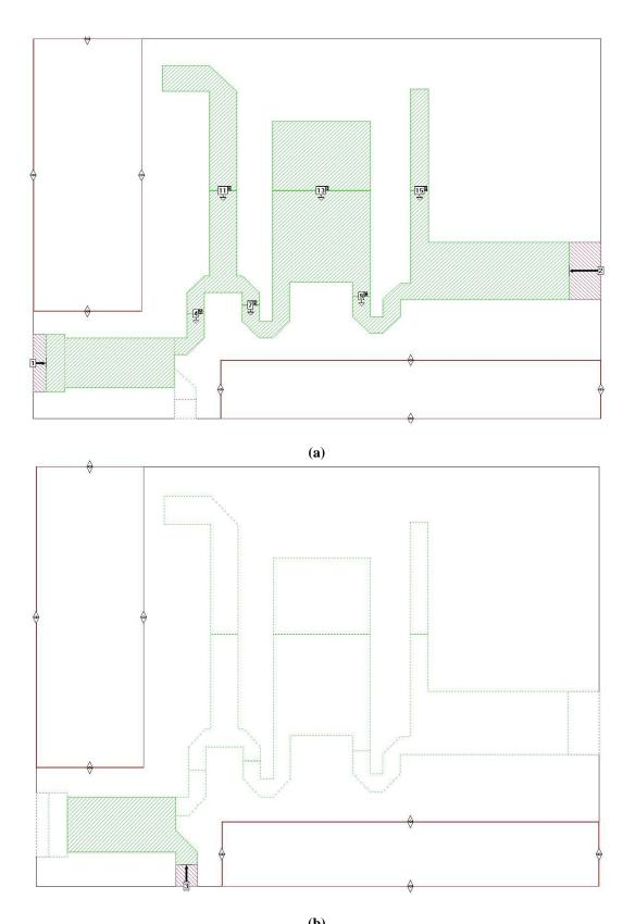
(b) Figure 4. 16 (a) top section of LP Channel of 6 GHz diplexer (b) bottom side of LP channel of 6 GHz diplexer
