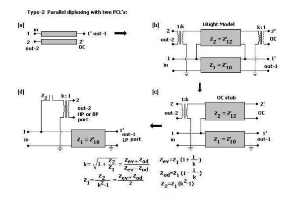
Figure 3. 12 Type-2 Parallel Diplexing Circuit
