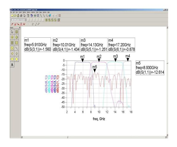
Figure 5. 18 ADS Simulation of the manifold for even numbered channels
