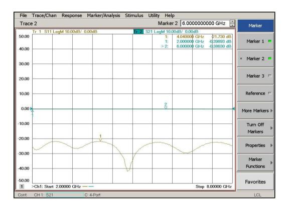
(c) Figure 5.8 Manufactured 2 GHz HP filter (continued): (c) measurement results
