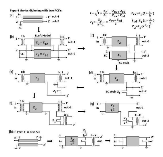
Figure 3. 8 Type-1 series diplexing PCL circuit
