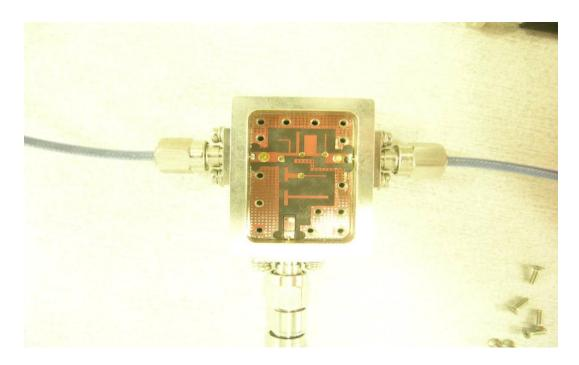
Figure 5.2 12 GHz Diplexer Layout
