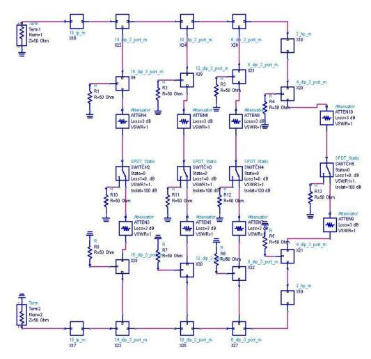
Figure 5. 31 Odd channel SW\_MUX with attenuators
