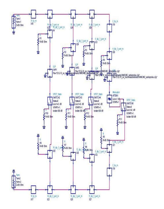
Figure 5. 35 Odd channel SW\_MUX with amplifiers
