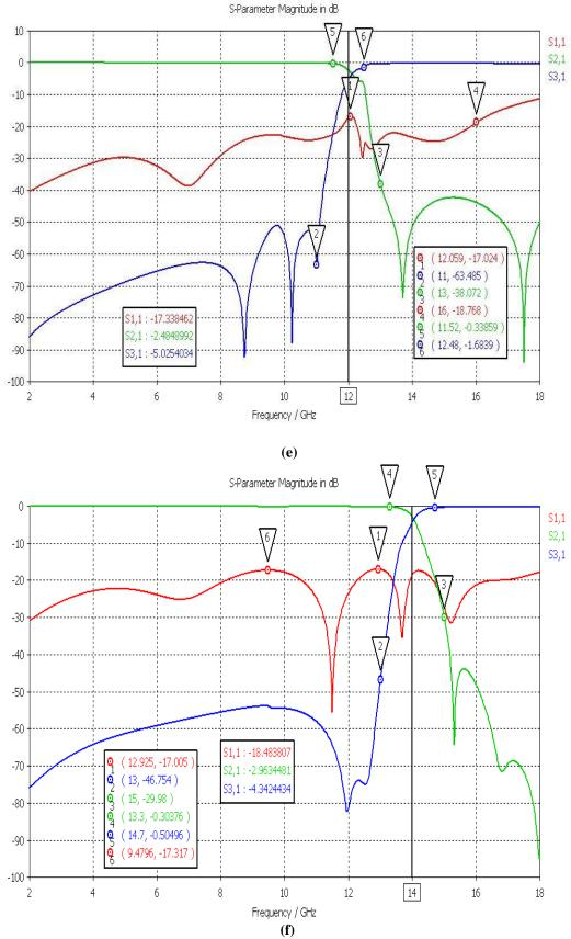
Figure 4.20 (continued) e) response of 12 GHz diplexer (f) response of 14 GHz diplexer
