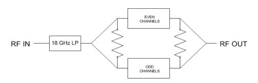
Figure 2. 18Connection of even and odd channel multiplexers through splitters.
