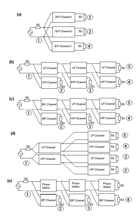
Figure 2.2 Typical Parallel Connected Multiplexer Structures (a) Parallel Bandpass Filter Multiplexer, (b) Ladder Type Lowpass-Highpass Multiplexer, (c) Bandpass-Bandstop and Lowpass Multiplexer, (d) Tree Type Multiplexer using Lowpass-Highpass Diplexers and (e) Manifold Type Multiplexer
