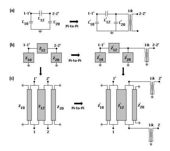
Figure 3. 5. Pi to Pi Transformatiom applied on a coupled line
