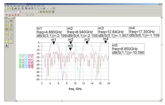
Figure 5.25 ADS results for multiplexer containing even numbered channels
