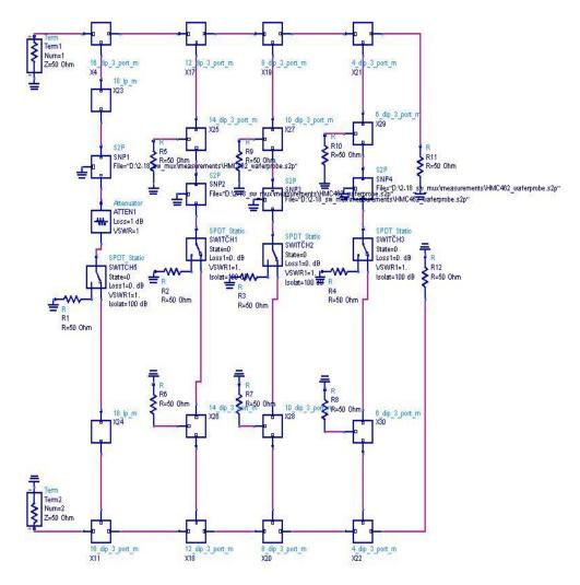
Figure 5. 38 Even channel SW\_MUX with amplifiers
