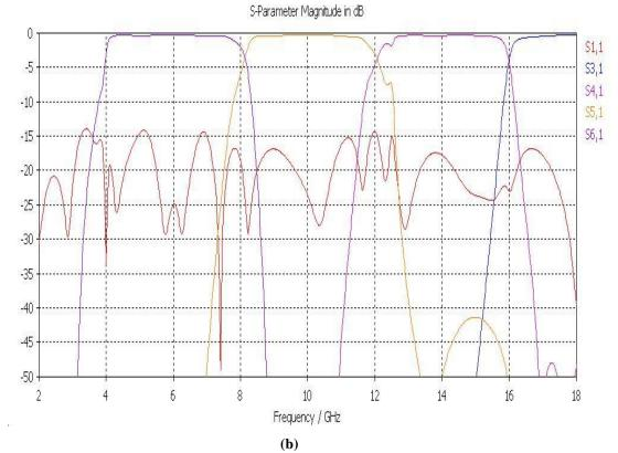
Figure 5. 19 CST layout and results for even numbered channels manifold (a) CST layout (b): CST results
