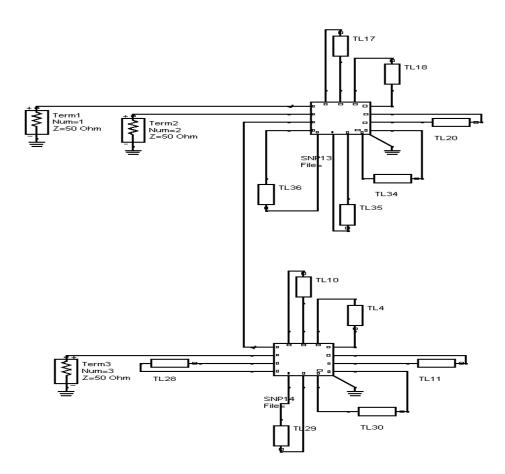
Figure 4. 15 N-port circuit for optimizing diplexer response
