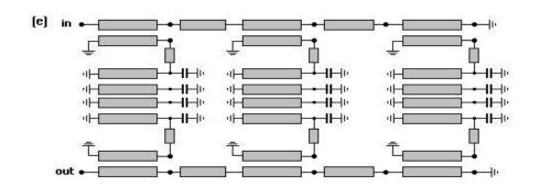
Figure 2. 13 (a) Series Diplexing PCL and Its Equivalent Circuit, (b) Series Multiplexing Structure (a Triplexer), (c) Equivalent Circuit of Series Multiplexer, (d) A Single Input-Single Output Switched Multiplexer and (e) A Possible Realization Layout Using Combline Filters
