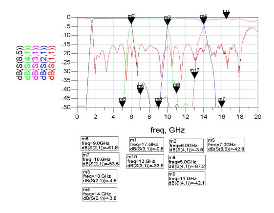
Figure 5. 16 Measurement results and layout for manifold for odd numbered channels (a) Measurement Results
