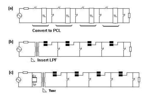
Figure 3. 24 Design steps for HP channel and diplexer
