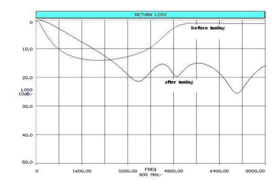
Figure 3. 16 . Return Loss of the diplexer with t-Junction before and after tuning
