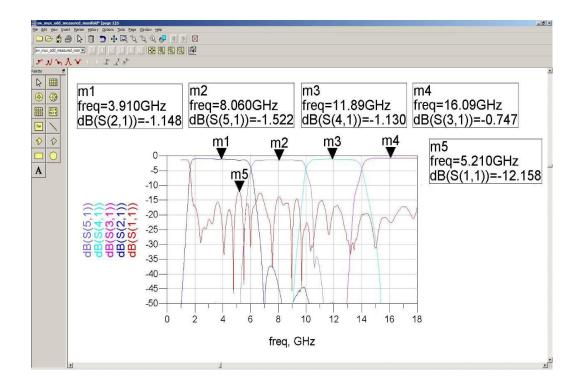
Figure 5. 14 ADS Simulation of the manifold for odd numbered channels
