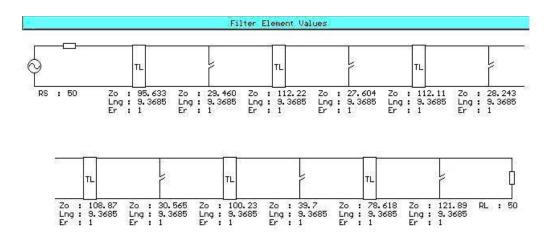
Figure 3. 22 LP channel schematics
