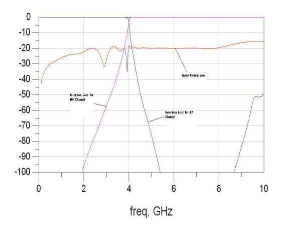
Figure 3. 29. Diplexer response after optimization in ADS
