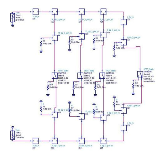
Figure 5. 27 Odd channel SW\_MUX 137
