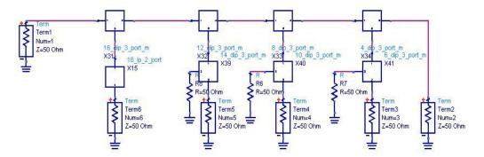
Figure 5.24 Multiplexer containing even numbered channels
