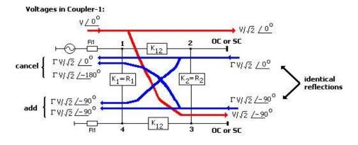
Figure 2. 9 Power Flow in One Channel of Hybrid Manifold Multiplexer
