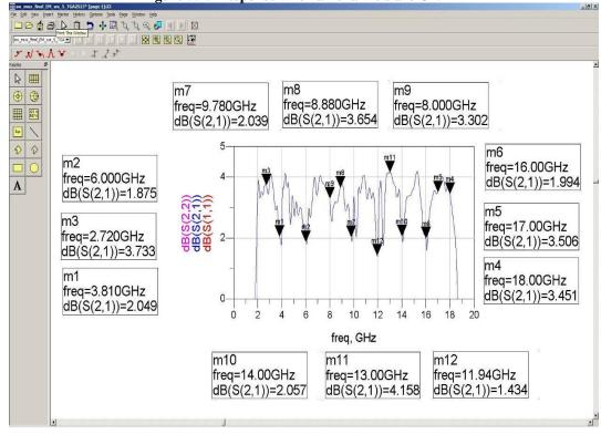
Figure 5.46 Insertion Loss when all channels are ON: zoomed
