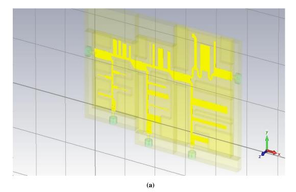
Figure 5.15 ( a) Manifold for odd numbered channels : CST layout
