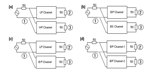
Figure 2.1 Some Parallel Connected Diplexers (a) Lowpass-Highpass Diplexer, (b) Bandpass-Bandstop Diplexer, (c) Lowpass-Bandpass Diplexer and (d) Bandpass-Bandpass Diplexer
