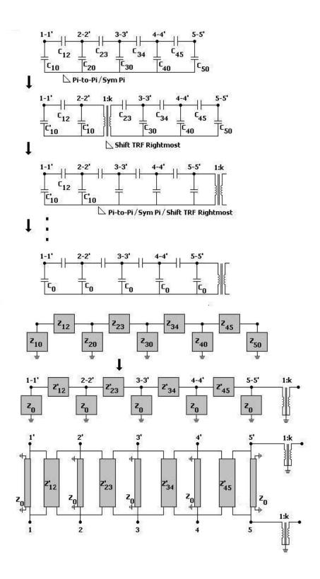
Figure 3. 6 Equating shunt impedances of an N-coupled line system for N=5
