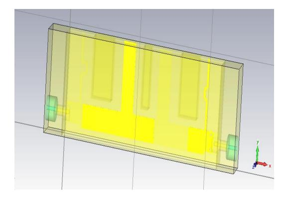
Figure 5.7 CST results and layout for 2 GHz HP filter (a) 2 GHz HP filter : CST layout
