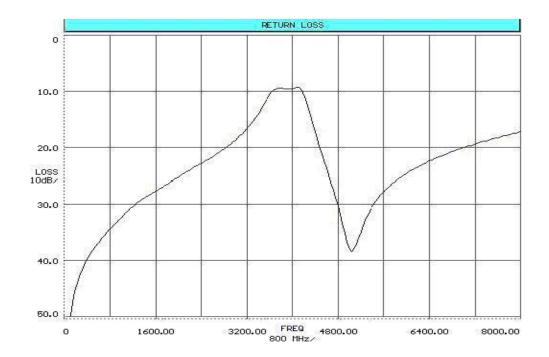
Figure 3. 25. Diplexer return loss after tuning transformer in HP channel
