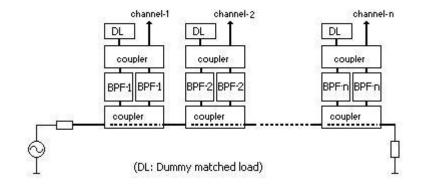
Figure 2. 7 Hybrid Coupled Manifold Multiplexer
