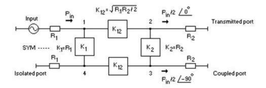
Figure 2. 8 Schematics of a 3 dB Impedance Transforming Branchline Coupler with Different Input-Output Terminations
