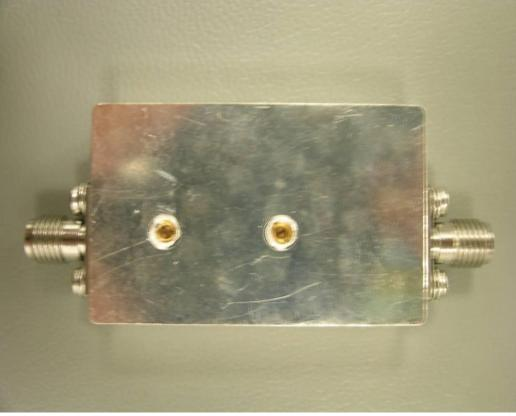
(b) Figure 5.8 Manufactured 2 GHz HP filter (continued): (b) Manufactured module
