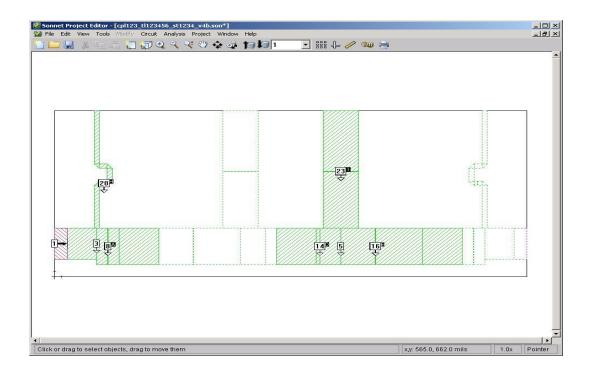
(a) 2 GHz HP filter N-port layout in SONNET: top side
