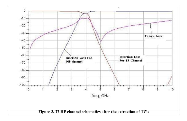
After 50 trials of optimization, the diplexer has return loss of 20 dB up to 8 GHz and, the highpass channel has a rejection greater than 50 dBc at 3 GHz and the lowpass channel has a rejection greater than 50 dBc at 5 GHz. In order to reach the 21 dB return loss goal the circuit has to be optimized several times more. The optimized circuit and its responses are given in Figures 3.27 and 3.28 respectively.
