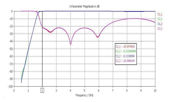
Figure 5.7 CST results and layout for 2 GHz HP filter (continued): (b) CST results
