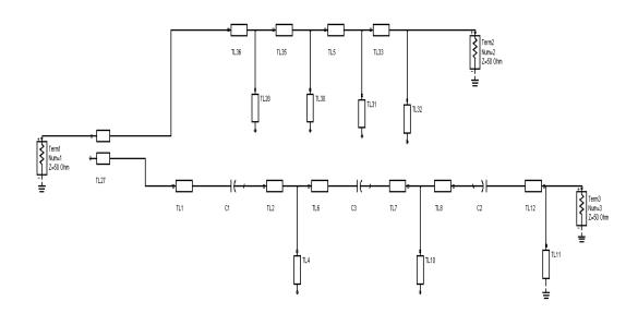
Figure 4. 13 ADS circuit of 6 GHz diplexer
