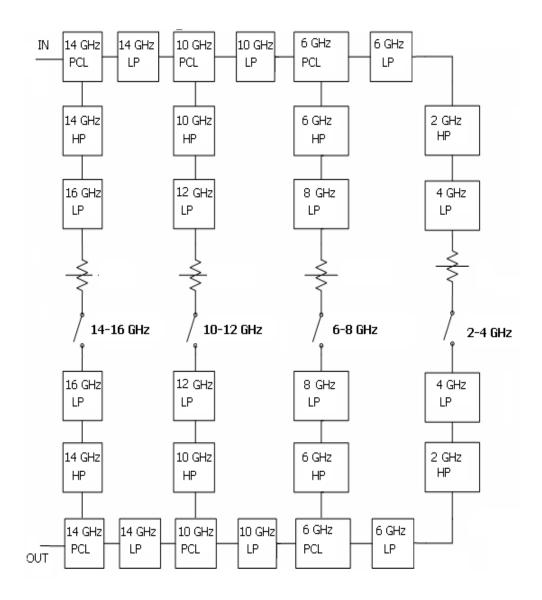
Figure 2. 17 Odd Half of SW\_MUX with LP filter
