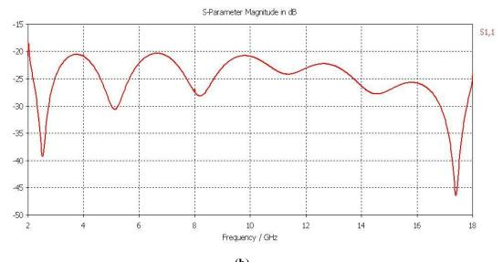
(b) Figure 5.12 2-18 GHz power divider (a) CST layout (b) Input return loss
