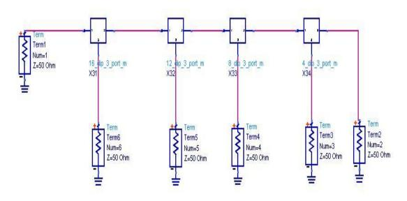
Figure 5. 17 Manifold for even numbered channels
