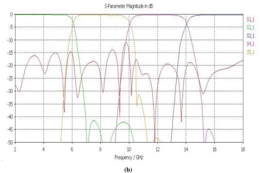
Figure 5.15 Manifold for odd numbered channels (continued) (b) CST results
