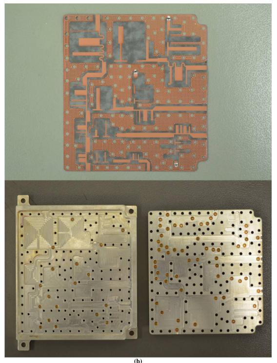
(b) Figure 5.23 Measurement results and layouts for multiplexer containing odd numbered channels: (b) Module decomposition
