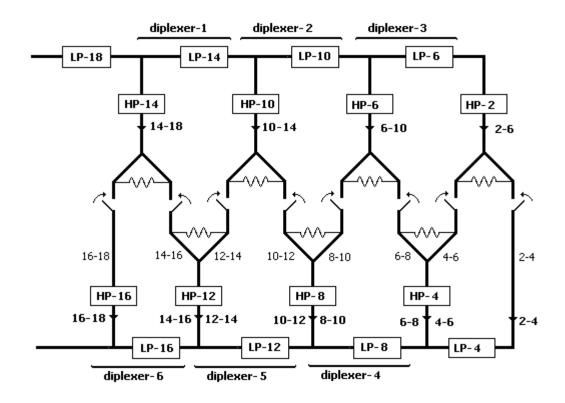
Figure 2. 5 An 8 Channel 2-18GHz SW\_MUX
