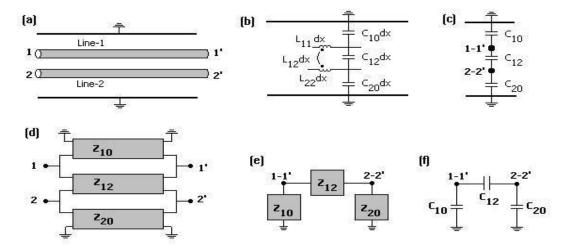
Figure 3. 1Three Line model of a parallel coupled line pair.
