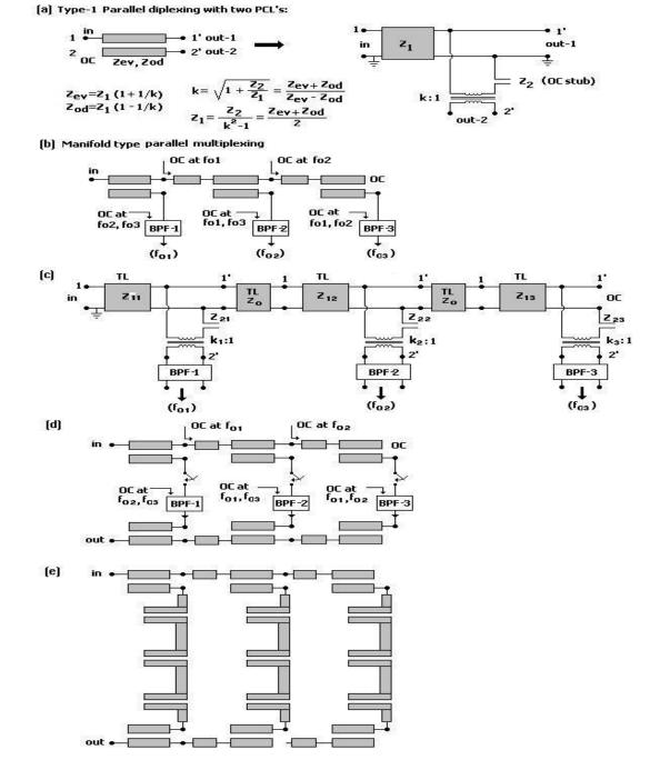
Figure 2. 14 a) Parallel diplexing PCL and its equivalent circuit. b) A parallel multiplexing structure (a triplexer). c) Equivalent circuit of parallel multiplexer. d) A single input-single output switched multiplexer. e) A possible realization layout using edge coupled line filters.
