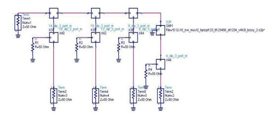
Figure 5.21 Multiplexer containing odd numbered channels
