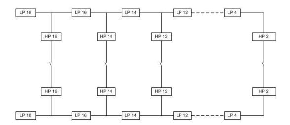
Figure 2. 3 A Simple SW\_MUX Based on LP-HP Diplexers
