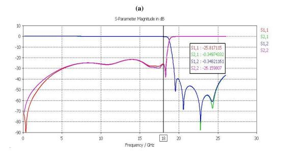
(b) Figure 5. 11 CST simulation results and 3-D structure for 18 GHz LP filter (a) 18 GHz LP filter: CST layout (b) 18 GHz LP filter : CST results
