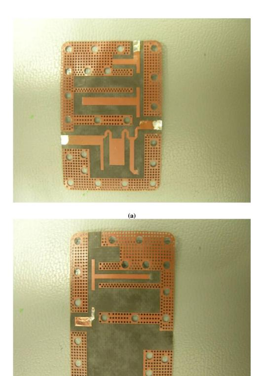
(b) Figure 4. 17 (a) top side for 6 GHz diplexer (b) bottom side for 6 GHz diplexer
