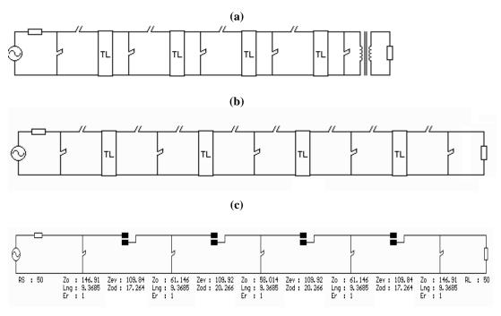
Figure 5. 4 Design of 2 GHz HP filter in FILPRO
