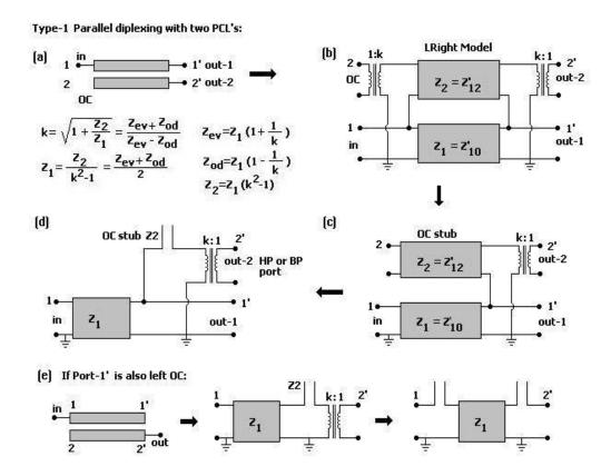
Figure 3. 11. Type-1 Parallel Diplexing Circuit
