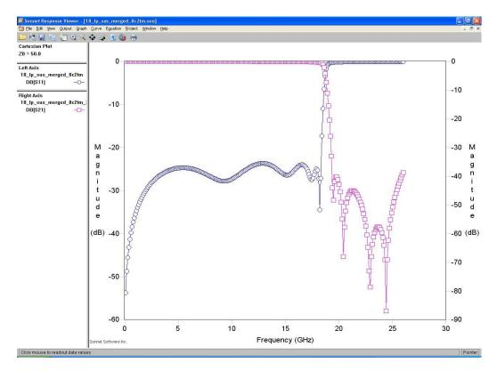
(b) Figure 5. 10 18 GHz LP filter (a) 18 GHz LP filter final circuit (b) 18 GHz LP filter final circuit: SONNET results
