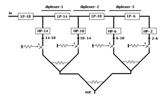
Figure 2. 4 A Switchable LP-HP Multiplexer Using Power Dividers
