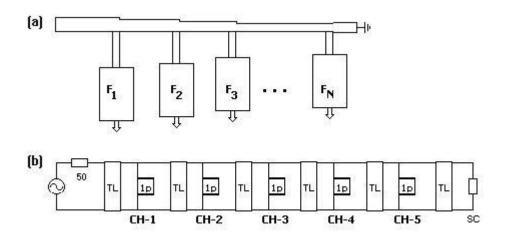
Figure 2. 6 A Manifold (Extended Junction) Stripline Multiplexer
