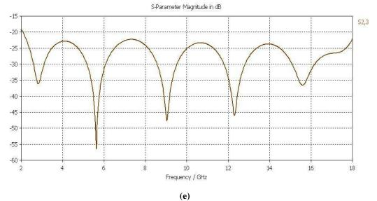
Figure 5. 12 2-18 GHz power divider (continued) (c) Insertion loss (d) Output return loss e) Isolation between output ports
