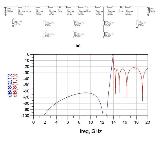
(b) Figure 4. 2 14 GHz diplexer (a) ADS schematic (b) the optimized response
