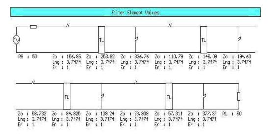
Figure 3. 23. HP channel schematics after the extraction of TZ's
