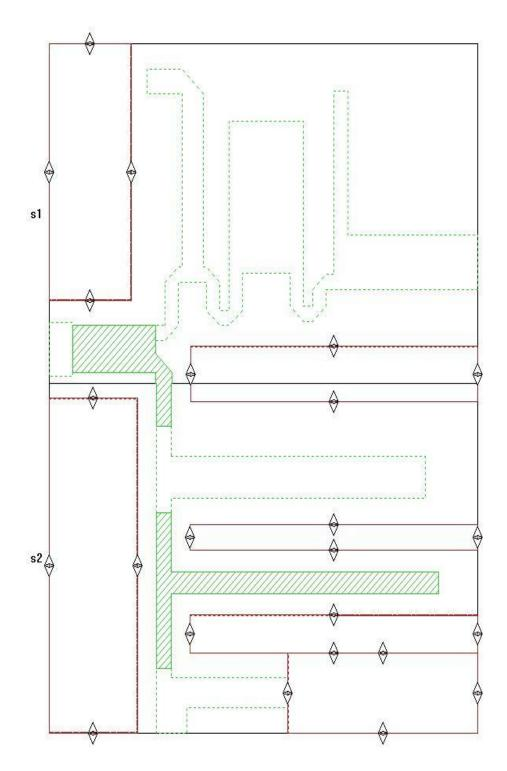
Figure 4.16 (a) ) top section of 6 GHz diplexer  $% \left( {{{\bf{F}}_{{\rm{c}}}} \right)$
