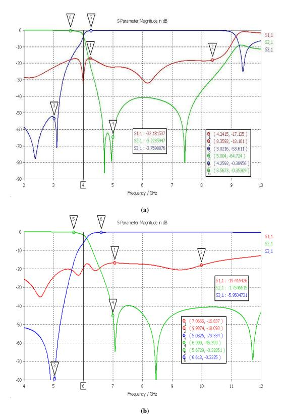
Figure 4. 20 (a) response of 4 GHz diplexer (b) response of 6 GHz diplexer
