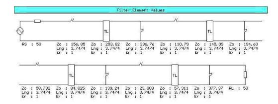
Figure 3. 30. HP channel after extraction
