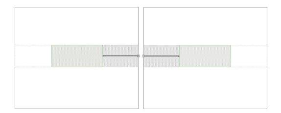
Figure 4. 4 Simulation layout for broadside coupled line replacing capacitors.
