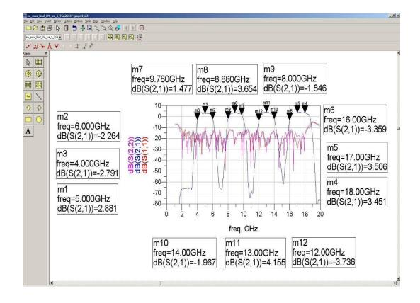
Figure 5.43 Response when odd channels are OFF, even channels are ON
