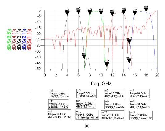
Figure 5.26 Measurement Results and layout for multiplexer for even channels (a) Measurement results
