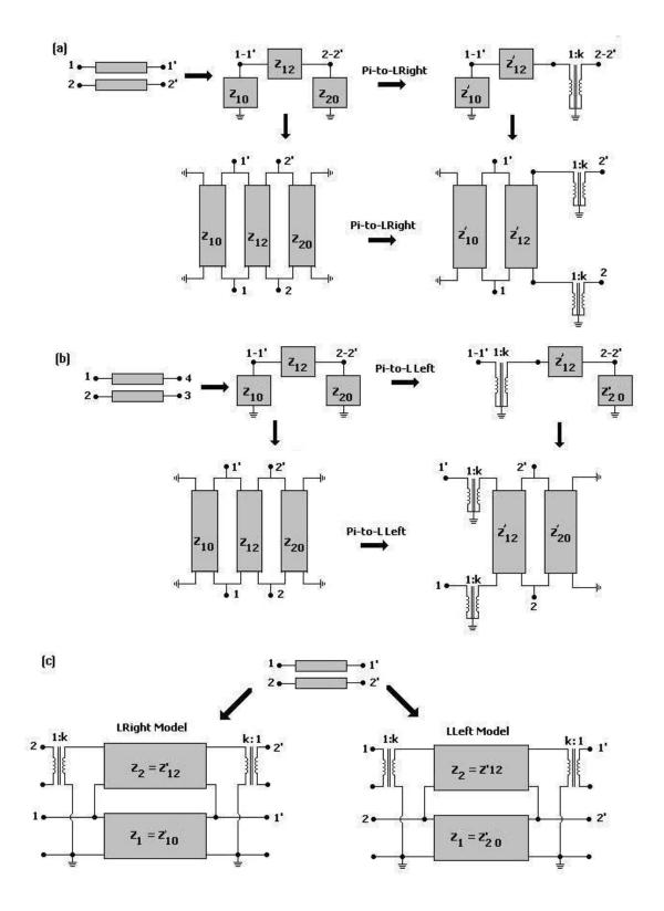
Figure 3. 7 Pi -to- Lright and Pi -to- Lleft transformations applies to a parallel coupled line
