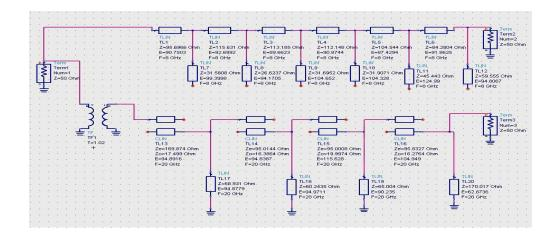
Figure 3. 28 Diplexer after optimization in ADS
