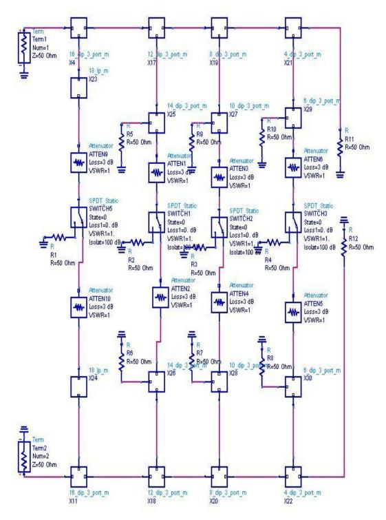
Figure 5. 34 Even channel SW\_MUX with attenuators
