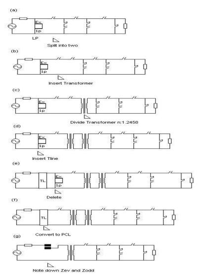
Figure 4. 11 Design steps for HP channel of 6 GHz diplexer
