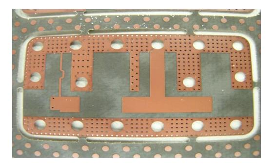
(a) Figure 5.8 Manufactured 2 GHz HP filter (a) PCB front side
