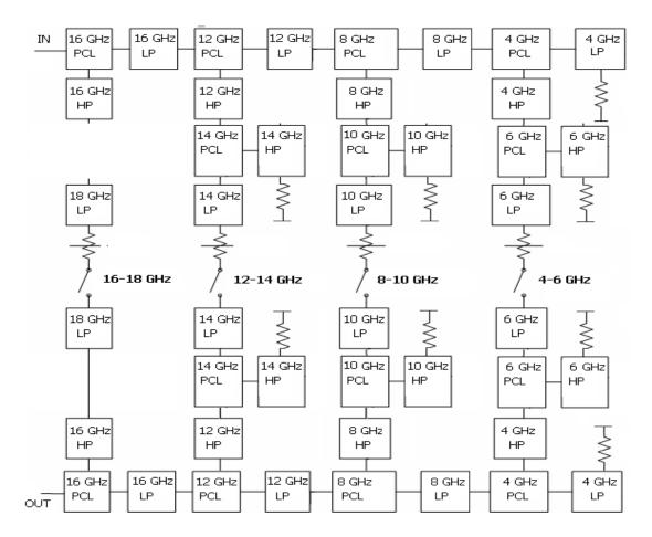
Figure 2. 19 Even Half of SW\_MUX with diplexers in place of extra attenuators.
