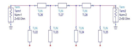
Figure 5.8 18 GHz LP filter
