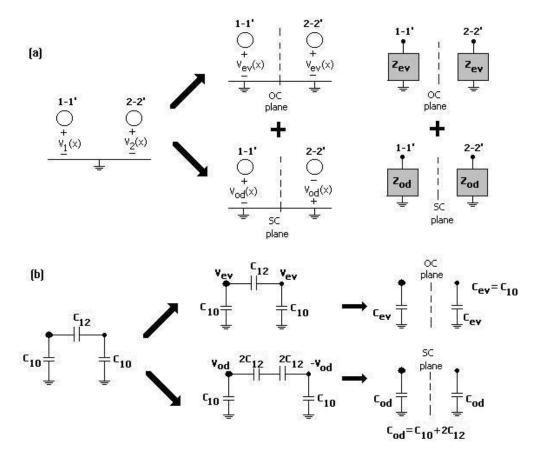
Figure 3. 2 Even-odd mode decomposition of a symmetric parallel coupled line pair
