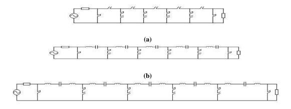
(c) Figure 4. 1 Design steps for the 14 GHz HPF in FILPRO
