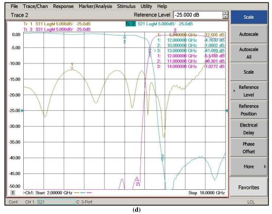
Figure 4. 18 (continued) (c) response of 10 GHz diplexer (d) response of 12 GHz diplexer
