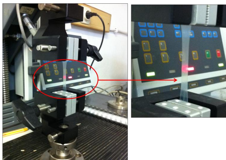
Figure 2.5. The mechanical tester used to study the tensile behavior of and P(L-D,L)LA and P(L-D,L)LA:PLGA (60:40) films.
