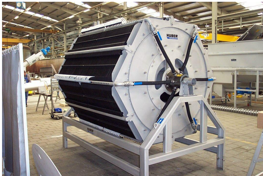
Figure 3.2 Vacuum Rotation Membrane Unit (Komesli et al., 2007)
