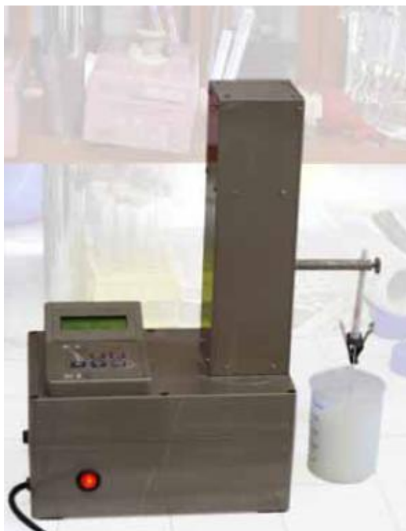
Figure 10: Dip coating apparatus
