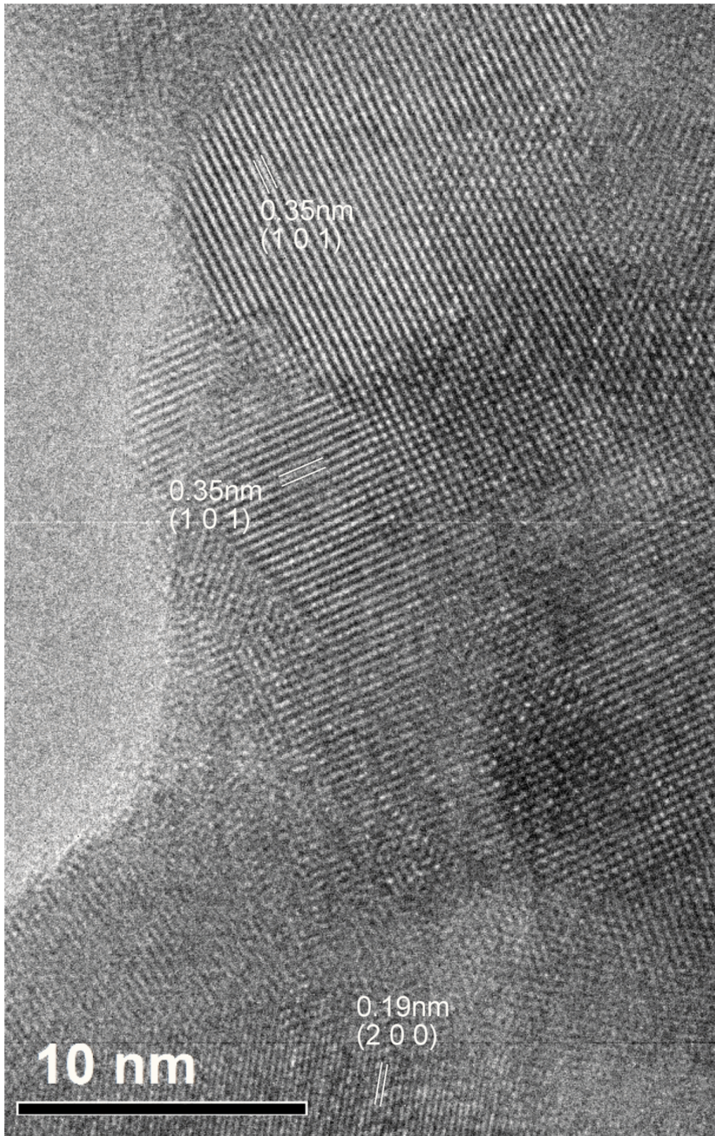
Figure 42: HRTEM photo of the catalyst containing 20%Pr and calcined at 600°C
