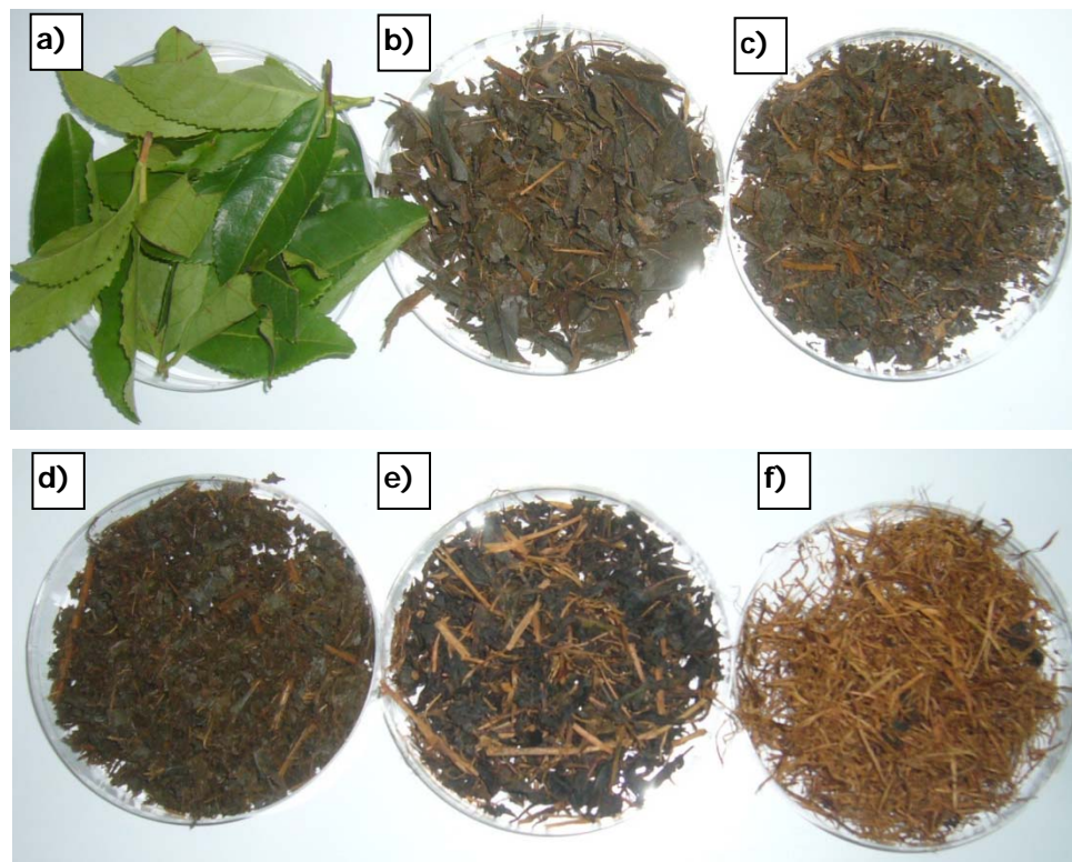
Figure 2. 5 Tea samples delivered freshly from production area (a)harvested fresh tea leaves, b) after bruising, c) before fermentation, d) after fermentation, e) after drying, f) remaining waste).
