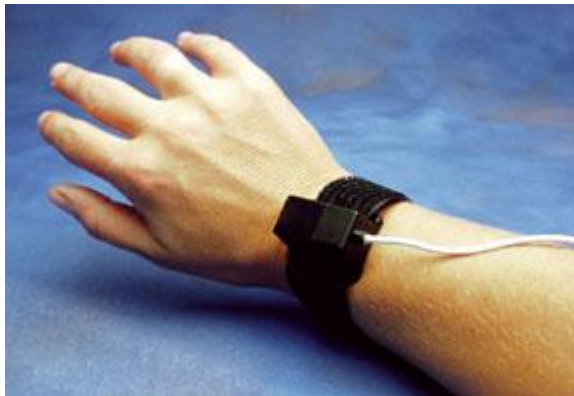
Figure 10.a) A tri-axial accelerometer mounted on wrist and
