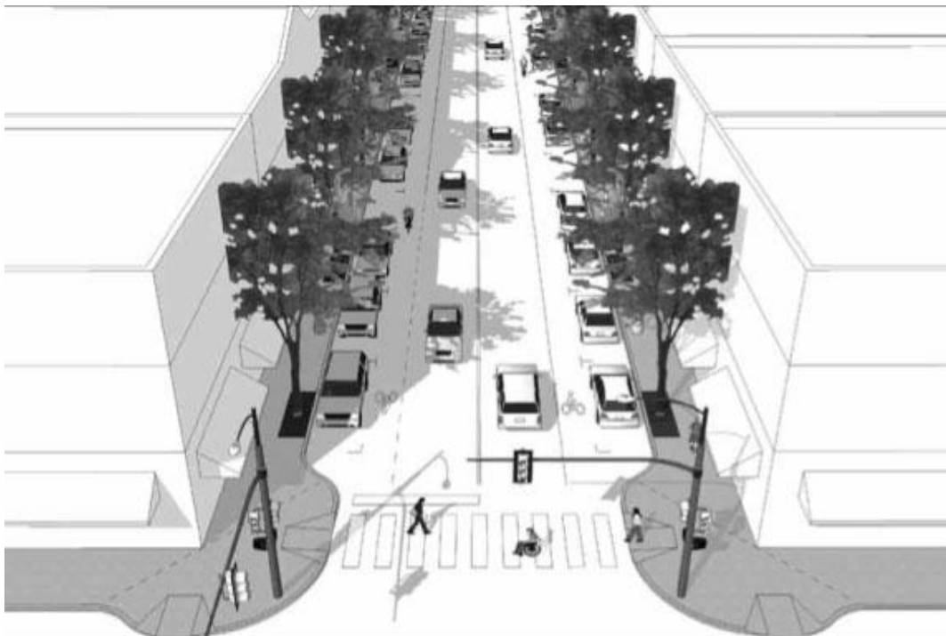
Figure 6-4: Traffic calming elements such as curb extensions, textured crosswalks, bollards, and plantings that encourage pedestrians to walk around within slowing vehicular traffic, and disabled people to increase their ease of movement and accessibility. ( http://www.streetsblog.org/2010/04/08/making-streets-for-walking-dan-burden-on-reforming-design-standards/ )
