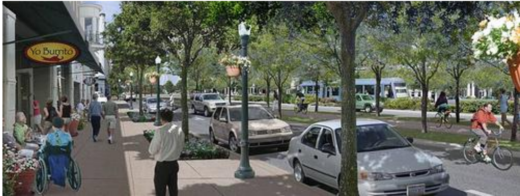
Figure 6-3: Defined walking zone, furnishing zone and frontage zone providing ease of movement ( http://switchboard.nrdc.org/blogs/kbenfield/made_in_the_shade_trees_and_wa.html )
