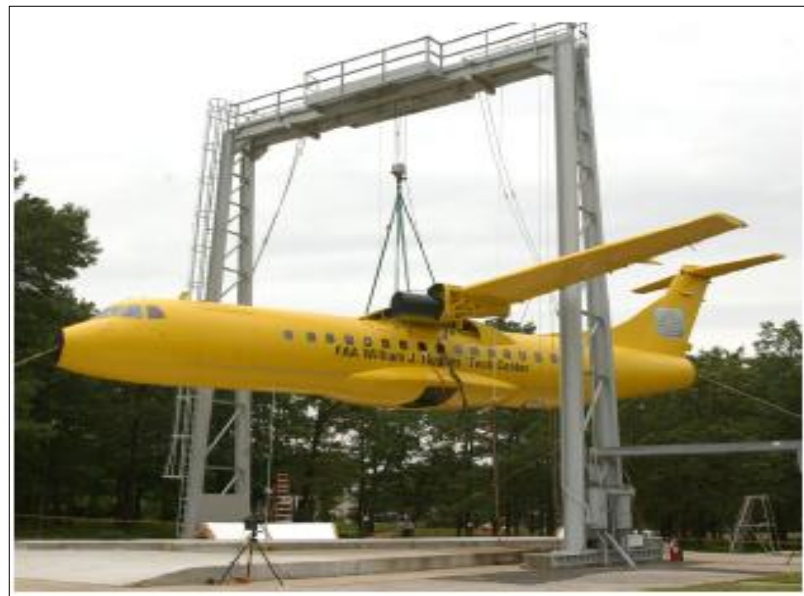
Figure 2-13 Pre-test photograph of the ATR42 aircraft at 14 feet [10]
