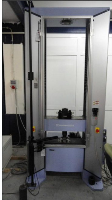
Figure 2-32 Quasi-static compression test device
