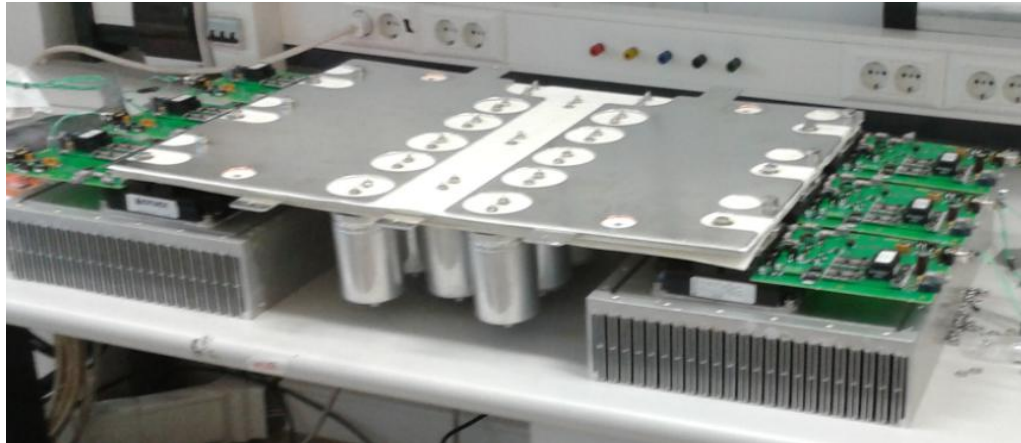
Figure 3.6 Bus bar and Capacitors of Low Pass Filter
