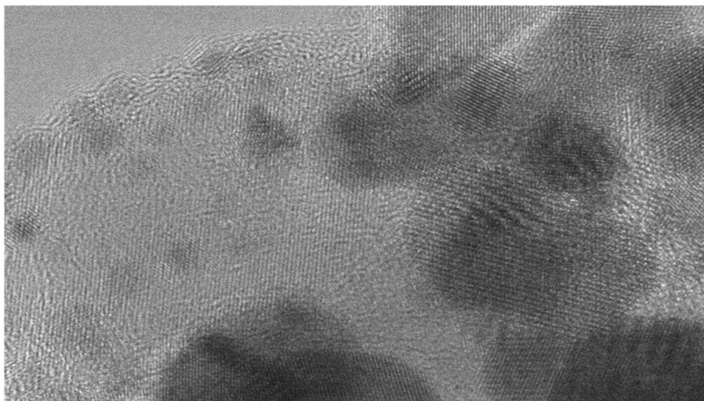
Fig. 1. XRD patterns of the TiO 2 films coated on the glass beads (a)TiO 2 films with Pt incorporated in the sol prior to calcinations, calcined at three stages; (b) The films are further coated with Pt via the incipient wetness technique and (c) the corresponding HR-TEM image containing Pt incorporated via incipient wetness technique.
