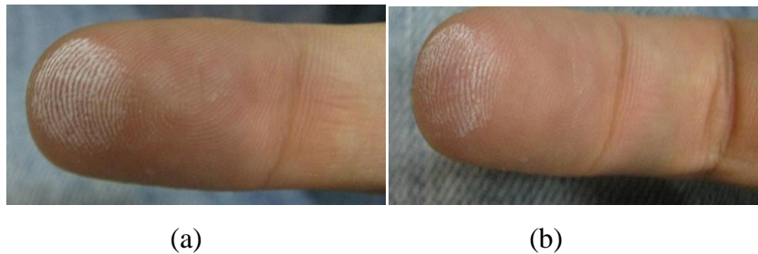
Figure 4.28 Finger testing of a) S9 sample a) without and b) with white cement binder.
