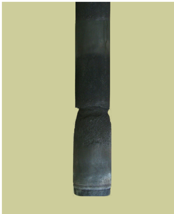
Figure 4.24: Photograph of the graphite rod after electrolysis in the preliminary large scale test.
