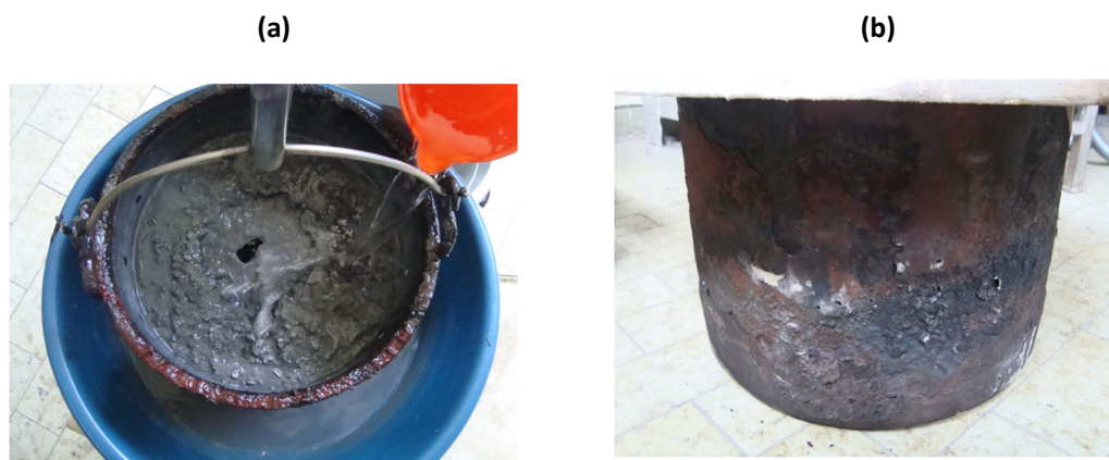
Figure 4.23: Photographs of the (a) cathode tray and (b) the vessel after 18 hours of electrolysis.
