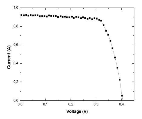
Figure 4.14 I-V curve of the solar cell at the doping concentration ratio of 5000 ppm with 72 cm<sup>2</sup> area and 4.7% efficiency with  $V_{oc}$ :0.406 V,  $I_{sc}$ :0.922 A, FF:89.46%.
