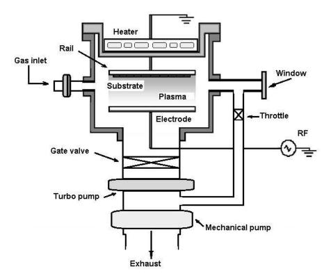
Figure 3.1 The schematic representation of a PECVD deposition system
