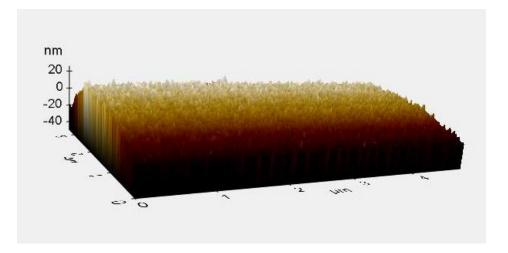
Figure 4.8 AFM surface measurement result for T<sub>subs</sub>: 225 °C sample.
