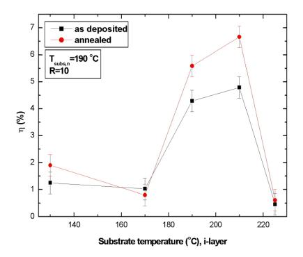
Figure 4.38 Effect of annealing on the efficiency of the deposited structures according to intrinsic layer deposition temperature, at 190 °C n layer deposition temperature.
