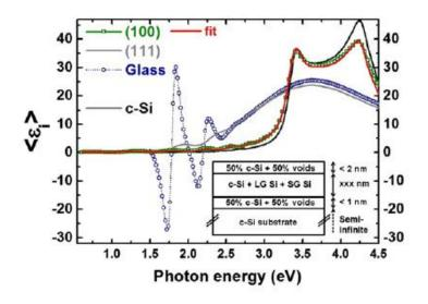
Figure 2.18  $\epsilon_i$  variation of silicon thin films with photon energy, deposited on Corning glass, (100) c-Si and (111) c-Si substrates [41].
