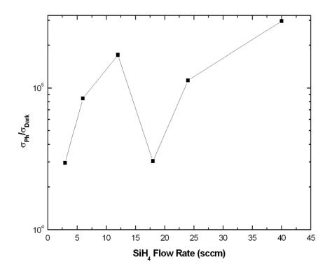
Figure 4.4 Variation of photo to dark conductivity ratio with gas flow rate.
