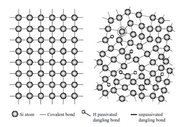
Figure 2.1 Schematic representation of the atomic structures for crystal silicon (a),and for hydrogenated amorphous silicon (b) [5].
