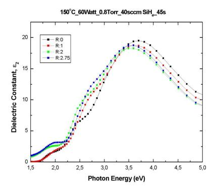
Figure 4.44 Dielectric constant variation of the films with respect to  $[H_2]/[SiH_4]$  ratio, deposited at 150 °C, 60 Watt.
