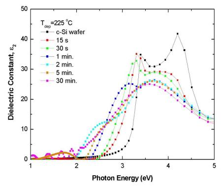
Figure 4.20 Imaginary part of the dielectric constant for the films with different deposition times.
