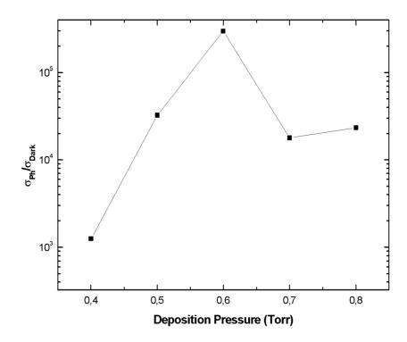
Figure 4.2 Variation of photo to dark conductivity ratio with deposition pressure.
