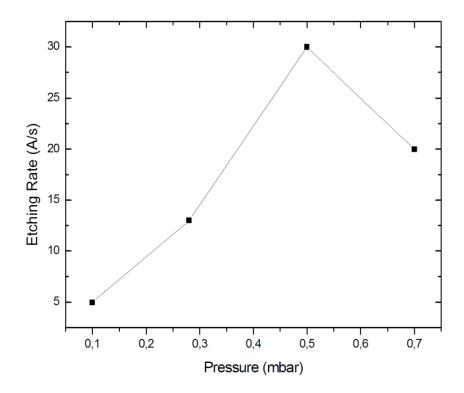
Figure 4.10 a-Si:H etching rate variation with respect to gas pressure.
