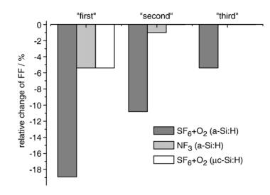
Figure 2.7 Change in the fill factor for a-Si:H and µc-Si:H solar cells relatevly, prepared after in situ cleaning procedure. "First", "second", and "third" cell denote the deposition sequence after in situ dry chamber cleaning [20].
