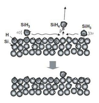
Figure 2.13 Schematic sketch of surface growth process for a-Si:H [35].
