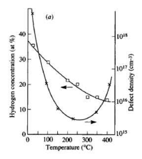
Figure 2.10 Dependence of material properties on substrate temperature [6].
