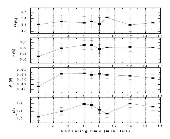
Figure 4.41 Measured  $I_{sc}$ ,  $V_{oc}$ , FF and efficiency variation of i:150 °C, n:225 °C substrate temperatures c-Si/a-Si:H HJ solar cell as a function of annealing time.
