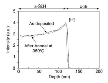
Figure 4.43 Hydrogen SIMS profile on n-type c-Si wafers passivated with a-Si:H before and after annealing at 350 °C [105].
