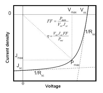
Figure 3.10 Typical J-V curve and the characterization parameters [91].
