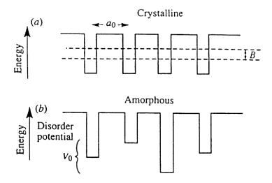
Figure 2.4 Anderson's model representations for both the crystalline and amorphous structures [6].
