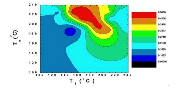
Figure 4.32 3D contour  $V_{oc}$  of solar cells as a function of i- and n- layer deposition temperatures.
