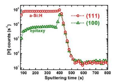
Figure 2.19 SIMS results of hydrogen in silicon thin films co-deposited at 175 °C on (111) and (100) c-Si substrates [41].
