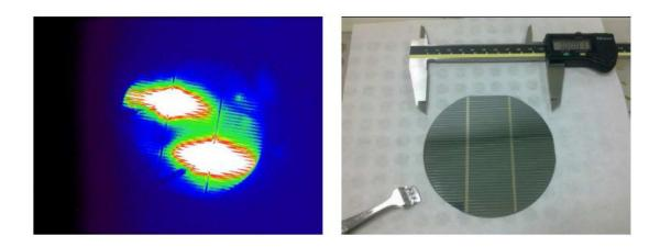
Figure 4.24 Electroluminescence image (left) and picture (right) of the solar cell deposited at at 225 °C substrate temperature; 0.6 Torr pressure; 12 mW/cm<sup>2</sup> and 5000 ppm doping ratio.
