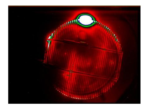
Figure 4.26 Electroluminescence image of the solar cell after optimization studies.
