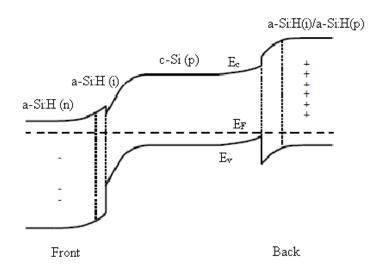
Figure 2.26 Band diagram sketch of a double side SHJ solar cell on (p) c-Si wafer [40].
