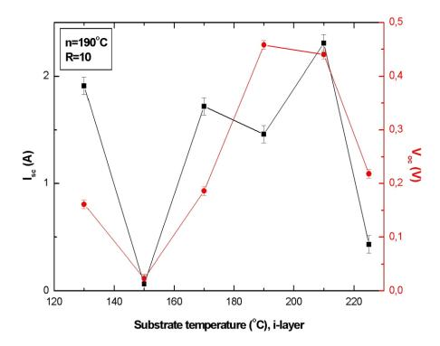
Figure 4.31  $I_{sc}$  and  $V_{oc}$  variation of the deposited structures according to intrinsic layer deposition temperature.
