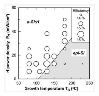
Figure 2.21 Solar cell efficiency distributions obtained at different growth temperatures and rf power densities [44].
