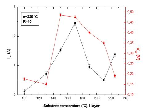
Figure 4.29  $I_{sc}$  and  $V_{oc}$  variation of the deposited structures according to intrinsic layer deposition temperature.
