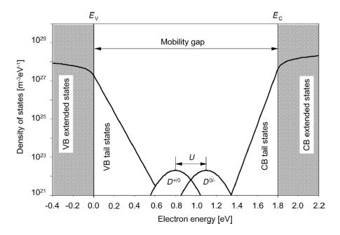
Figure 2.3 Density of states distribution for both c-Si and a-Si:H [5]
