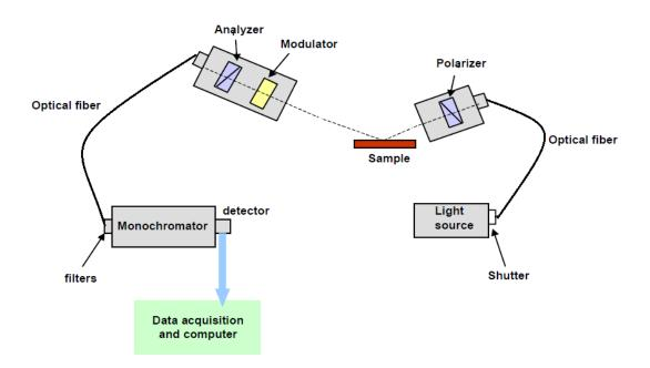
Figure 3.6 Schematic of the Spectroscopic Ellipsometer measurement system [69]
