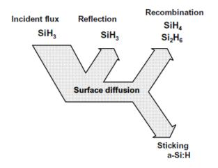
Figure 2.12 Surface reaction processes for on-coming SiH<sub>3</sub> radicals [35].
