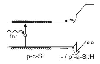
Figure 2.27 Band diagram sketch of a (p) c-Si wafer/ (i) a-Si:H/( $p^+$ ) a-Si:H heterostructure [2].
