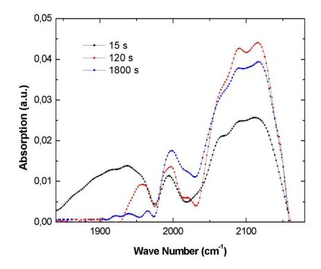
Figure 4.23 Variation of FTIR spectrum of the films at different deposition times.
