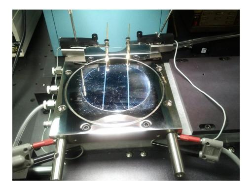
Figure 3.9 Picture of the J-V measurement system
