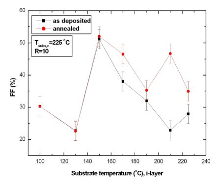
Figure 4.36 Effect of annealing on the FF of the deposited structures according to intrinsic layer deposition temperature, at 225 °C n layer deposition temperature.
