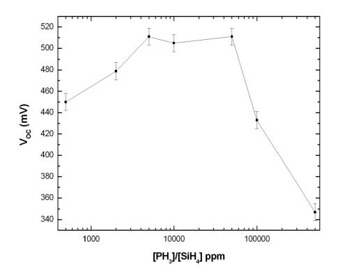
Figure 4.13 Open-circuit voltage variation as a function of the gas phase doping concentration
