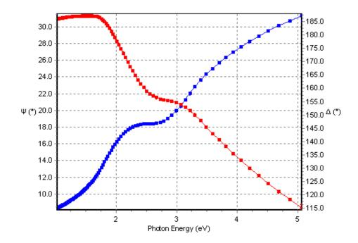
Figure 4.19 Matching of SE measurements (symbols) with model fitting (solid lines), for 120 s deposited sample.
