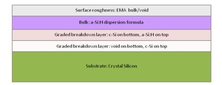
Figure 4.18 Multi layer model for 120 s deposited sample, representing the structure of the material as accurately as possible.
