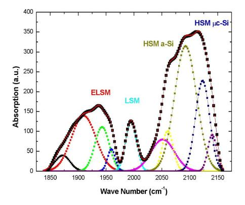
Figure 4.22 Hydride stretching modes in the FTIR spectra for 15 s film.
