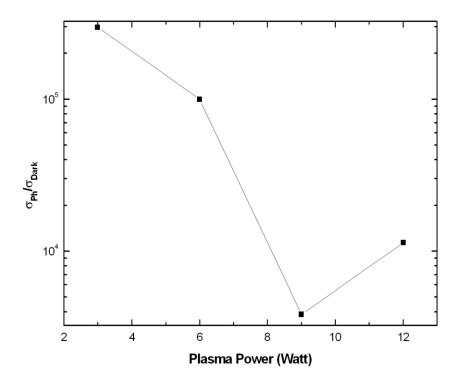
Figure 4.3 Variation of photo to dark conductivity ratio with plasma power.
