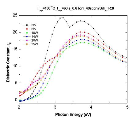
Figure 4.27 Dielectric constant variation of the films with respect to RF power.
