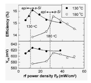
Figure 2.20 Efficiency and  $V_{\rm oc}$  variations of the a-Si:H/c-Si solar cell, plotted as a function of rf power density  $P_{\rm rf}.$
