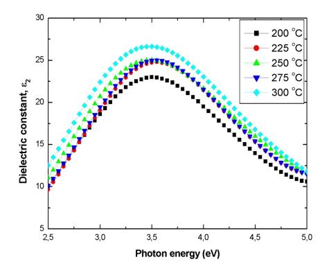
Figure 4.5 Dielectric function spectra for the a-Si:H films deposited on glass substrate at different substrate temperatures.
