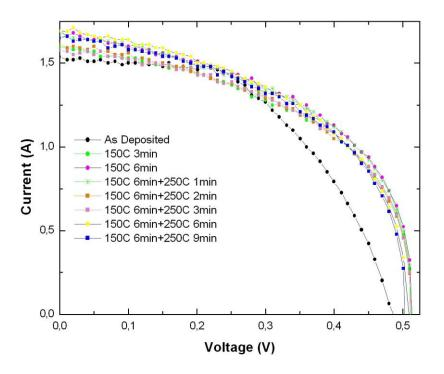
Figure 4.40 Current-Voltage improvement graph with annealing of the film deposited at n=225 °C, i:150 °C, R:10.
