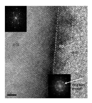
Figure 4.16 HRTEM micrograph of c-Si/(i) a-Si:H interface.
