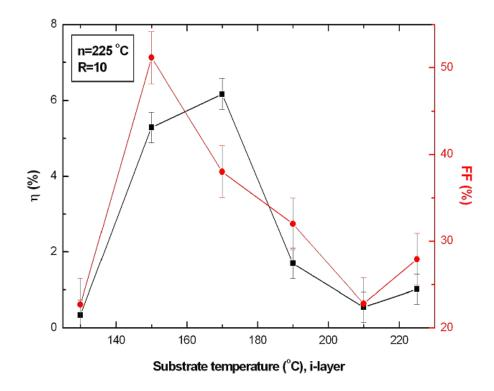
Figure 4.28 Efficiency and FF variation of the deposited structures according to intrinsic layer deposition temperature.
