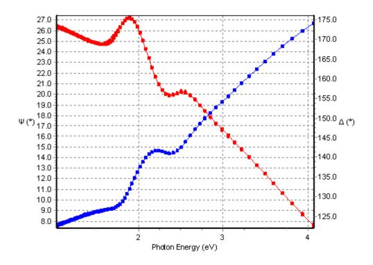
Figure 4.47 SE fit with  $\chi^2$  0.063, for the intrinsic a-Si:H thin film deposited at 150 °C substrate temperature, R:1, 80 Watt, 0.8 Torr, 45 seconds on (p) c-Si wafer.
