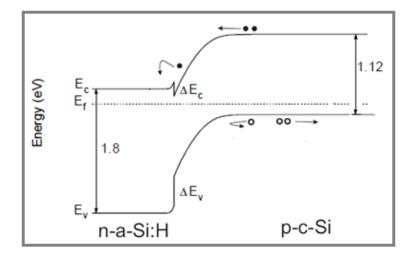
Figure 2.24 Energy bandgap diagram for (n) a-Si:H/(p) c-Si heterojunction interface [2].
