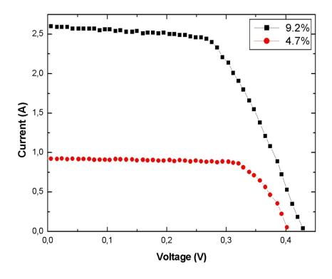
Figure 4.25 I-V curve of the solar cell after the optimization studies under AM 1.5G solar simulator light.
