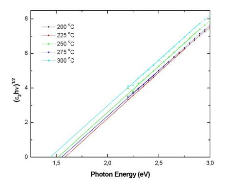
Figure 4.6 Analysis of optical bandgap (Cody gap) using the  $\varepsilon_2$  spectra.
