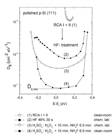
Figure 3.4 Interface state density curves for p-type Si(111) surfaces obtained after different cleaning procedures [61].
