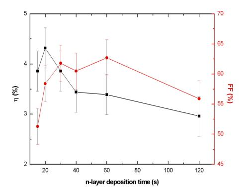
Figure 4.48 Efficiency and FF variation of the device, deposited at 225 °C, with respect to n layer deposition time.
