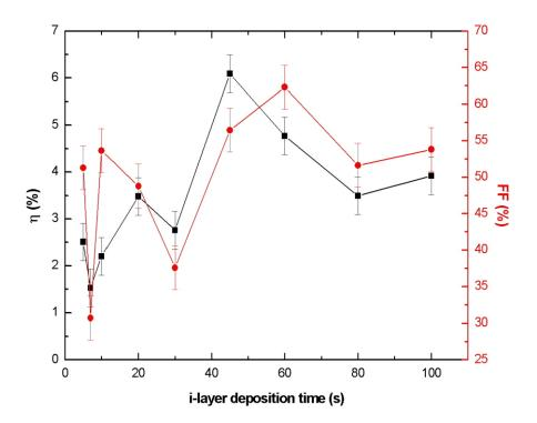
Figure 4.50 Efficieny and FF variation of the device, deposited at 225 °C, with respect to i layer deposition time.
