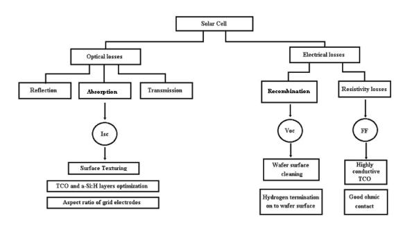
Figure 2. 16 Losses sources in heterojunction silicon solar cells.
