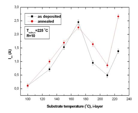
Figure 4.37 Effect of annealing on the  $I_{sc}$  of the deposited structures according to intrinsic layer deposition temperature, at 225 °C n layer deposition temperature.
