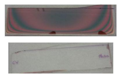
Figure 4.11 Glass substrate before and after NF<sub>3</sub> etcing in PECVD.
