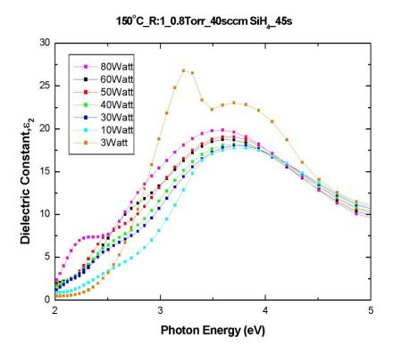
Figure 4.45 Dielectric constant variation of the films with respect to RF power, deposited at 150 °C,  $[H_2]/[SiH_4]=1$ .
