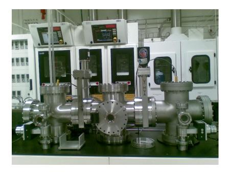
Figure 3.2: TUBITAK UME UHV-PECVD System
