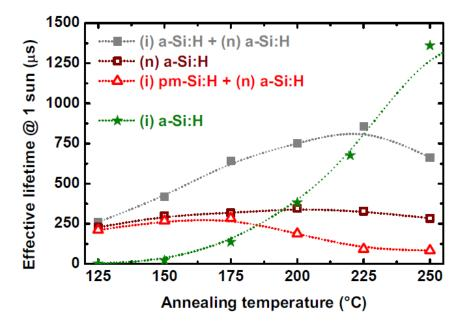
Figure 2.23 Effective lifetime at 1 sun on (n) c-Si with different structures.
