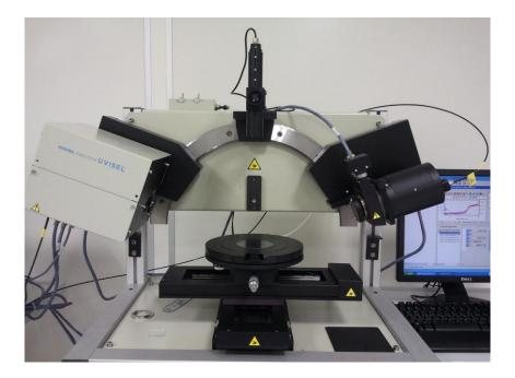
Figure 3.5 TUBITAK UME Jovin Yvon UVISEL Spectroscopic Ellipsometer measurement system
