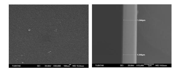
Figure 4.7 SEM surface and cross-section images of a T<sub>subs</sub>: 225 °C sample.
