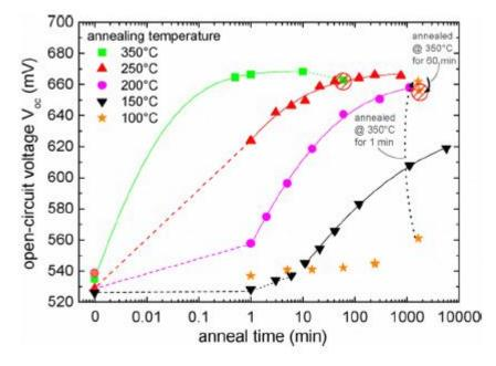
Figure 2.22 The open-circuit voltage variation with respect to annealing time at different annealing temperatures [45].
