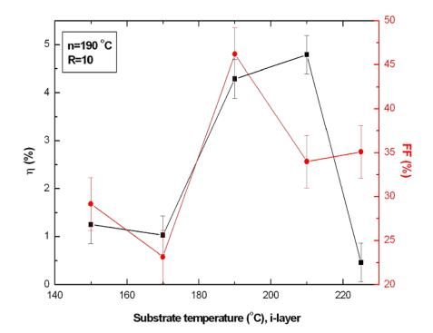
Figure 4.30 Efficiency and FF variation of the deposited structures according to intrinsic layer deposition temperature.
