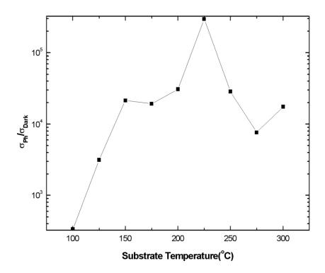
Figure 4.1 Variation of photo to dark conductivity ratio with substrate temperature.
