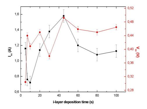
Figure 4.51  $I_{sc}$  and  $V_{oc}$  variation of the device, deposited at 225 °C, with respect to i layer deposition time.
