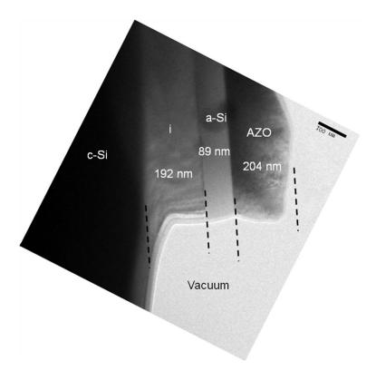
Figure 4.15 HRTEM micrograph of AZO/5 min deposited (n) a-Si:H/5min deposited (i) a-Si:H/c-Si.
