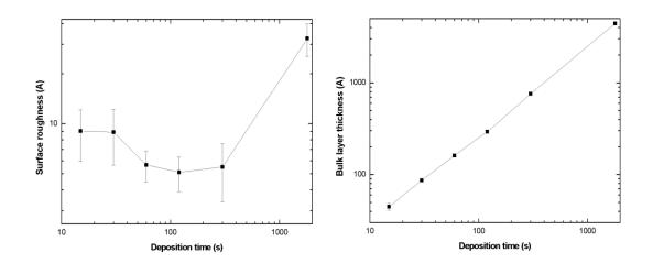
Figure 4.21 Variation of the surface roughness (left) and bulk layer thickness (right) of the a-Si:H films.
