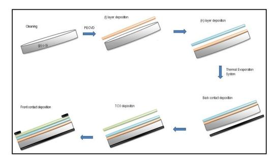
Figure 3.3: Sketch of the preparation sequence of c-Si/a-Si:H cell devices equipped with heterojunction emitters.
