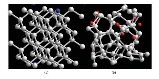
Figure 2.6 3-d computer model representation of c-Si (a), and a-Si (b) with dangling bonds passivated by hydrogen atoms [15].
