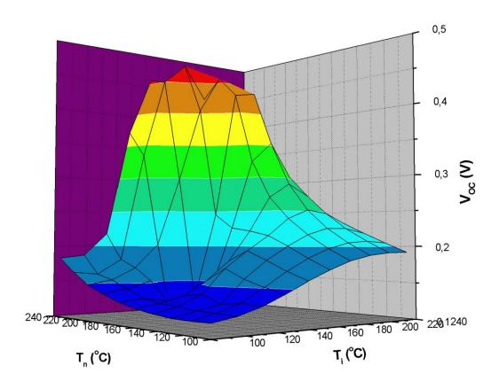
Figure 4.33 3D plot  $V_{\rm oc}$  of solar cells as a function of i- and n- layer deposition temperatures.
