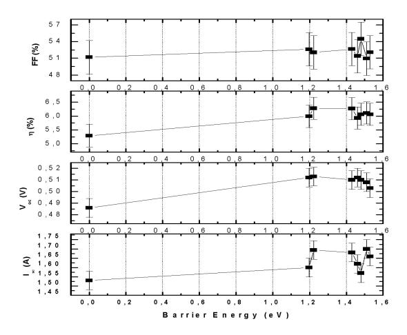
Figure 4.42 Measured I<sub>sc</sub>, V<sub>oc</sub>, FF and efficiency variation of i:150 °C, n:225 °C substrate temperatures c-Si/a-Si:H HJ solar cell as a function of barrier energy.
