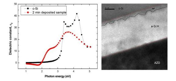
Figure 4.17 Photon Energy versus  $\varepsilon_2$  Graph (left) and HRTEM Image (right) for 120s a-Si:H film.
