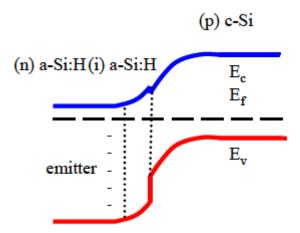
Figure 2.25 Band diagram sketch of a (n) a-Si:H/ (i) a-Si:H/ (p) c-Si heterojunction interface [36].
