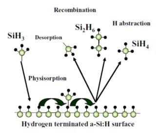
Figure 2.11 Schematic representation of the surface reactions during the growth of a-Si:H where the SiH<sub>3</sub> radicals are the only growth precursors [33-34].
