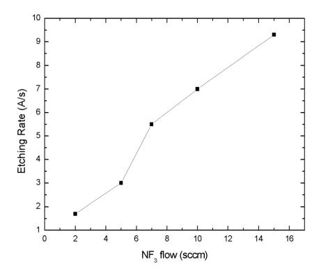
Figure 4.9 a-Si:H etching rate variation with respect to  $NF_3$  flow rate.
