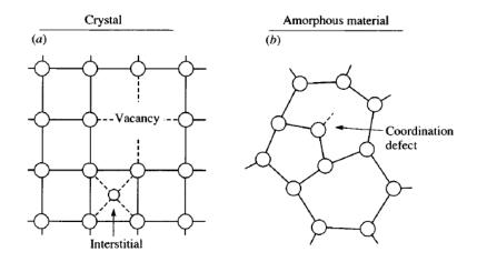
Figure 2.2 An illustration contrasting the different types of simple defects in (a) crystalline and (b) amorphous networks [6].
