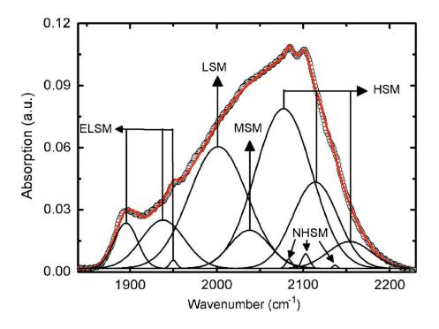
Figure 3.8 Deconvolution gaussian peaks for µc-Si:H films IR spectrum [87].
