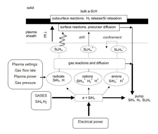
Figure 2.8 Schematic representation of the a-Si:H deposition from SiH<sub>4</sub>/H<sub>2</sub> plasma [27].
