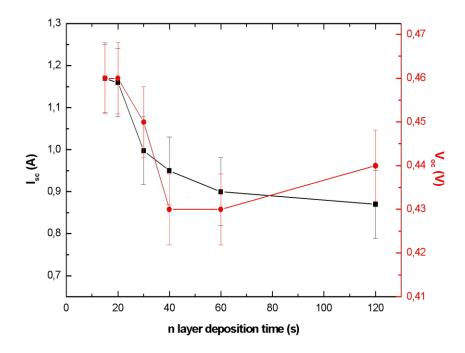
Figure 4.49  $I_{sc}$  and  $V_{oc}$  variation of the device, deposited at 225 °C, with respect to n layer deposition time.
