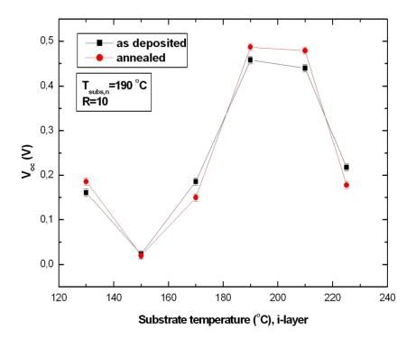
Figure 4.39 Effect of annealing on the  $V_{oc}$  of the deposited structures according to intrinsic layer deposition temperature, at 190 °C n layer deposition temperature.
