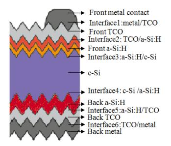
Figure 2. 17 Structure of a double side heterojunction solar cell.
