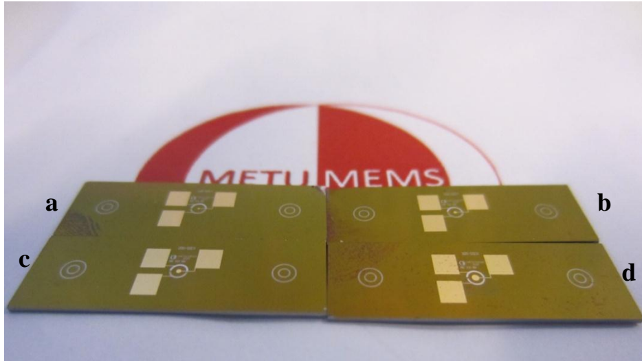
Figure 4.31. A photograph demonstrating fabricated prototypes (a) r = 100 \mu\text{m} , (b) r = 150 \mu\text{m} , (c) r = 200 \mu\text{m} , (d) r = 300 \mu\text{m} .
