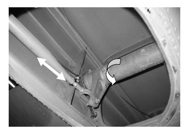
Figure 1-8. Control mechanism of the horizontal stabilizer
