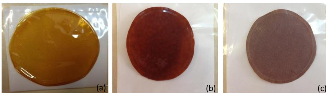
Figure 4.2: In-line annealed (a) Neat PBI membrane, (b) PBI/Zeolite 3A membrane top side, (c) PBI/Zeolite 3A membrane bottom side after solvent evaporation
