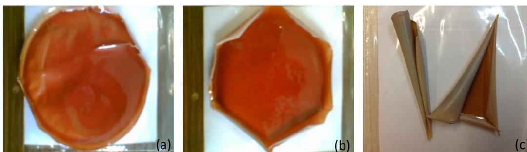
Figure 4.1: In-oven annealed membranes (a) Neat PBI membrane, (b) (c) PBI/Zeolite 3A membranes
