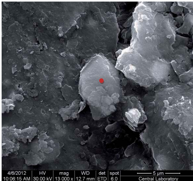
Figure 3.17. (a) The platy and coalesced morphology of illites within sample YBA-19A from Yılanlı Burnu quarry (b) The EDX pattern of YBA-19A presents the illitic composition (high S and Fe contents indicate pyritization)
