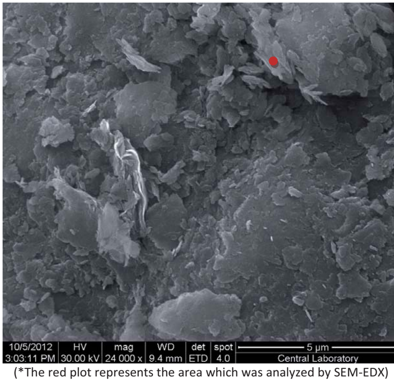
Figure 3.21. (a) The SEM microphotograph displays platy and juxtaposed structure of illites and (b) EDX pattern of OC1(B3) sample indicates the illitic composition of the sample.
