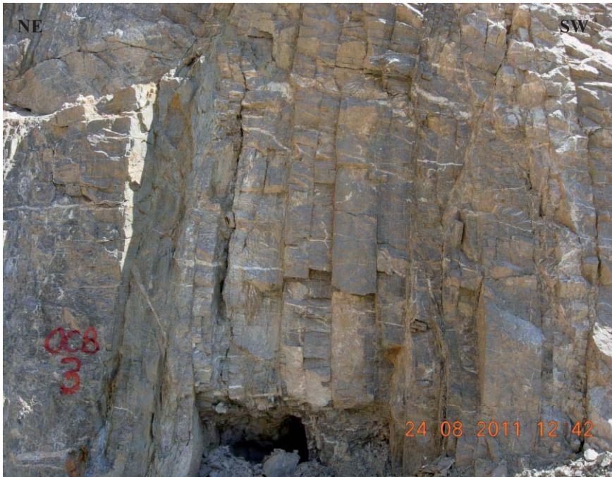
Figure 1.8. Another view of vertically layering Gavurpinari limestone beds along the NE-SW direction.
